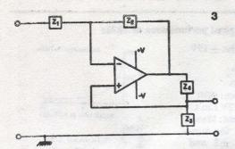
Fig. 3 shows the general form of the circuit, one version of which has been discussed. Other configurations are possible by interchanging  $Z_1$  and  $Z_4$  and/or  $Z_2$  and  $Z_3$ . Note that the output may not then be taken from the op-amp output.
