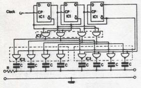
IC1 SN7474 D-type IC2 2 off SN7400 connected as two-input AND gates IC<sub>3</sub> SN7401 quadruple with open collector out- N = number of lowput. R: 1k0 ±1%
