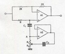
Q of resonant branch is  $\frac{1}{R_1 + R_2} \cdot \sqrt{\frac{C_2 R_1 R_2}{C_1}}$
