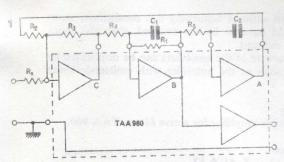
$f_0 = \frac{1}{2\pi \sqrt{C_1 C_2 R_4 R_5}}$ Drive: 400mV pk-pk.
