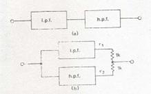
(a) provides the bandpass characteristic shown. Low and highpass filters used are described in cards 4 and 5 with cut-off frequencies 10kHz and 2.35kHz respectively.  $f_1 = 5kHz$ ,  $f_2 = 1.9 \text{kHz}$  and  $f_3 = 13 \text{kHz}.$
