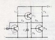
Typical performance  $R_1$  100kΩ,  $R_2$  22kΩ  $R_3$  4.7kΩ,  $R_4$ ,  $R_5$  470kΩ  $C_1$ ,  $C_2$  10 $\mu$ F  $Tr_1$ ,  $Tr_3$  BC125  $Tr_2$  BC126 Supply +1.5V Voltage gain 2100 Output impedance  $3k\Omega$
