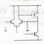
commonplace in the monolithic i.cs mentioned above. As Tr<sub>7</sub> and Tr<sub>8</sub> carry the same current, then provided Tr<sub>6</sub> base current remains small, so also must Tr<sub>3</sub> and Tr<sub>4</sub>.
