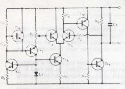
Typical performance  $R_1$ ,  $R_2$ ,  $R_3$  1k $\Omega$  $R_4 12k\Omega$  $R_5$ ,  $R_6$  3.3k $\Omega$ R<sub>7</sub>, R<sub>8</sub>, R<sub>9</sub> 1<sub>κ</sub>Ω  $C_1 100 \mu F$ Tr<sub>1</sub>, Tr<sub>3</sub> 2N1302 Tr<sub>2</sub> 2N1303 Tr4, Tr5, Tr8 B2125 Tr<sub>6</sub> BC126 Tr<sub>7</sub> MJE521 Supply 2V  $R_L 2\Omega$ V<sub>L</sub> 400mV Output res.  $0.01\Omega$ For  $\Delta V_s/R_L \pm 20\%$ ,  $\Delta R_{\rm L}/R_{\rm L} \pm 20\%$  $\Delta V_{\rm L}/V_{\rm L} \approx \pm 0.5\%$
