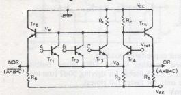
Typical operating data  $R_1 \, 270 \Omega$ ,  $R_2 \, 300 \Omega$   $R_3 \, 1.2 k \Omega \, R_5$ ,  $R_6 \, 1.5 to \, 2 k \Omega$  VCC 0V, Vref -1.15V, VEE -5V Logic 1 output -0.75V Logic 0 output -1.5V Propagation delay 5 to 11ns Max a.c. fan-out 15
