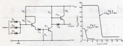
Elimination of the  $V_{\rm BB}$  supply can simplify circuitry in many instances, a popular modified form of the d.t.l. NAND gate using a single supply being shown in Fig. 3. In comparison with Fig. 2, the offset diode  $D_4$  is replaced by  $Tr_2$  and  $R_D$ . This transistor provides amplification that allows a higher level of base drive to be fed to  $Tr_1$ , achieving a higher fan-out capability, and also permits a reduction in the value of  $R_K$  compared with Fig. 2.
