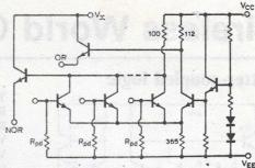
A temperature-compensated regulator package of the form shown left is available as the reference voltage, also frequently on the same chip as the gate structure. This minimizes variation of noise margin with temperature.
