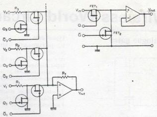
• The arrangement right, a series-shunt chopper, is best suited to voltage sources as neither the op-amp or Tr<sub>2</sub> draws significant current when Tr<sub>1</sub> is on, or when Tr<sub>1</sub> is off. The current from the source is negligible. Hence the input signal is gated to the op-amp with almost zero attenuation.
