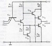
In the basic, or standard t.t.l. NAND gate (card 3), the resistance values affect performance. Resistor R1 influences the rate of voltage at Tr2 base and hence turn-on time. Gate dissipation, when the output is in the 0-state is affected by the value of R2. Stored base charge in Tr4 is removed via R3 when the output state changes from logical 0 to 1. Turn-off time of the gate when feeding a capacitative load is influenced by the value of R4 which provides short-circuit protection.
