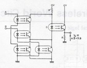
obtained using photo-diodes and lower frequencies with greater current handling capacity with photo-darlingtons (cross ref. 2).
