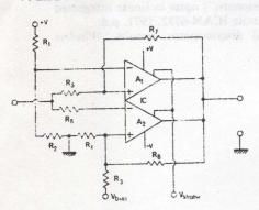
Typical performance Supplies +12V, -6V  $V_{\text{strobe}} = +5V; V_{\text{bias}} - 12V$ R<sub>1</sub>, R<sub>3</sub>: 5.6kΩ R2, R4, R5, R6: 4700 R<sub>7</sub>, R<sub>8</sub>: 22kΩ 1-U = 953mV; 1'L 886mV (i.e. Vou hysteresis = 67mV) V-U -- 946mV; V-L -879mV (i.e. Vol hysteresis 67mV)
