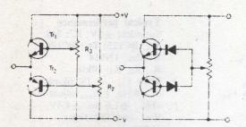
• Diodes could be placed in series with the emitters of the transistors. This still provides base-emitter breakdown protection but the diodes then carry the larger emitter currents producing larger diode p.ds.
