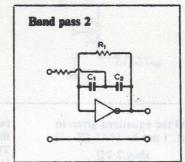
Q-values occur because of the low gain of the amplifier. The centre frequency lay within the tolerance range of the passive components in the samples tested. At the centre frequency, the output is anti-phase to the input. This leads to a simple means of obtaining a notch-characteristic as indicated over. The high values of resistors that can be used make it easy to obtain a very low-frequency band-pass characteristic, while
