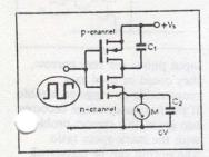
Typical performance IC CD4007AE Supply +10V  $C_1 0.1\mu F$  Meter  $500\mu A$ ,  $200\Omega$  Input Logic level pulse train 0 to 300Hz  $C_2 100\mu F$  I  $fC_1V_8$
