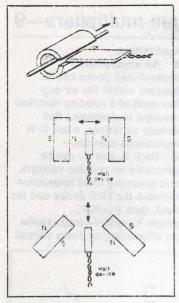
Typical dimensions for transverse devices for insertion in thin gaps 0.006in and for axial probes 0.063in in diameter. A recent development<sup>1</sup>, is a Hall-effect magnetic field detector for translating
