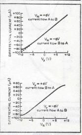
V<sub>y</sub> is zero demands trimming of resistor R6 and R2 to allow for the 1.2V potential at the emitters of Tr2, Tr3. Linearity of Idiff is shown in accompanying graphs. Note, that if  $V_x = +8V$ , this is equivalent to eight units of
