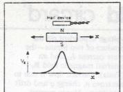
between the device and a stationary magnetic field. Displacement laterally between the magnets will produce an output voltage when the device is moved from the mid-position. An alternative arrangement will provide a linear output proportional to the displacement direction shown. In this case the magnetic field strength varies along a central plane.
