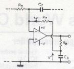
some low audio frequency, but as its Q is not high it could be used to give a degree of bass boost if desired.
