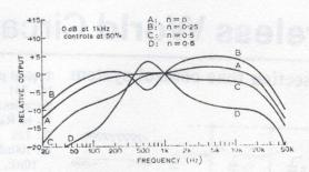
to a virtual notch. These methods must be applied with discretion but as the accompanying graph shows even a single active filter can produce dramatic variations in response (applications could include sound-effects, tone forming in electronic musical instruments).
