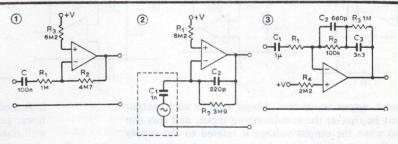
of 10Hz to 100kHz possible with distortion <1% in range 100Hz to 10kHz. Ripple induced hum may be minimized by centre tapping  $R_3$  and decoupling to ground.
