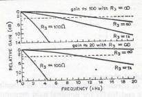
sum of the parallel admittances which determines the gainfrequency characteristic of the amplifier, and either a gain of 20 for a single amplifier, or ten separate gains of 2 can be achieved from the mixer. Thus an overall unity-gain mixer is a not-unreasonable circuit. Although it appears to waste bandwidth at first sight, it allows in practice, with ten inputs, a bandwidth approaching 100kHz.
