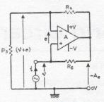
The output impedance at the load terminals is  $Z_0 = Z_p//R_5$ where  $Z_p = v/i$ . For simplicity, let  $R_3 = R_4 = R_5 = R_6 = R$ , then -Ae = 2(V + e)/R. Hence e = -2V/(A + 2) and i = 1(V+Ae)/R = v - [A.2V/(A+2)]. Thus  $Z_p = V/i = (A+2)R/(2-A)$  and  $Z_0 = Z_p/R = R(A+2)/4$ . Therefore, as  $A \to \infty$  $Z_0 \rightarrow \infty$  and a constant current may be fed to R<sub>L</sub>. For an operational amplifier of the 741 type,  $A = -jA_0f_0/f$
