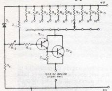
Typical performance Supply: +12V Tr<sub>1</sub>: 2N3702 Tr<sub>2</sub>: BFY50 D<sub>1</sub>: HS7062
