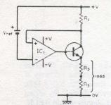
Typical data Supply: ±15V IC1: 741; Tr1: BFR41  $R_1: 1k\Omega \pm 5\% R_2: 680\Omega \pm 5\%$  $R_3: 100\Omega + 0.05\%$ Maximum current: 8mA. Note: Careful layout required to avoid r.f.
