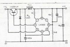
• Output current can be increased by replacing the drive transistor by any high gain combination such as the Darlington pair provided frequency is not too high (charge storage problems) and the increased losses due to saturation are acceptable. At low supply voltages the collector of the first transistor may be returned to the zero line.
