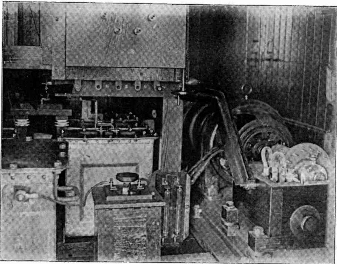
*Transmitting Apparatus on board the S.Y. "Mahroussa."*
