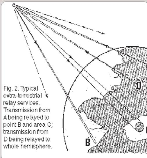
Fig. 2. Typical extra-terrestrial relay services. Transmission from A being relayed to point B and area C; transmission from D being relayed to whole hemisphere.
