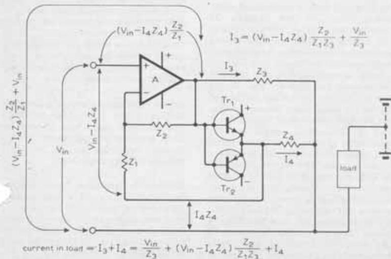
It will help in visualising the operation if the impedances are assumed to be resistors of values  $Z_1=1k\ \text{ohm}$ ;  $Z_2=100k\ \text{ohm}$ ;  $Z_3=100\ \text{ohm}$ ; and  $Z_4=1\ \text{ohm}$ . In the interest of simplicity we have assumed  $Z_4$  to be negligibly small compared to  $Z_1$ , and for the time being we will assume that the voltage output of amplifier A is completely defined by the external impedances.
