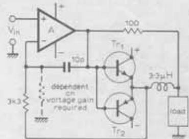
Fig. 3. Simplified diagram showing Class A stage, current dumpers and bridge components.
