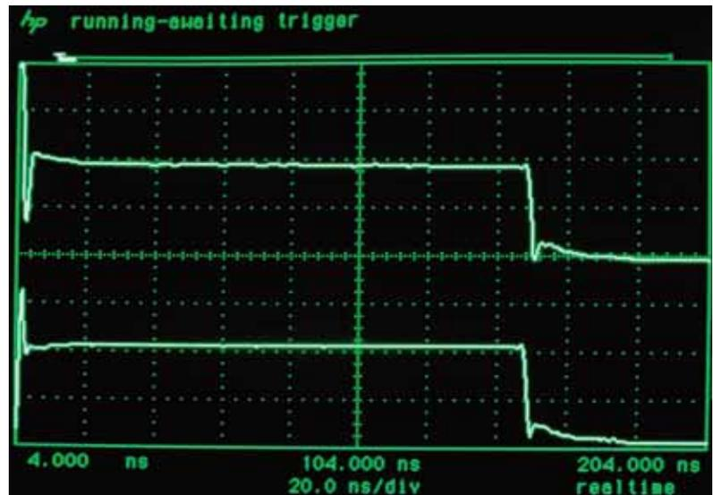
**Figure 1: Bottom Trace:** The bottom trace probe is across the 75Ω terminator used as a trigger. It shows a pulse of the half battery voltage (actually 8V after the 2 x 1MΩ resistors and the probe loading); **Top trace:** Left-hand side of the reed switch. The trace immediately drops from 8V to 4V
