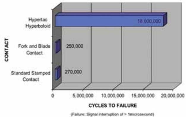
Figure 3: Fretting corrosion characteristic of Hyperboloid contacts
