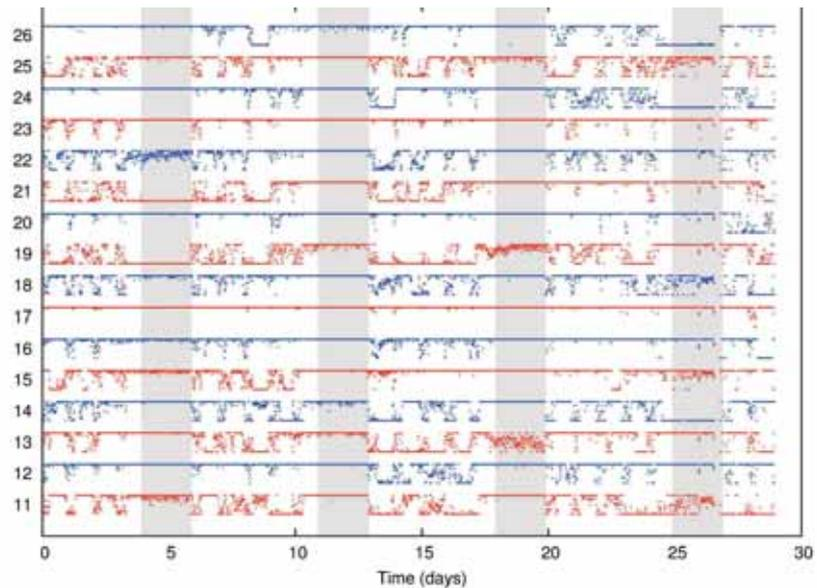
Figure 2: The packet delivery ratio of a wireless link evolves over time
