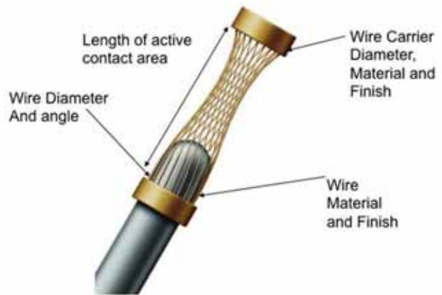
Figure 2: Design parameters of the Hyperboloid socket contact
