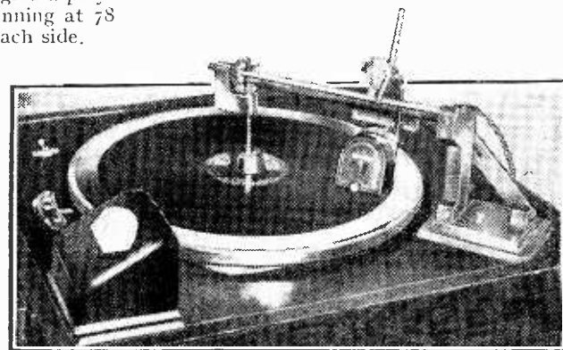
The Permarec Junior home recorder showing also the motor-unit and level indicator.
