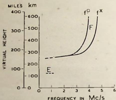
Fig. 13 : Curve showing heights from which the echoes are returned for various frequencies during winter night
