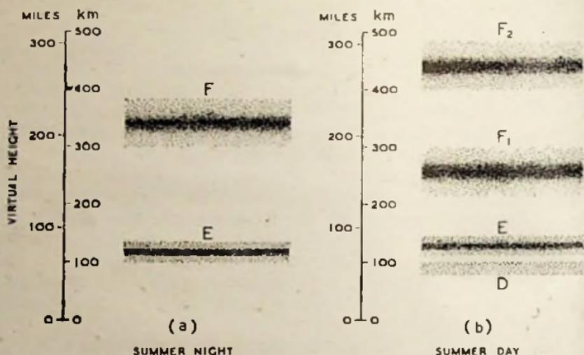
Fig. 9 : How the structure of the ionosphere changes from night to day
