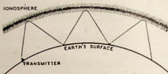
Fig. 6 : Short-wave transmission round the curvature of the earth
