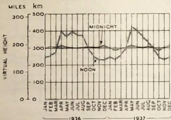
Fig. 19 : Monthly mean of noon and midnight virtual height for  $F$  and  $F_2$  layers
