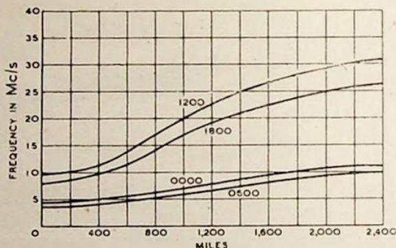
Fig. 25 : Skip distances for various frequencies at different times of day
