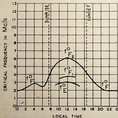
Fig. 15 : (Courtesy U.S. Nat. Monthly graphs of critical frequencies and virtual heights for the Summer and Winter of years of minimum solar activity.
