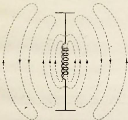
Fig. 1 : Radiation of an electric field from a dipole aerial
