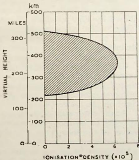
Fig. 8 : Variation of Ionisation density with height—F<sub>2</sub> region
