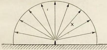
Fig. 3 : Showing direction of travel of some of the "rays" of radio energy
