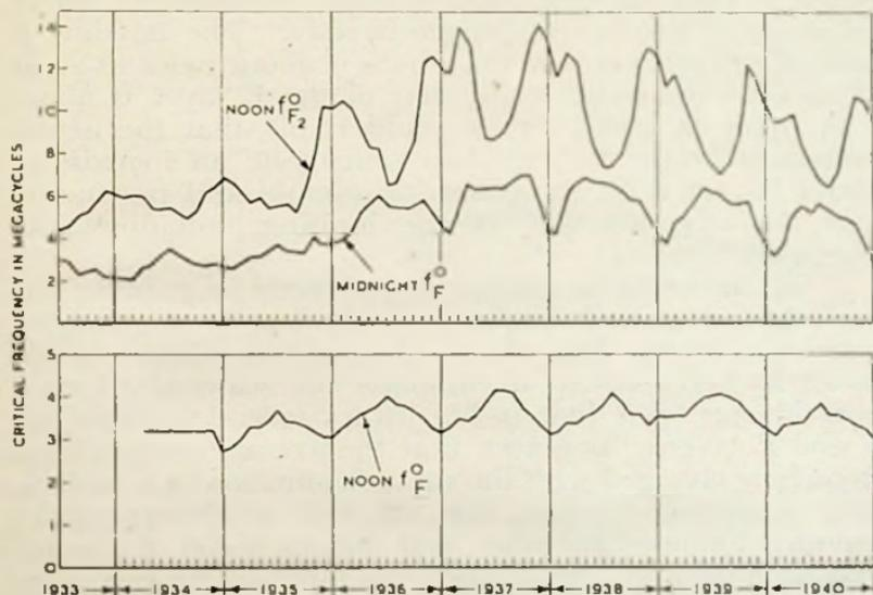
Fig. 17 : Monthly average of noon ( $f_{E}^O$  and  $f_{F_2}^O$ ) and midnight ( $f_F^O$ ) critical frequencies at Washington
