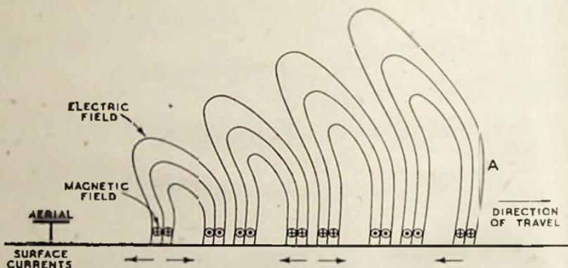
Fig. 2 : Illustrating the elements of the "ground" wave
