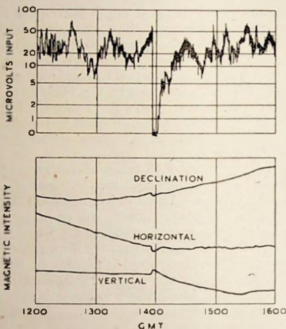
Fig. 26 : Sudden disturbance of the ionosphere on April 6, 1936, as shown by fade-out of 13.525 Mc/s transmission from GLH, Dorchester, observed at Riverhead, New York, and (below) coincidental terrestrial magnetic perturbation recorded at Cheltenham, Maryland, U.S.A. (Reproduced from "Sudden Disturbances of the Ionosphere," by J. H. Dellinger)
