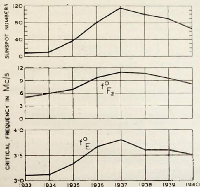
Fig. 18 : Comparison of yearly means of sunspot numbers and of critical frequencies of the E and  $F_2$  layers at noon
