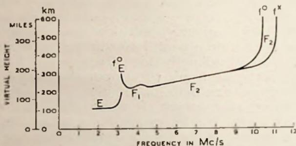
Fig. 12: Curve showing heights from which the echoes are returned for various frequencies during winter day.  $f_o$  relates to the "ordinary" and  $f_x$  to the extraordinary wave, see page 34
