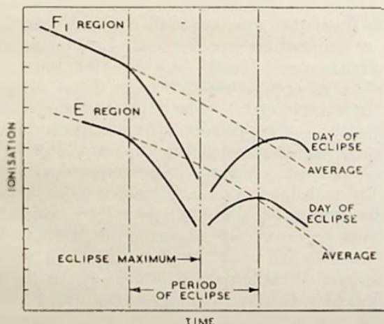
Fig. 7 : Effect of an eclipse of the sun on the ionisation of the  $F_1$  and E layer
