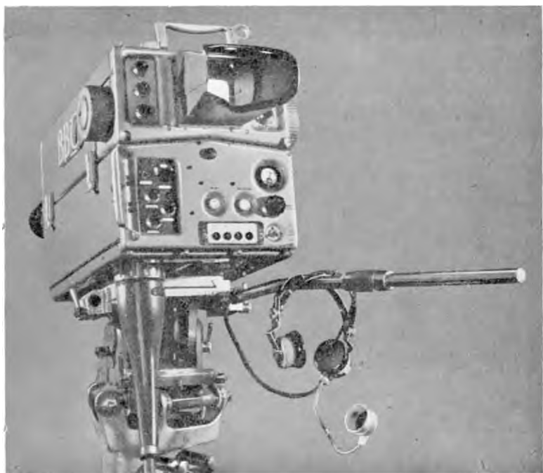
Fig. 119—Rear view of an image orthicon camera showing a portion of the viewfinder screen through the hood
