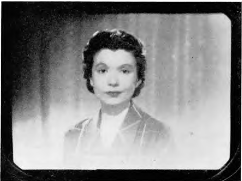
Fig. 30—Effect of spurious signals on image reproduced from an iconoscope
