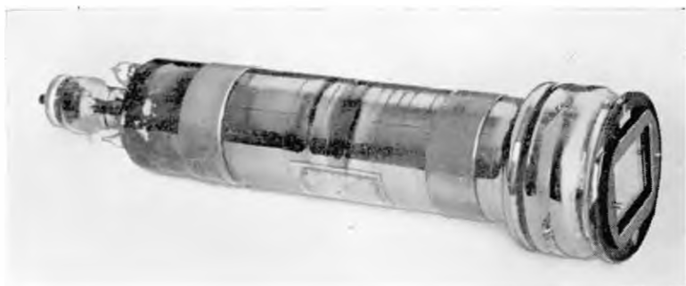
Fig. 44—C.P.S. Emitron camera tube
