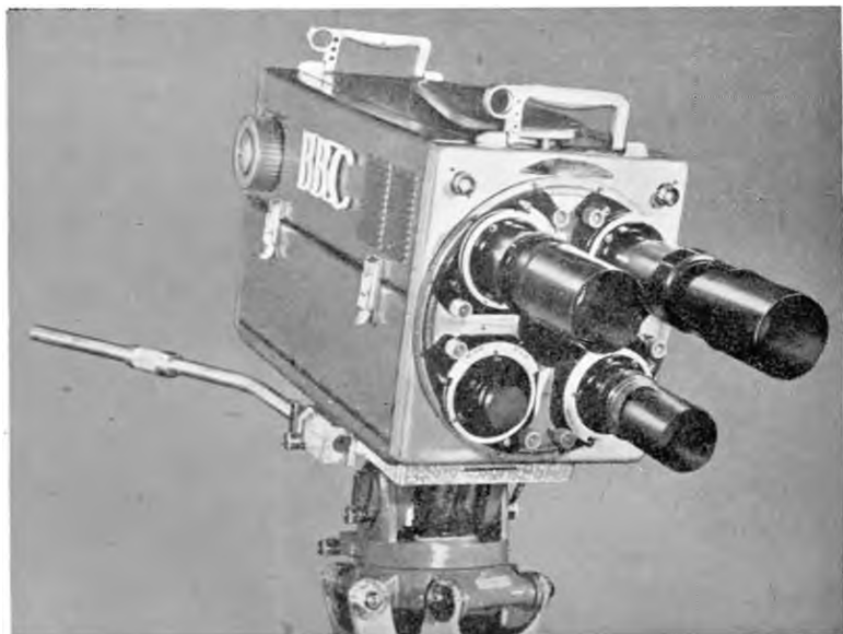
Fig. 115—An image orthicon camera with a four-lens turret
