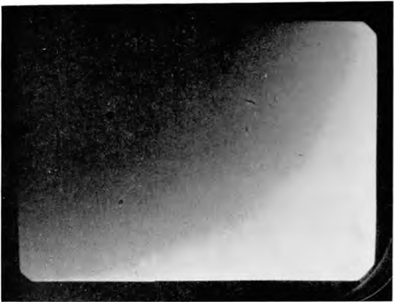
Fig. 29—Background shading due to spurious signals in iconoscope
