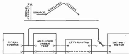
Fig. 148. Block diagram of the arrangement of apparatus when measuring the gain of any amplifier by comparing it with the loss introduced by a calibrated attenuator. If the attenuator is continuously variable over the range concerned, the only purpose of the meter is to adjust the signal level at the two points shown by the stars in the signal strength diagram to equality ; no meter calibration is needed. Note that both source and meter are at relatively low signal levels.
