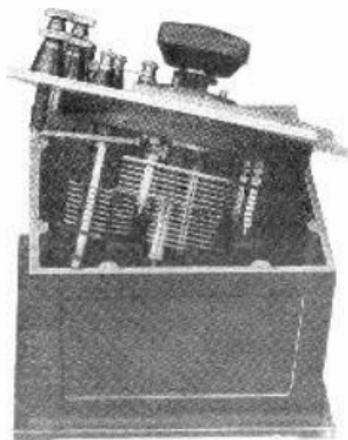
Fig. 62: Sullivan-Griffiths dual range variable condensers have many advantages for laboratory work.
