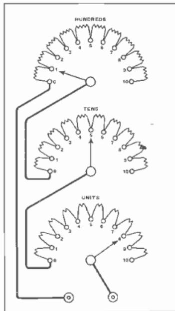
Fig. 55: Connections of a 3-figure decade resistance box, providing 1,110 ohms in steps of 1 ohm
