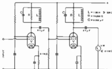
Fig. 159: Circuit of a weighted amplifier to compensate for the characteristics of the average ear, as shown in Fig. 158.
