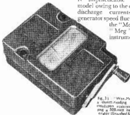
Fig. 33 - "Wee-Megger-Tester", a direct-reading ohmmeter for insulation resistance, incorporating a 500-volt hand-driven generator (Evershed & Vignoles Ltd.)
