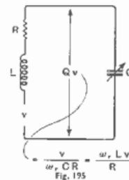
$Q$  is a measure of the "response" of a tuned circuit at resonance, and of its selectivity; and is sometimes known as the *magnification* because it is equal to the ratio of the voltage developed across the circuit to the voltage injected into it.
