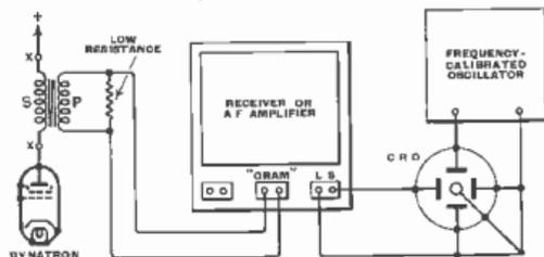
Fig. 135 : Apparatus used for measuring the natural frequency of oscillation of a transformer secondary winding with the primary virtually short-circuited. By measuring also the inductance of the secondary in this condition, the self-capacitance can be derived
