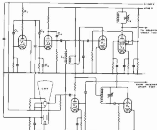
Fig. 51 All-electronic system for observing the frequency response characteristics of receivers. The valve  $V_1$  acts as a variable reactance, altering the frequency of the oscillations generated by  $V_1$ , which is one oscillator in a beat-frequency system.  $V_2$  is the fixed-frequency oscillator and  $V_3$  the mixer.  $V_4$  amplifies the receiver response before applying it to the deflector
