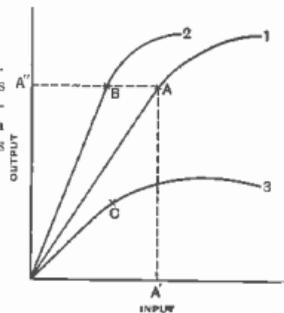
Fig. 151: Showing that a signal level that is within the capabilities of an amplifier in one set of conditions may overload it in another
