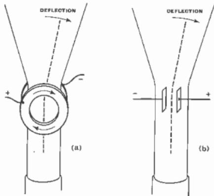
Fig. 43: Showing how (a) magnetic deflection and (b) electrostatic deflection are accomplished, and the relationship between polarity of current or voltage and the direction of deflection
