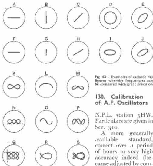
Fig 83. Examples of cathode ray figures whereby frequencies can be compared with great precision
