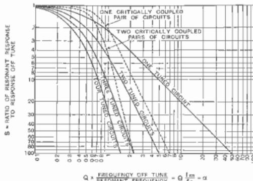
Fig. 196: Universal response curves, showing the extent to which the response falls off as the resonant frequency is departed from. Comparing one critically-coupled pair of circuits with two single circuits, it can be seen that the steepness of the slope well away from resonance is the same, but the coupled pair gives much more level response near resonance.
