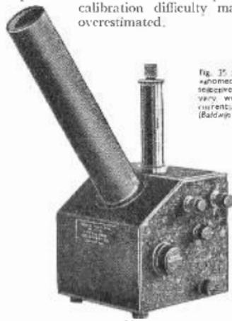
Fig. 35: Vibration galvanometer, used for sensitive detection of very weak alternating currents of about 50 c/s (Baldwin Instrument Co., Ltd.)
