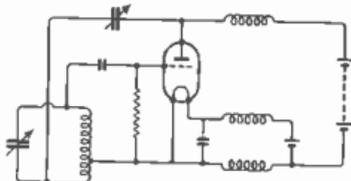
The oscillation can be controlled by a small trimmer slung in the wiring. Three chokes are shown (Fig. 170) for isolating the batteries in case it is desired to put them at some distance. In any case it is a good thing to keep the R.F. currents in their own quarters. The filament chokes must be of reasonably low resistance, and assuming
