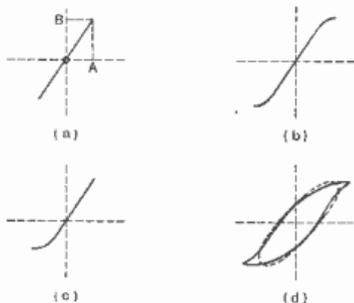
Fig. 136: Representative cathode-ray figures from which non-linearity distortion (harmonics and intermodulation) and phase shift can be deduced
