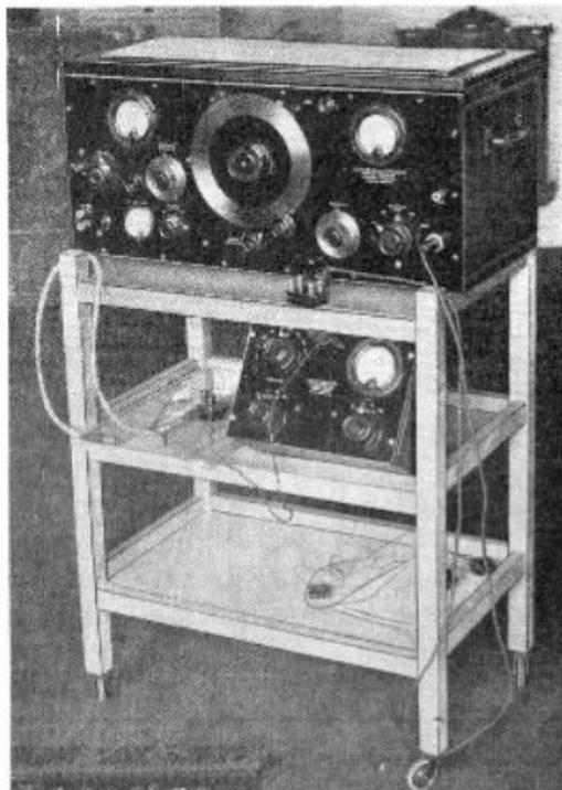
Fig. 7: Trolley mounting is particularly suitable for much-used bulky units. The instruments shown are the General Radio Co.'s 603-A Standard Signal Generator and 583-A Output Power Meter
