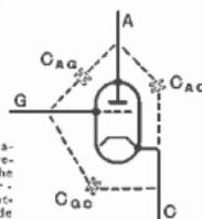
Fig. 124—Diagrammatic representation of the three inter-electrode capacitances in a triode
