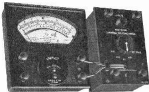
Fig 28: The Cambridge Instrument Co.'s "Unipivot" Versatile Galvanometer can be used for accurate work in conjunction with a great variety of accessories. A multi-range ohm-meter manufactured to the author's design is shown
