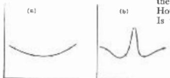
Fig 178. Two ways of drawing a curve through a series of plotted points. Which is right?
