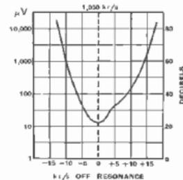
Fig. 165 : Typical selectivity curve (slightly asymmetrical) by the single-generator method
