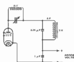
Fig. 99: Modulated R.F. is obtained by connecting audio and radio sources in series. The values shown are for modulation at about 1,000 c/s
