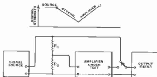
Fig. 149: It may be better in some cases for the amplifier and attenuator to be at low signal levels, source and meter being high. This is done by putting the attenuator ahead. This diagram also shows the use of a simple fixed or semi-variable attenuator to bring the meter points to approximate equality. A meter calibration is then needed as well as the attenuator calibration, but the need for wide range is avoided, as are some other disadvantages.
