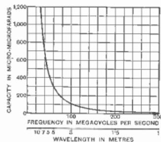
Fig. 171: Optimum capacitance of by-pass condensers, assuming the total length of connections (including the condenser itself) is about one inch
