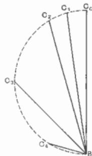
Fig. 134 : If the vector  $BC$  in the preceding figure, representing the impedance of the coil, is drawn for varying numbers of short-circuited turns, the points  $C$  lie on a semi-circle. Where the shorted turns are few, the effect on resistance is much more pronounced than on the impedance or reactance
