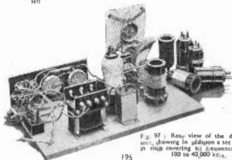
Fig. 97: Rear view of the dynatron unit, showing in addition a set of plug-in coils covering all frequencies from 100 to 40,000 kc.
