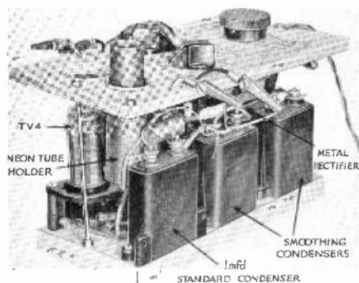
Fig. 214 Bridge with case removed
