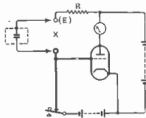
Fig. 110 - Circuit for measuring condenser leakage and other very high resistances
