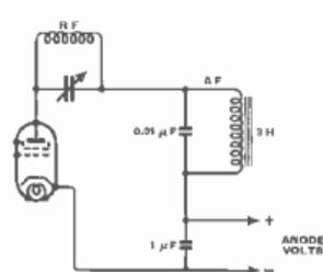
Fig. 99: Modulated R.F. is obtained by connecting audio and radio sources in series. The values shown are for modulation at about 1,000 c/s
