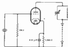
Fig. 80. Simple crystal oscillator for frequency checking
