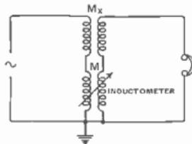
Fig. 131: Measurement of mutual inductance by direct balancing against mutual inductometer
