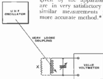
Fig. 176: Alternative arrangements for U.H.F. impedance measurement
