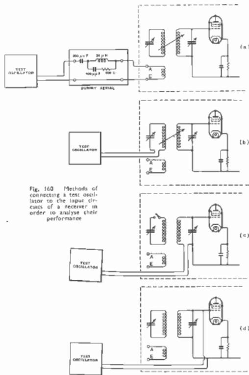
Fig. 160 Methods of connecting a test oscillator to the input circuits of a receiver in order to analyse their performance
