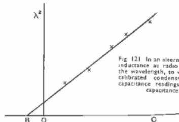
Fig. 121 In an alternative method of measuring inductance at radio frequency the square of the wavelength, to which the coil is tuned by a calibrated condenser, is plotted against capacitance readings, and the total circuit capacitance thus determined.
