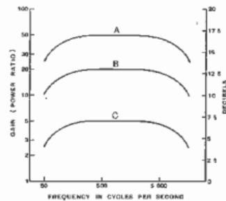
Fig. 147. When the curves of Fig. 146 are replotted on a logarithmic gain scale, which is the same as a linear decibel scale, the true proportions appear
