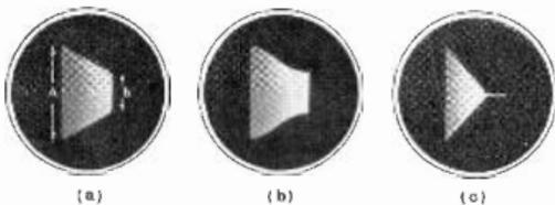
Fig. 161 Cathode-ray figures from which the purity and depth of modulation can be determined
