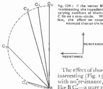
Fig. 134: If the vector  $BC$  in the preceding figure, representing the impedance of the coil, is drawn for varying numbers of short-circuited turns, the points  $C$  lie on a semi-circle. Where the shorted turns are few, the effect on resistance is much more pronounced than on the impedance or reactance
