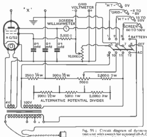
Fig. 95: Circuit diagram of dynatron test unit with switch for optional all-A.C. or semi-battery drive. An alternative fixed potential divider is shown.
