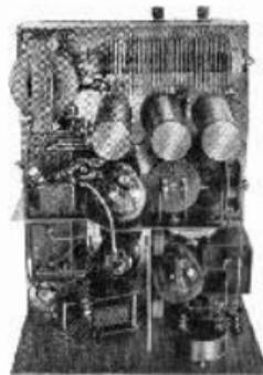
Fig. 20 Beat-frequency audio source designed by C. F. Edwards, employing triode hexode frequency changer
