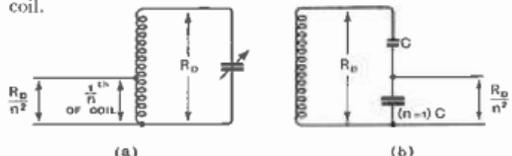
Fig. 194. How the dynamic resistance,  $R_D$ , of a tuned circuit is reduced by "tapping down," either on inductance (a) or capacitance (b) side. The impedance across the tapping points still remains a resistance.
