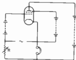
Fig. 143. Circuit for measurement of mutual conductance
