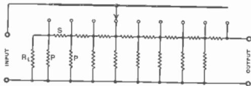
FIG. 91 : A convenient type of attenuator much used in radio work—the "Ladder"
