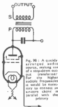
Fig. 98: A quickly arranged audio source, making use of a step-down output transformer for the higher audible frequencies it would be necessary to connect an air-core choke in parallel with the primary
