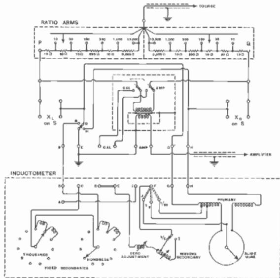
Fig. 73 - Circuit diagram of the bridge included in Fig. 72. According to the nature of the test the "unknown" is connected to terminals  $X_1$  or  $X_2$ , and extra terminals are provided for connecting resistance boxes in parallel. The inductometer may be replaced by a resistance box. The screened and balanced transformer in the center is to enable an earthed amplifier to be connected across the unearthed diagonals
