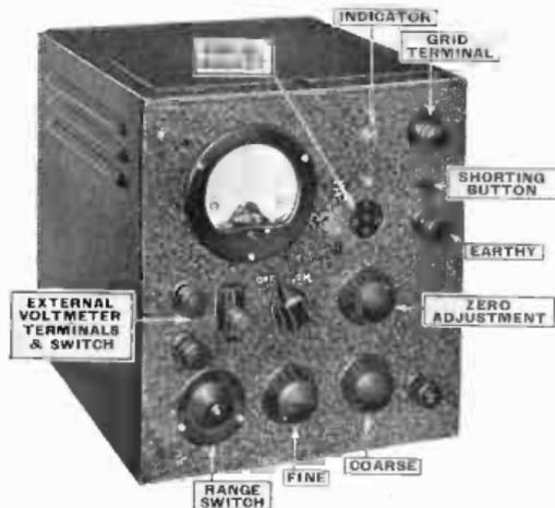
Fig. 104 : Home-made mains-driven slide-back valve voltmeter. It is completely self-contained, but an optional acorn valve probe for U.H.F. use can be plugged in as shown. The cathode-ray Indicator window is immediately above this socket
