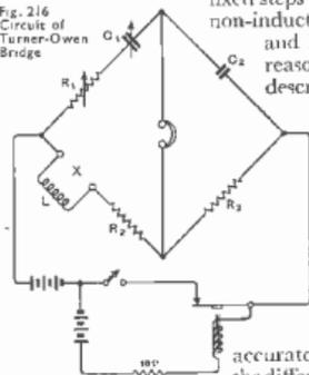
As in the Owen bridge  $L = R_1 R_2 C_2$ , the maximum values in the four ranges are 0.1, 1, 10, and 100 mH; so the total range covered is from a few  $\mu\text{H}$  to 0.1 H. The arrangement is not well adapted for measuring  $R_2$  however.
