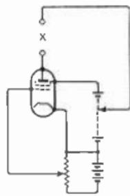
Fig. 93: Simple dynatron circuit illustrating the principle of its uses for testing
