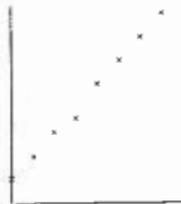
Fig 179: If it were not for one point, a straight line could be drawn through them all. Is the odd reading an error, or does it point out a fact?
