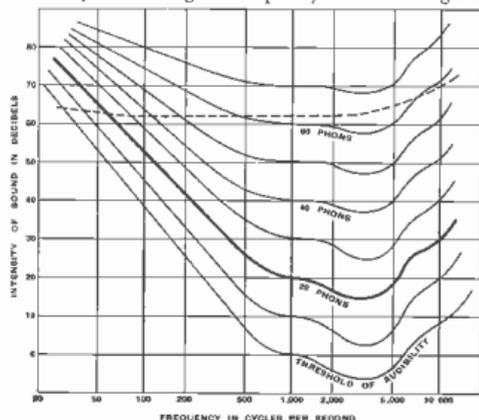
Fig. 158. Average characteristics of the human ear. The curves of equal loudness (measured in phons) are very different from the horizontal straight lines corresponding to equal intensities of sound. By using the "weighted" amplifier specified in Fig. 159 the 20-phon line is brought up to the almost level dotted line, enabling an ordinary meter to read proportionately to loudness.
