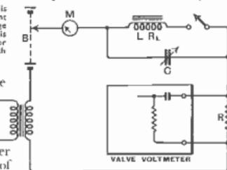
potentially accurate. One of them is illustrated by Fig. 132. The condenser C is adjusted until the current is the same whether the coil under test is switched in or not. When this condition exists,
