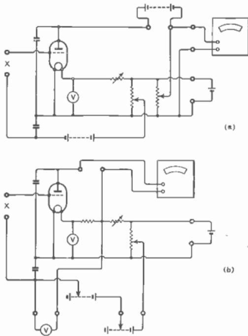
Fig. 37. Simplified circuit diagrams of Fig. 36, showing the connections when used as a valve voltmeter of the (a) anode bend and (b) slide-back types. It can also be used as a condenser insulation meter. The positions of components correspond to those in Fig. 36, which provides a key to them.
