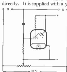
Fig. 212. Showing how a "magic eye" is employed in a bridge as detector. For circuit details see Fig. 79.
