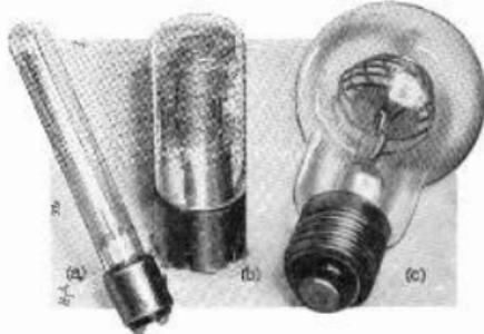
Fig. 54: Some inexpensive and very useful electronic indicators: (a) Cossor 3180 neon tuning indicator, (b) Mullard T.V.4 cathode ray tuning indicator, and (c) General Electric "Osgilim" neon lamp
