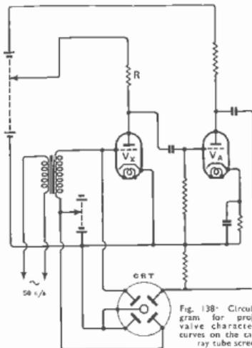
Fig. 138. Circuit diagram for projecting valve characteristic curves on the cathode-ray tube screen
