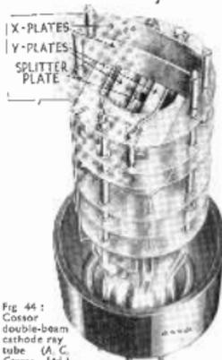
Fig. 44: Cossor double-beam cathode ray tube. (A. C. Cossor, Ltd.)
