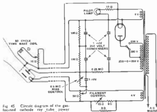
Fig. 45: Circuit diagram of the gas-focused cathode ray tube power supply unit shown in Fig. 46. It is composed entirely of standard receiver parts.
