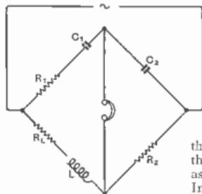
Fig. 75: The Owen bridge is more convenient than the Maxwell for inductance measurement with a fixed condenser
