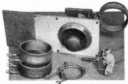
Fig 82. Simple absorption wavemeter and coils: the larger covers 2 to 100 Mc/s and the smaller is for quick checking of decimetre waves
