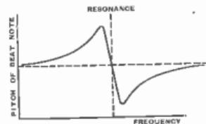
Fig 86 - The "N-curve", showing the disturbing effect of a loosely-coupled circuit tuned through resonance; a phenomenon that is helpful in synchronising circuits very exactly
