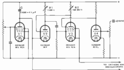
Fig. 48 Schematic circuit diagram of hard valve linear time base circuit (due to O. S. Puckle)
