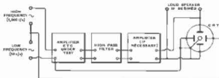
Fig. 156. Apparatus for testing amplifiers for intermodulation, due to non-linearity
