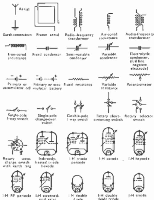
Fig 103 Symbols used in circuit diagrams
