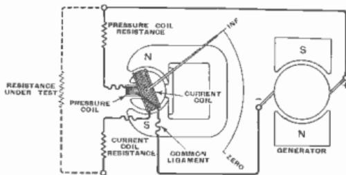
Fig. 34 - Circuit diagram of the "Wee-Megger-Tester". With infinite resistance, current flows only through the pressure coil, causing the pointer to be held in the full-scale position. Any current flowing through the resistance under test traverses the current coil and causes a corresponding deflection (Evershed & Vignoles Ltd.)
