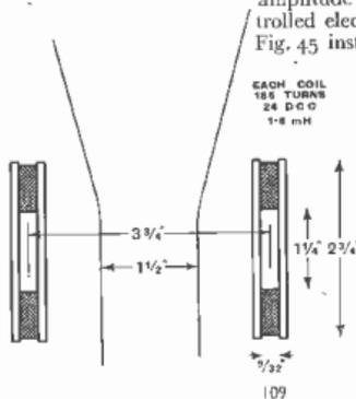
Fig. 47: Dimensions of coils suitable for providing a uniform 50-cycle deflecting field
