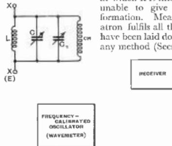
Fig 118: Apparatus used for measuring the resistance and reactance at working frequencies of a R.F. choke, Ch. This is typical of many measurements that can be made by means of a dynatron oscillator.
