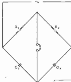
Fig. 113 (left) The simplest capacitance bridge, in which no account is taken of the resistive properties of the condenser
