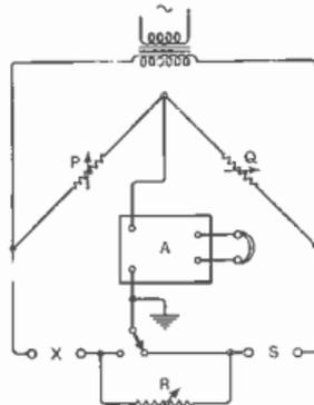
Fig. 70 - Diagram of a general purpose A.C. bridge, for which external standards of reactance must be provided
