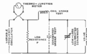
Fig. 128 Schematic diagram of Q meter
