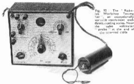
FIG. 92 The "Radio-lab Workshop Testing Set" is an exceptionally versatile instrument with direct-reading scales. Note the valve voltmeter "probe" at the end of the screened cable.
