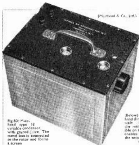
Fig. 60: Muirhead type 18 variable condenser with geared drive. The metal box is connected to the rotor and forms a screen
