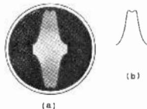
Fig. 166 : How selectivity curves appear on the cathode-ray screen when (a) the R.F. or I.F. signal and (b) the rectified and filtered Z.F. output are used
