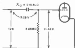
Fig. 192: A typical example of vectorial addition of voltages and impedances
