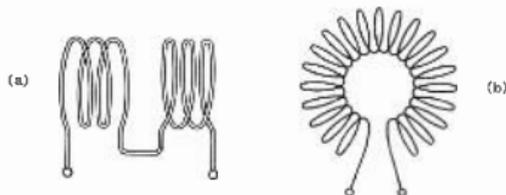
Fig. 66. Two methods of reducing the external field of coils—(a) the astatic pair, consisting of two adjacent coils with opposite rotation and (b) the toroid, consisting of a long solenoid bent round into a circle.
