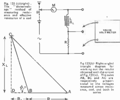
Fig. 133 (b) - Right-angled triangle diagram for working out the results obtained with the circuit of Fig. 133 (a). The sides  $AB$ ,  $BC$  and  $AC$  are respectively proportional to the voltages measured across resistance, coil, and both in series
