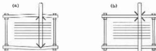
Fig. 59: Two types of condenser bearing. Type b in which the end-plates are not under a separating stress, is to be preferred for permanence of calibration.
