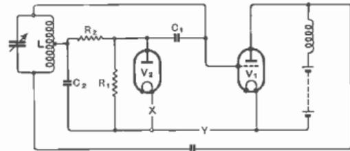
Fig. 16: Automatic oscillation control. The grid bias for the oscillator valve  $V_1$  is derived from the oscillation itself, rectified by  $V_2$ . Modulation can be introduced at X or Y.
