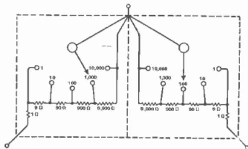
Fig. 68. Diagram of a pair of switched ratio arms for A.C. bridges
