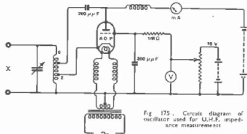
Fig. 175. Circuit diagram of oscillator used for U.H.F. impedance measurements
