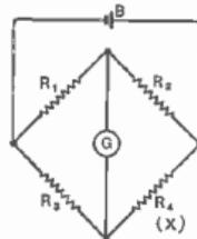
Fig. 67. Simple Wheatstone Bridge, on which nearly all other forms of bridge are based
