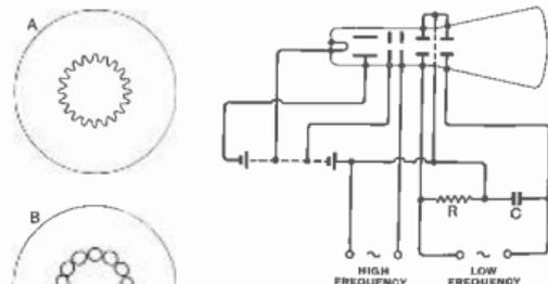
Fig. 84: Circuit for comparing frequencies related by a larger ratio than is easy to distinguish from the figures of Fig. 83. The ratio is found by counting the "teeth" in the figure A, or half the number of loops in figure B. Intermediate ratios are determined by speeds of rotation as described.
