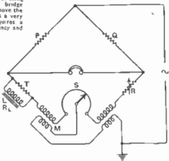
Higher inductances still, with practically no top limit, are measurable by shunting the coil with a non-reactive resistance T (Fig. 130). The arm thus formed is equivalent to a comparatively low inductance in series with a resistance, and by this device is brought within the equal-ratio range. T is in general equal to the initial value of R, and having made the preliminary zero adjustment with L disconnected, balance is obtained with L in position.
