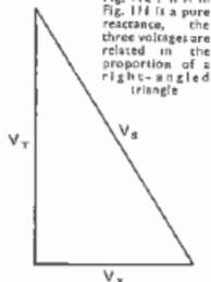
Fig. 112 : If X in Fig. 111 is a pure reactance, the three voltages are related in the proportion of a right-angled triangle
