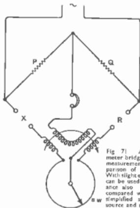
Fig 71 An inductometer bridge circuit, for measurement or comparison of inductances. With slight elaboration it can be used for capacitance also. Note that, compared with Fig 70, simplified symbols for source and detector are used.
