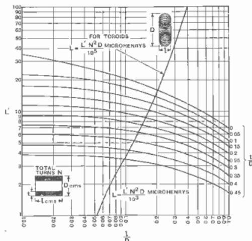
Fig. 200: Data sheet compiled from standard formulae by Mr. F. Charman, by which the inductance of coils of all shapes can easily be found
