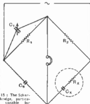
Fig. 115 : The Schering bridge, particularly suitable for measuring the loss factors of small condensers
