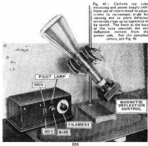
Fig. 46: Cathode ray tube mounting and power supply unit. Note use of rotor's stand to adjust screen to convenient angle for viewing and to place deflector terminals close up to apparatus to be tested. The knob at the base of the tube controls the coil deflection current from the power unit. For the complete circuit, see Fig. 45.
