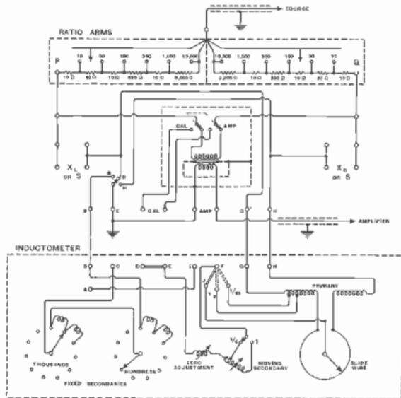
Fig. 73 - Circuit diagram of the bridge included in Fig. 72. According to the nature of the test the "unknown" is connected to terminals  $X_1$  or  $X_2$ , and extra terminals are provided for connecting resistance boxes in parallel. The inductometer may be replaced by a resistance box. The screened and balanced transformer in the center is to enable an earthed amplifier to be connected across the unshielded diagonals
