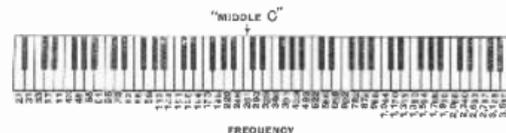
Fig 85 ; Piano scale showing the frequencies to which the keys are tuned. The usually-published scales based on C=256, are misleading. Frequencies of black keys can be obtained by multiplying the frequency of the white key below it by 1.059
