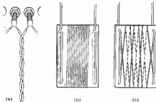
Fig. 56. Three of the many methods of transmitting reactance in elements. (a) The "twisted hairpin" is suitable for low resistance; (b) consists of fine wire wound on a thin mica card, which is stiffened by the thick wire connecting leads. In (c) (the Ayrton-Perry method) there are two windings in parallel, in opposite rotation to neutralise self-inductance.
