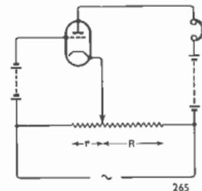
Fig. 141 : Simple bridge circuit for measuring  $\mu$ . For more accurate work especially with high- $\mu$  valves, it is necessary to balance out stray capacitances as shown in the next figure
