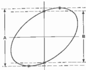
If the loss factor of  $C_X$  is very bad it causes an appreciable departure from the circular form; the dimensions A and B (Fig. 117) enable the phase angle and hence the loss factor to be calculated, for  $\sin \phi = B/A$ .
