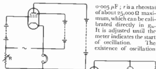
Fig. 143. Circuit for measurement of mutual conductance
