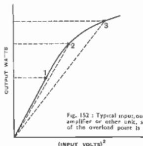
Fig. 152 : Typical input-output characteristic of an amplifier or other unit, showing how estimation of the overload point is a matter for judgment
