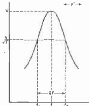
Fig. 127. Resonance-curve method of measuring R.F. resistance.
