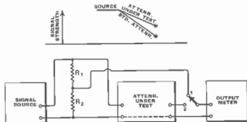
Fig. 150—Here two attenuators are being compared and the only difference in method is that they are connected in parallel instead of series. If possible the standard is adjusted to make the two stars coincide.
