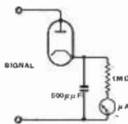
anode circuit of which is a suitable meter. An easily obtainable and effective type of diode for U.H.F. use is the Mazda D.1 (Sec. 68).
