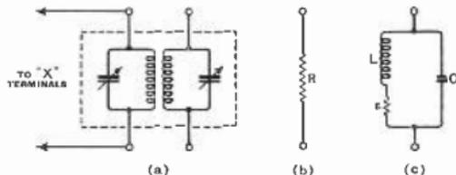
Fig. 120 : An I.F. transformer represented by the diagram (a) or any other tuned circuit, however complex, is equivalent at resonance to a high resistance  $R$  (b) which is the quantity measured by the dynatron apparatus. Alternatively it can be represented in the form (c)
