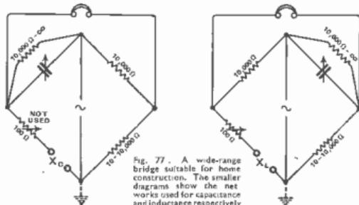
Fig. 77: A wide-range bridge suitable for home construction. The smaller diagrams show the net works used for capacitance and inductance respectively
