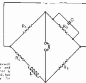
Fig. 74 - Theoretical diagram of Maxwell bridge for comparing inductance and capacitance. If a standard of either is available, the other can be measured, but certain precautions are necessary for practical success
