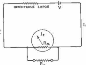
Fig. 106. Scheme for measuring low resistances
