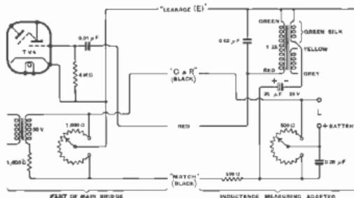
Fig. 215. Circuit of auxiliary bridge for measuring iron-core coils
