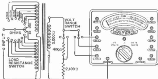
Fig. 106. Circuit of unit for adding to multi-range test set to convert it into an output meter
