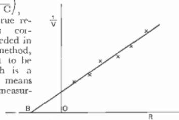
Fig. 126. Method of plotting the results derived from the system of Fig. 125 to get  $r'$ , the R.F. resistance, neglecting the self-capacitance,  $C_1$ , of the coil. Knowing  $C_1$ , the true resistance  $r$  can be calculated.
