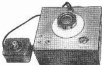
A good example is the "Radiolab" modulated oscillator illustrated here, covering 100-30,000 kc/s in five switch-controlled ranges. Either internal 400 c/s or external modulation is possible, and the internal signal is available for A.F. tests. The attenuator in the separate small box controls the output between the limits of approximately 1 and 100,000 microvolts. The price is £9 17s. 6d. for battery drive and £10 17s. 6d. for A.C. mains.
