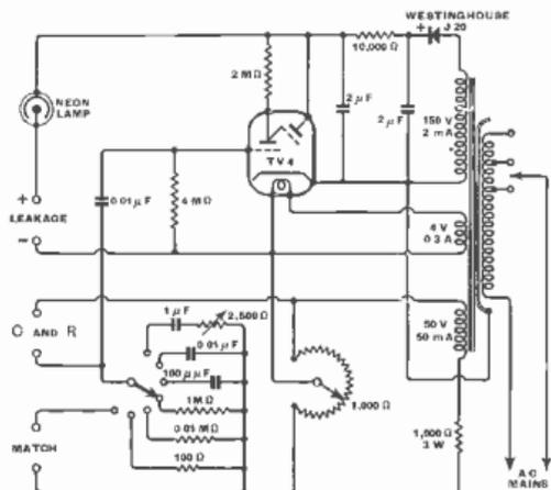
Fig. 79: Diagram with values of a self-contained mains-driven resistance and capacitance bridge employing a "magic eye" as amplifier-detector. For constructional details and pictures refer to Appendix, p. 384. The nature of the scale, assuming a uniform resistance element, is shown above
