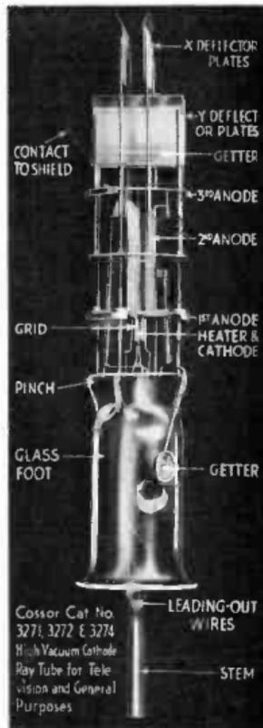
position of the spot (known as *origin distortion*); modulation of the spot's brightness (as in television) is not practicable; and only tubes with directly-heated cathodes are obtainable.
