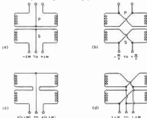
Fig. 64. Various methods of connecting a 4-coil inductometer, giving approximately the mutual and self inductances shown, where  $L$  is the self inductance of one coil and  $M$  the maximum mutual between one pair of coils
