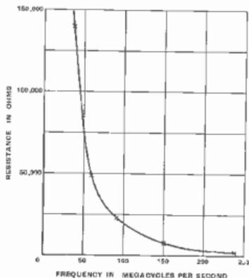
Fig. 180: The general law connecting input resistance of a valve with frequency is not obvious from a curve plotted in this way
