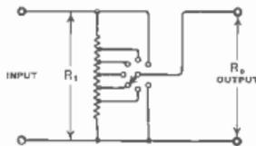
Fig. 88 The simple potential divider can be used as an attenuator within certain restrictions
