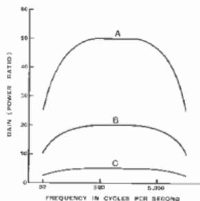
Fig. 146: Three characteristic curves plotted on an ordinary magnification or gain scale. The general appearance of the curves leads to quite wrong conclusions.
