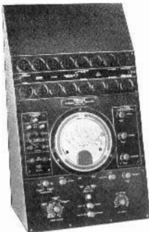
Fig. 137. Radiolab Visual Valve Tester, providing for a wide range of tests on valves of many types (Errect Edgcomb & Co., Ltd.)
