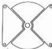
Fig. 49: Shapes of moving and fixed vanes of a rotating condenser for providing a continuous linear variation of capacitance with time in observing frequency characteristics by cathode ray tube
