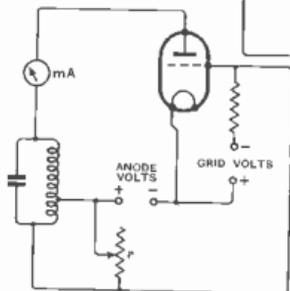
Fig. 145. Another mutual conductance meter, depending on the ability of the valve under test to set up oscillation
