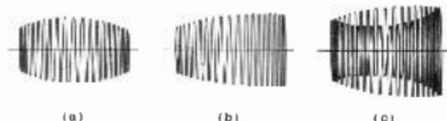
Fig. 157. Typical cathode ray figures displaying intermodulation
