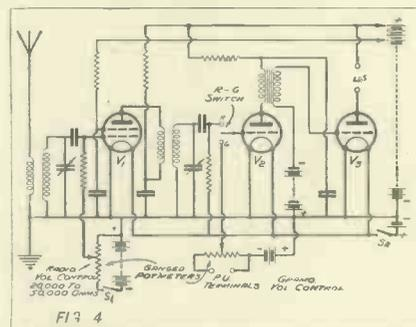
In this S.G., det. and L.F. circuit the multi- $\mu$  and radiogram volume control are ganged together.
