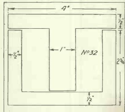
Fig. 2. The core of the component is shaped like this, two sets of stampings being used
