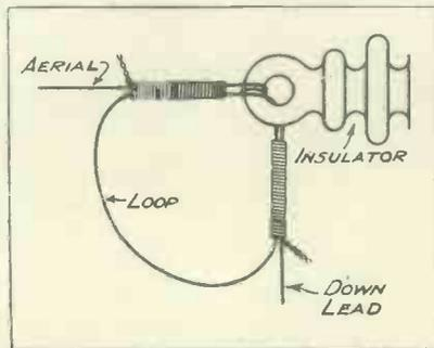
Fig. 2. The suggested method of arranging the down-lead.
