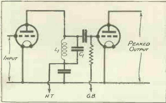
Fig. 1. The fundamental low-frequency arrangement for obtaining a peaked output.  $L_1, C_1$  is tuned to the particular frequency to which it is desired to give greater amplification.
