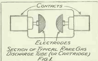
A simple gas discharge tube consisting of two electrodes inside a glass bulb filled with a gas, such as neon, at a very low pressure.
