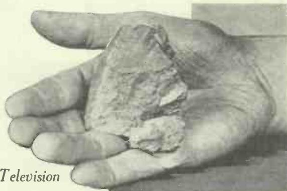
There is sufficient "active substance" in this piece of natural zinc silicate ore to make several hundred fluorescent screens for television viewing.
