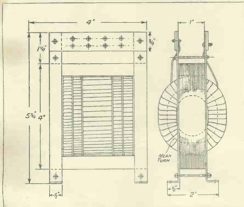
Fig. 3. The general outline of the transformer is seen here and also the method of clamping the stumpings of the core. Note that the clamping bolts are well clear of the core.
