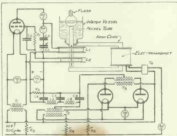
The circuit arrangement used in Professor Gaines' experiments with super sound waves.
