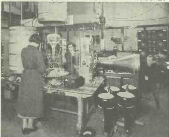
Some of the apparatus used in the Wembley Research Laboratories for the development of cathode-ray tubes. Note the cylindrical shields which are placed over the tubes while they are being exhausted.
