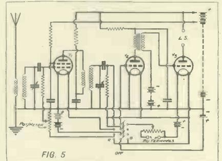
By means of this circuit the whole set can be controlled with a single switch.
