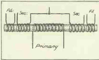
Fig. 1. The diagram of connections of a typical mains transformer.
