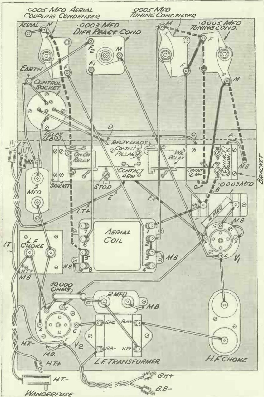
Insert all the double-line connections, and then add the dotted or solid ones as explained in the text. The points marked M.B. indicate connections to metallised baseboard.
