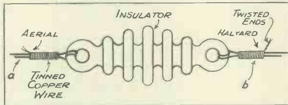
Fig. 1. How to fix the wire and halyard to the insulator.
