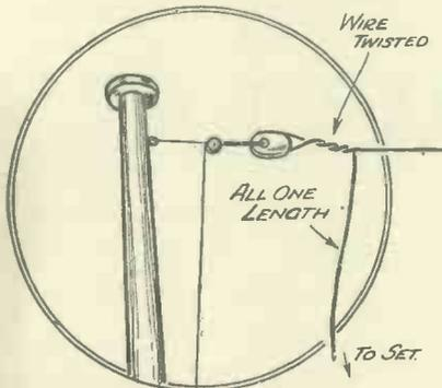
Bad joint can be completely avoided in this simple way.
