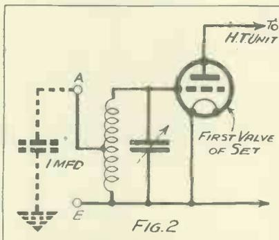
*The aerial terminal is connected to earth via a 1-mfd. condenser, while the earth terminal has no connection made to it. No other components are required.*
