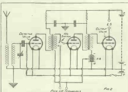
A "Det. and Two L.F." class of receiver with the radiogram switch in the first L.F. valve's grid circuit.
