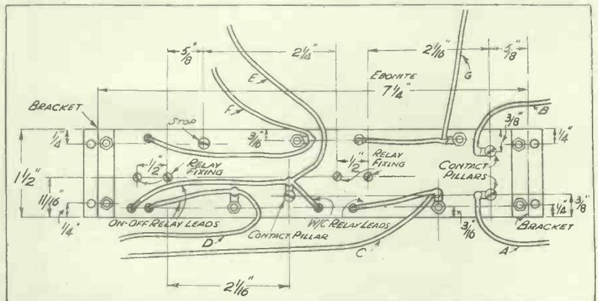
This is the underneath of the relay strip seen in the wiring diagram above. Note that it is shown turned over from top to bottom and not from left to right.
