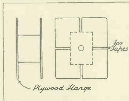
Fig. 4. The formers should be made like this, with places for tapes so that the windings can be fixed.
