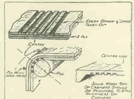
Both ply-wood and plain wood may be treated in this way for rounding corners.
