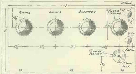
You can save the trouble of drilling your panel if you buy a kit of parts complete. The panel will then be supplied ready drilled.
