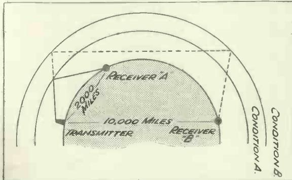
Fig. 3. Sometimes freak reception of ultra-short waves is caused by the lower layer temporarily reflecting them.
