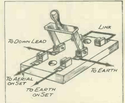
Fig. 3. The connections for the earthing switch.
