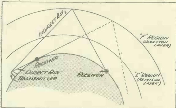
Fig. 1. The "shorter" short waves pass through the lower ionised layer and are reflected by the Appleton Layer.
