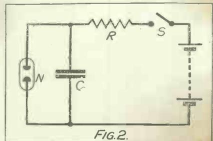
An ordinary neon lamp can, when set up in this circuit, be employed as a generator of electrical oscillations.
