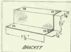
*Details of the supports, one of which goes at each end of the relay strip.*
