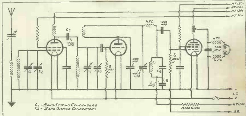
Fig. 3. Here is the complete circuit of the receiver. The H.F. side is quite conventional and normal component values are employed.
