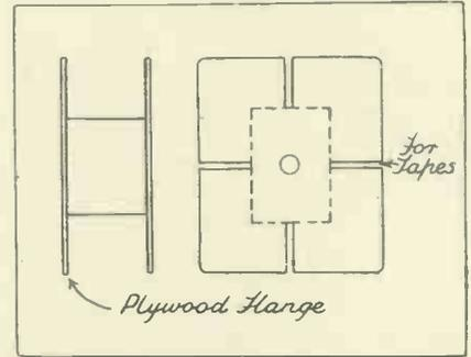
Fig. 4. The formers should be made like this, with places for tapes so that the windings can be fixed.
