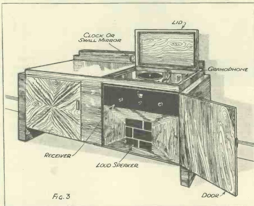
This ambitious design allows for a record turntable as well as for an electric clock, and part of it can be used as a sideboard in the ordinary way.
