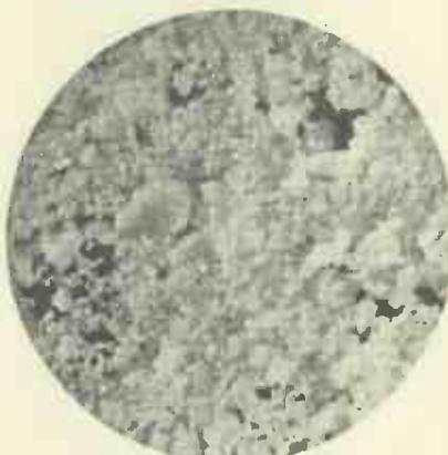
*A small area of the screen of a cathode-ray tube as seen under the microscope.*
