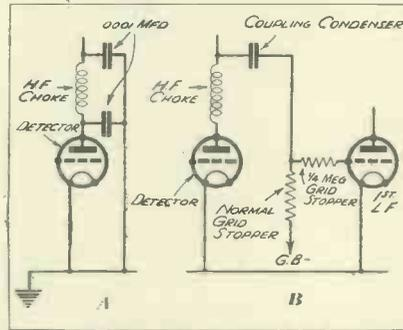
Two methods of improving the stability of a circuit. The second scheme (B) is only applicable to resistance-capacity-coupled amplifiers.
