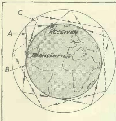
Fig. 2. Showing how signals may reach a receiver via a number of different paths.
