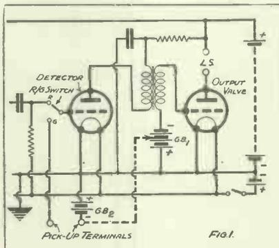
This arrangement uses the detector as an L.F. amplifier for gramophone work.
