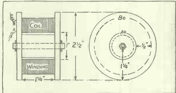
Fig. 2. This is the special inductance recommended by the author. No. 38 S.W.G. enamelled wire is used, 5,000 turns giving the required value.
