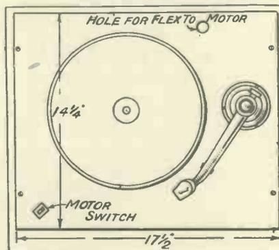
This board is arranged to fit inside the drawer about one inch from the bottom.
