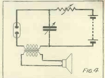
The oscillations generated by the neon lamp can be made audible in the loud-speaker.
