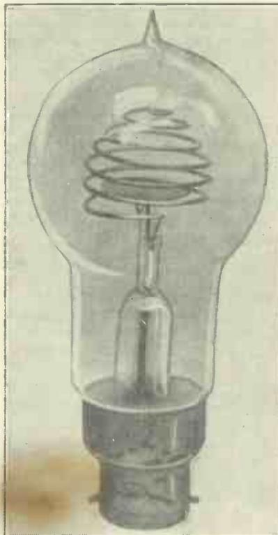
This gas discharge tube may be purchased at any electrician's and has many uses for the amateur radio experimenter.
