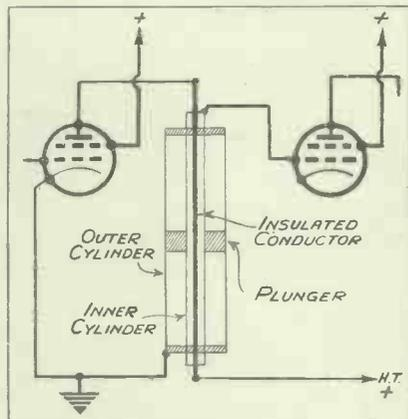
Fig. 1. This is a single stage in the new type of circuit described by W. L. S. in the text.
