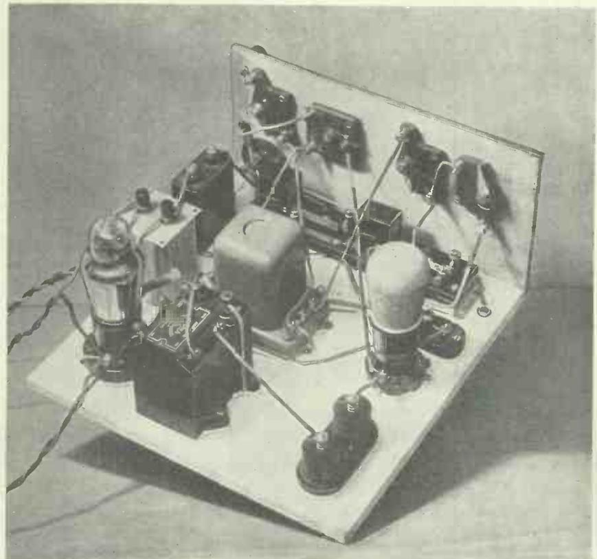
*In this view the receiver is seen in its completed form. The wiring shown is that for the reception of two medium-wave transmissions.*
