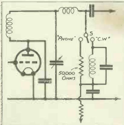
Fig. 4. If it is desired to receive telephony as well as C.W., the L.F. side of the circuit should be modified as shown above.
