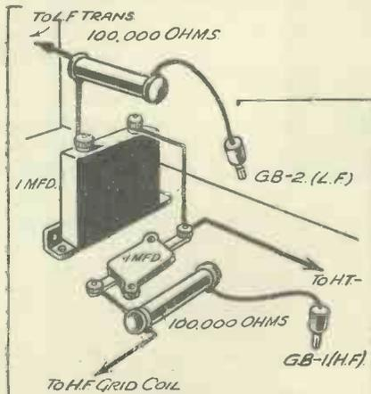
Different component values are used for H.F. and L.F. stages.
