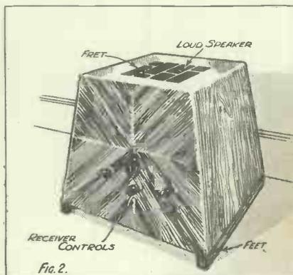
*A compact design very suitable for a three-valver. Note the unusual position for the loudspeaker.*
