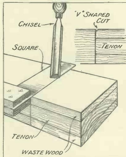
Tenon joints should be deeply marked with a chisel as shown here.
