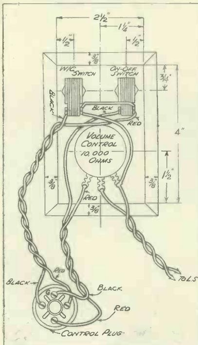
Dimensional and wiring details of the switch panel and control plug.
