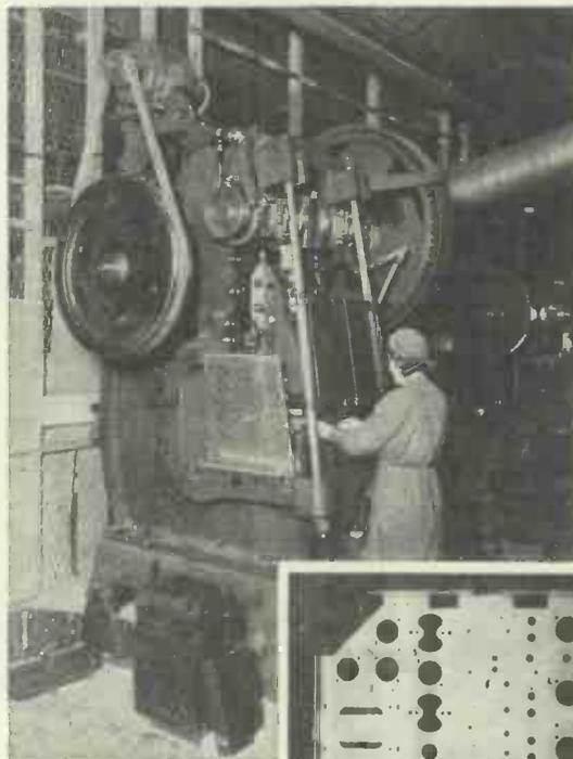
*This press is employed at the Southend works of Messrs. E. K. Cole, Ltd. for making the chassis of receivers. The inset photo shows how the chassis appears after leaving the machine.*
