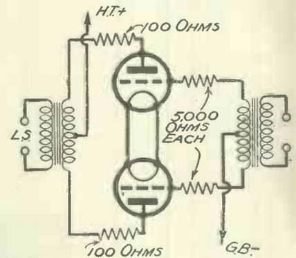
The resistances shown in this circuit will stop distortion due to parasitic oscillation.
