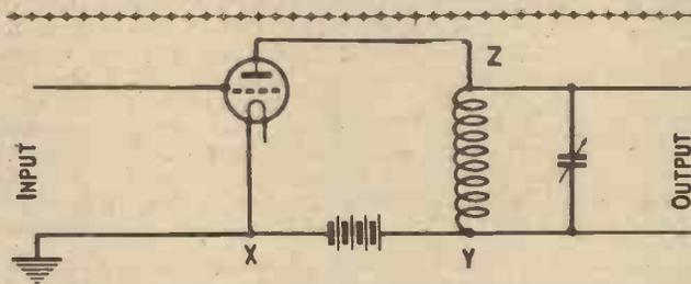
Fig. 1.—The simplest form of tuned-anode circuit.
