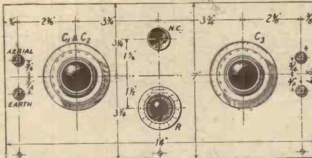
Fig. 1.—Symmetry is the keynote of the panel layout, full dimensions of which can be obtained from this diagram. Blue Print No. W2009A.
