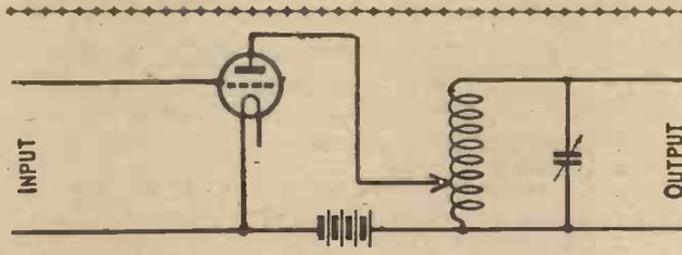
Fig. 2.—A skeleton circuit in which an auto-transformer is employed.
