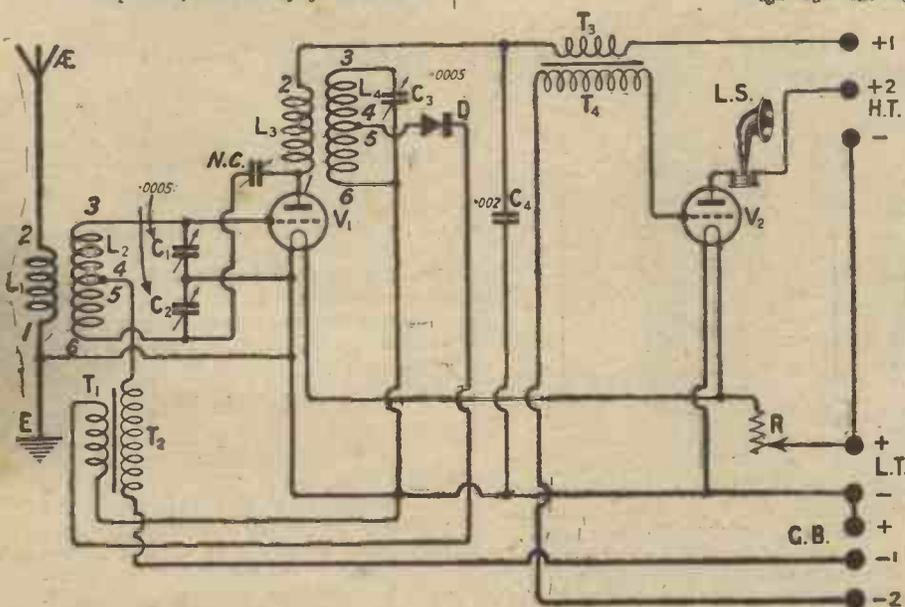
Fig. 3.—The condensers C1 and C2, form the dual condenser and both are operated by one knob.
