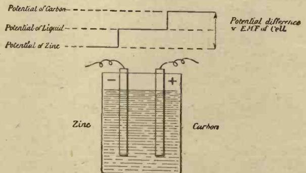
Fig. 7.—Potential difference between ends of conducting wire maintained by means of battery.
