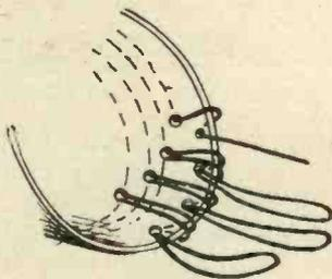
Fig. 10.—Inside of coil showing tappings.
