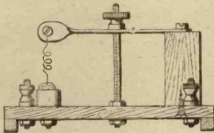
Fig. 9.—Elevation of crystal detector.
