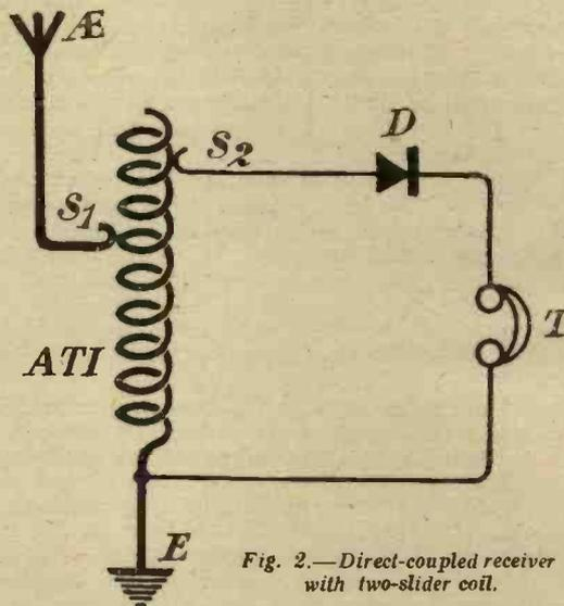
Fig. 2.—Direct-coupled receiver with two-slider coil.
