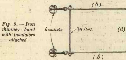
Fig. 9. — Iron chimney-band with insulators attached.
