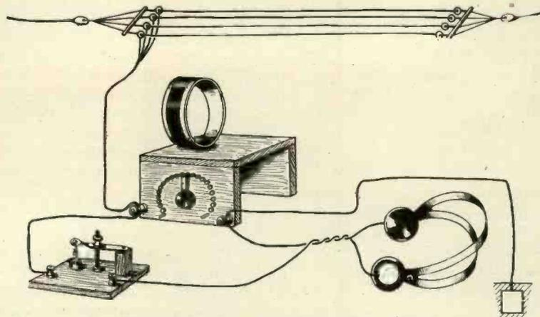
Fig. 4.—Arrangement for use on long aerials.
