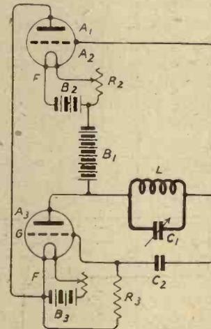
Fig. 7.—Showing use of two ordinary valves.
