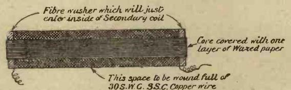
Fig. 2.—Showing new primary winding.
