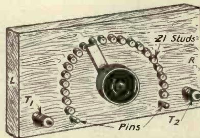
Fig. 14.—Arrangement of selector switch.
