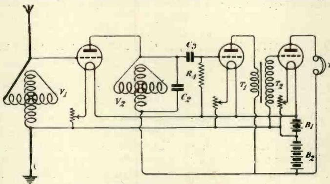
Fig. 5.—Circuit diagram of three-valve receiver.
