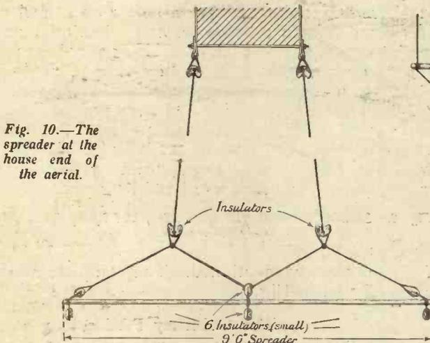
Fig. 10. — The spreader at the house end of the aerial.
