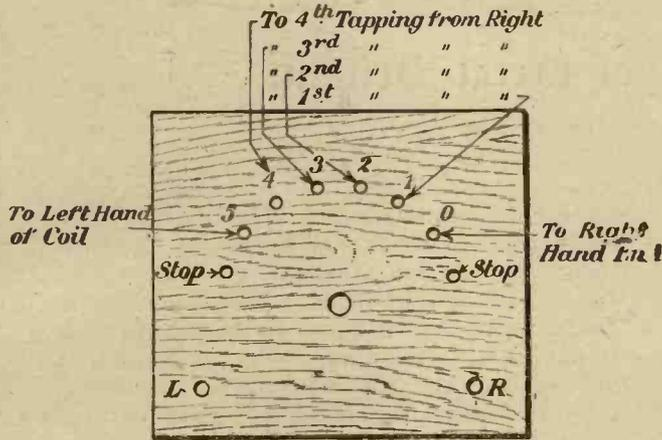
Fig. 6.—Arrangement of studs and terminals.
