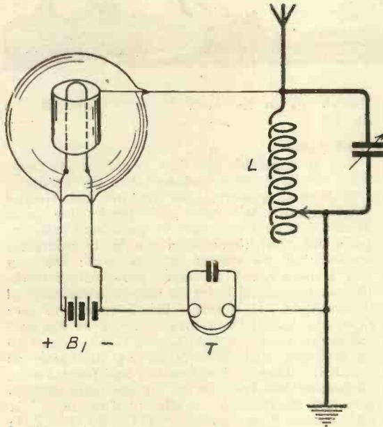
Fig. 14.—Circuit for use with 2-electrode valve.
