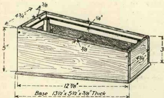
Fig. 3.—Details of the containing box.
