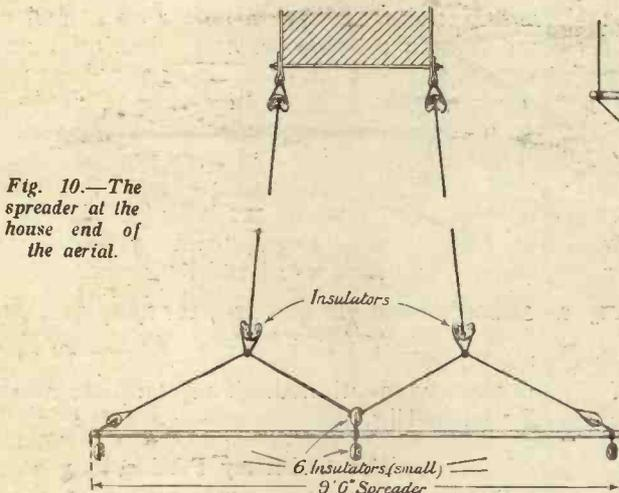
Fig. 10. — The spreader at the house end of the aerial.
