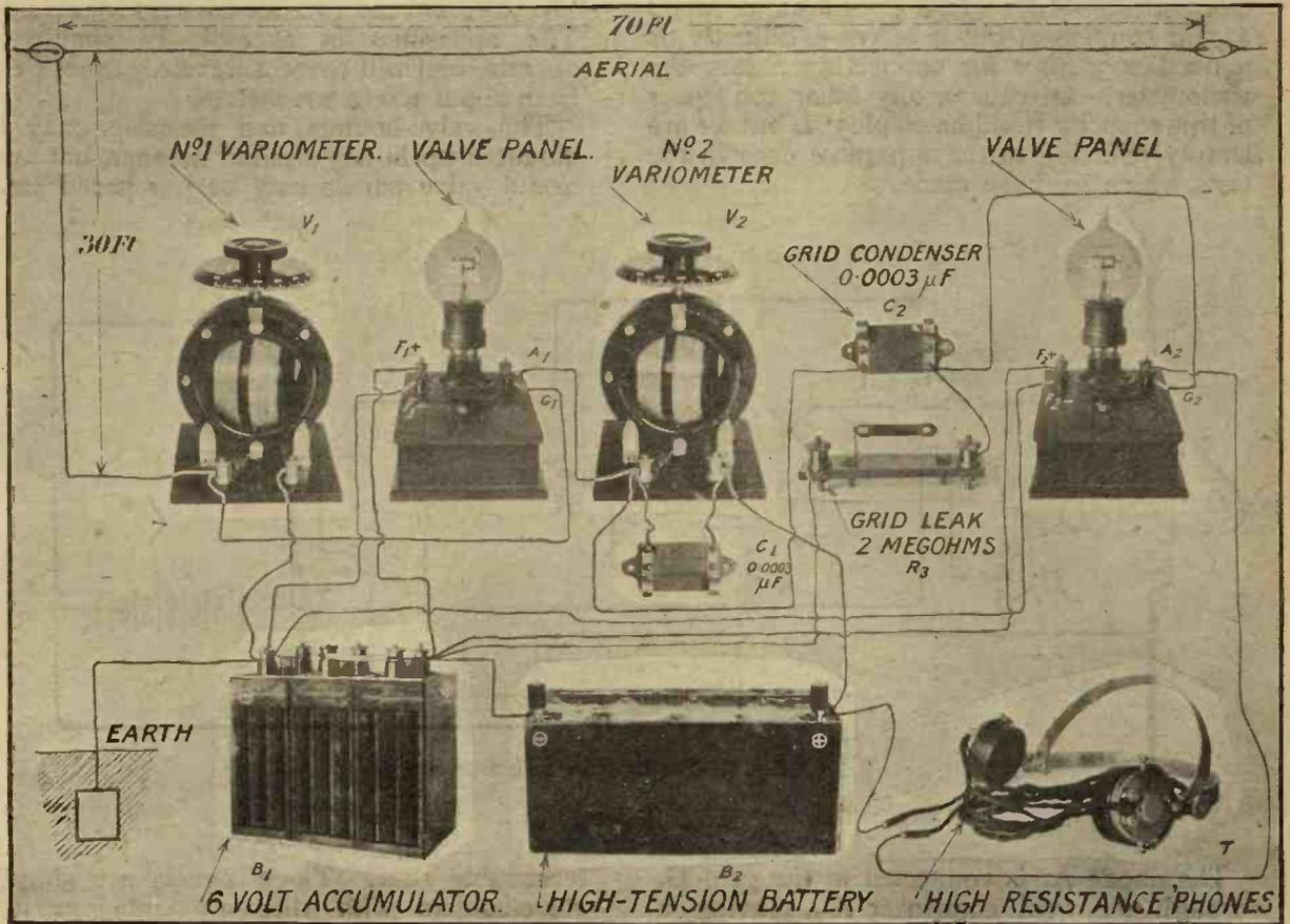
Fig. 2.—Showing how the different components are connected together
