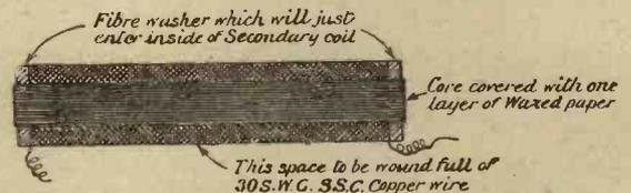
Fig. 2.—Showing new primary winding.
