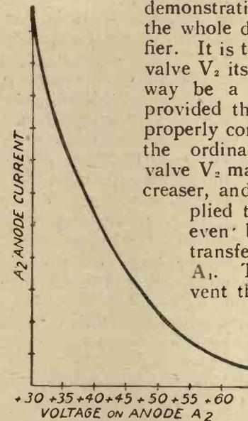
Fig. 3.—Characteristic curve of valve.
