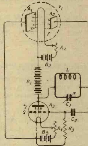
Fig. 6.—Circuit for producing oscillations.
