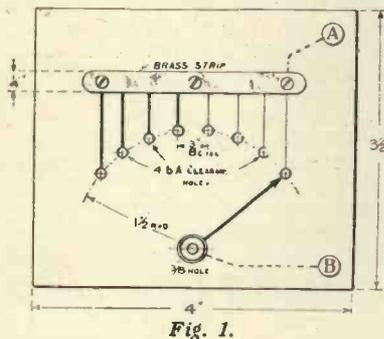
A piece of 1/4-inch ebonite measuring 3 1/2 inches by 4 is marked out and drilled as shown in the drawing. The central hole is for the spindle of a rotary switch arm, which can be bought complete with nut and bush for about 1s. from advertisers in this Journal. The circumferential holes, made with a 4 B.A. clearing drill, are for studs of the ordinary type, from eight to a dozen of which may be fitted.
