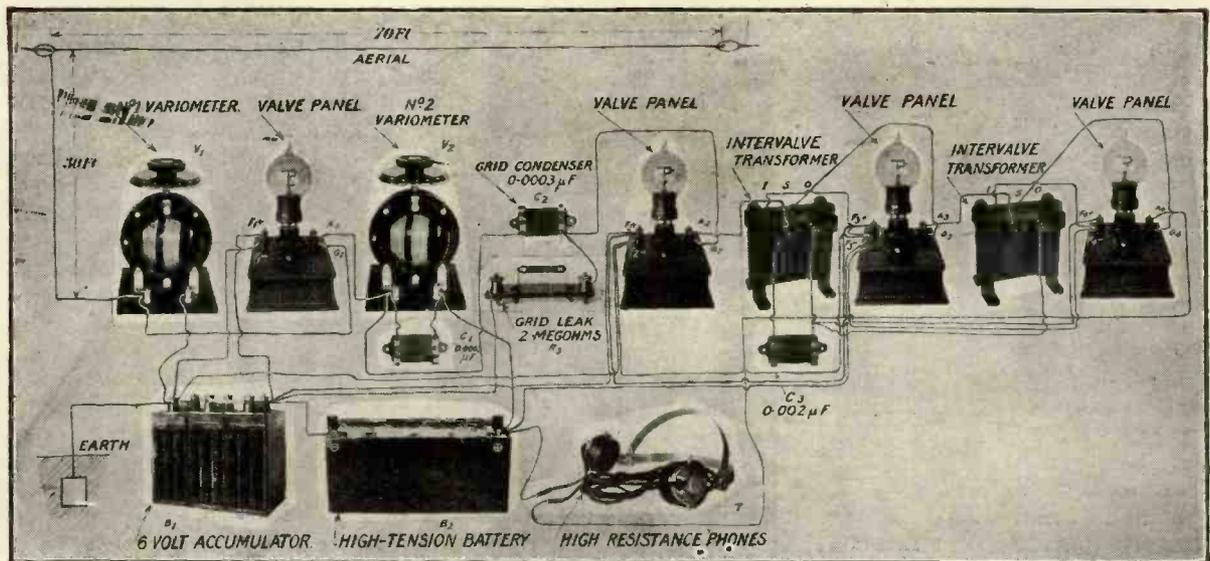
Fig. 6.—The four-valve receiver.
