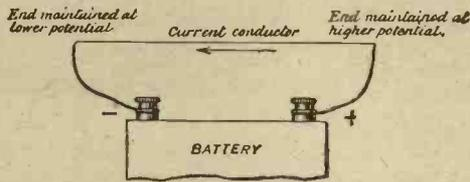
Fig. 6.—Diagrammatic representation of the potential differences existing between the elements of an electric cell.
