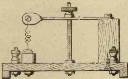
Fig. 9.—Elevation of crystal detector.
