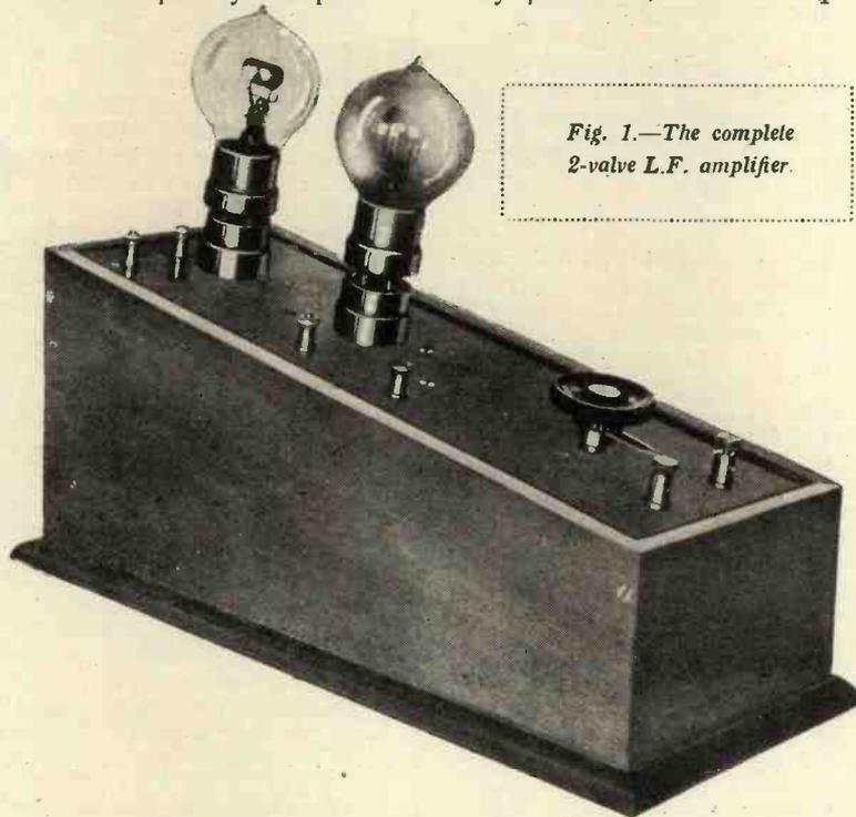
Fig. 1.—The complete 2-valve L.F. amplifier.
