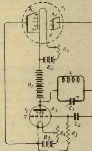
Fig. 6.—Circuit for producing oscillations.
