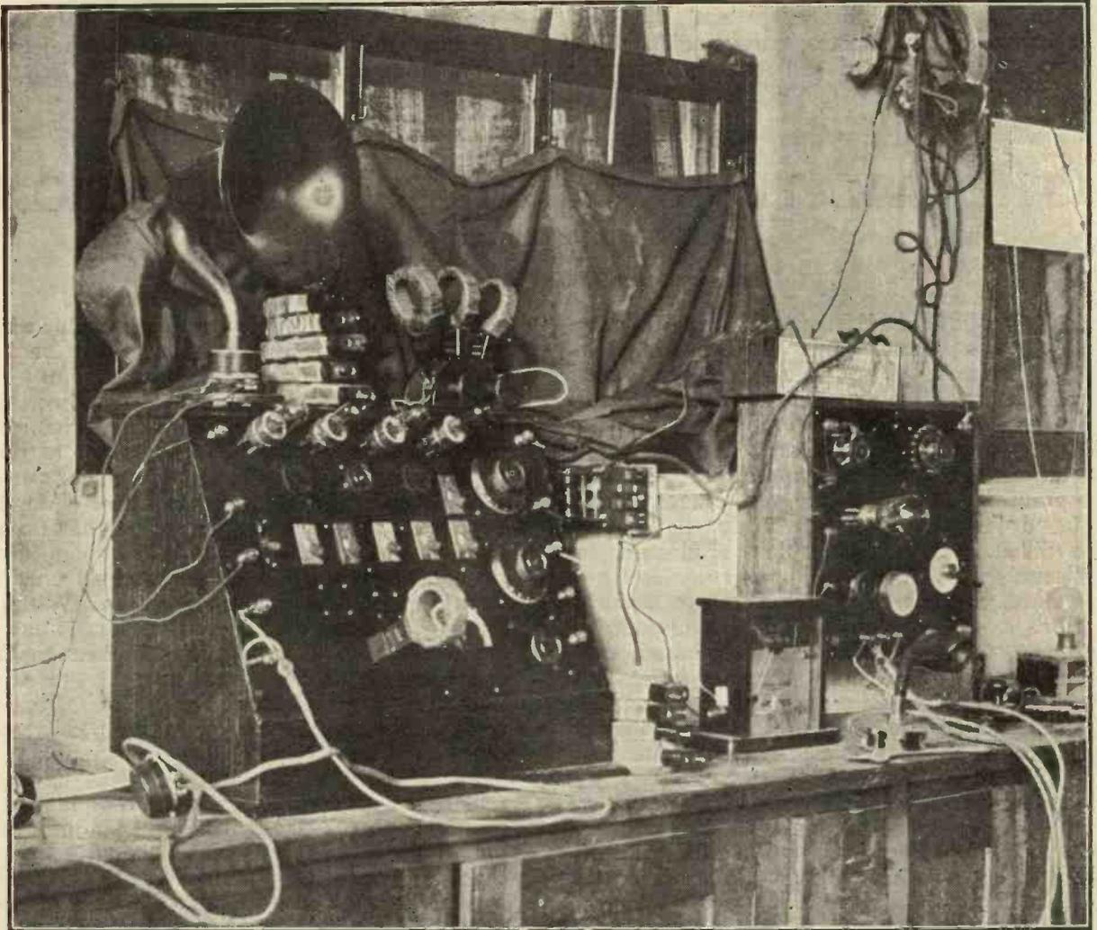
**T**HE above photograph shows the wireless installation at the Lowestoft Secondary School, owned by the Physics Master. The set comprises a four-valve receiver and a C.W. and telephony transmitter, the former being shown on the left and the latter on the right.
