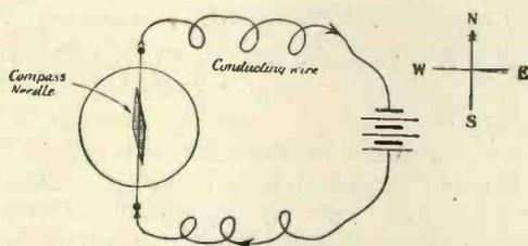
Fig. 9.—Plan showing how wire carrying current, held above compass needle, deflects North Pole to left when current is passing from South to North.
