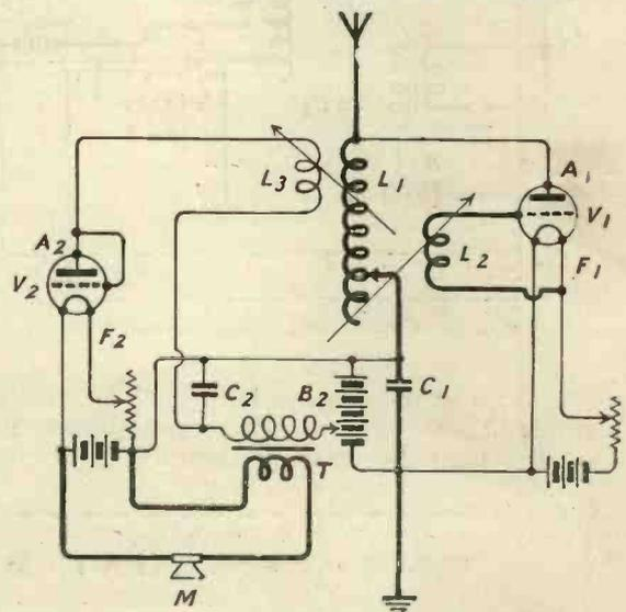
Fig. 4.—An arrangement using a common anode battery.
