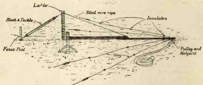
Fig. 8.—Showing the mast with stays fitted, and lifting tackle all ready for erection.
