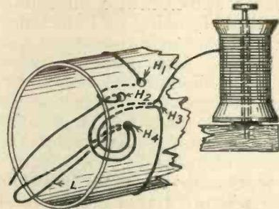
Fig. 6.—The first tapping completed.
