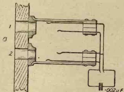
Fig. 8.—Telephone plug mounting.
