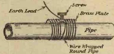
Fig. 2.—Method of tightening binding wire.
