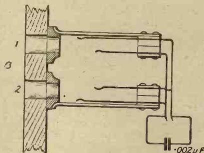
Fig. 8.—Telephone plug mounting.
