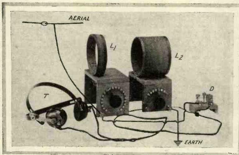
Fig. 1.—The complete receiver.
