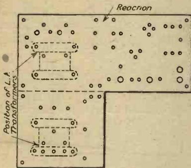
Fig. 2.—Drilling plan of the panel.
