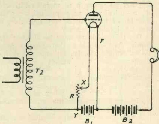
The circuit shown is a simple low frequency amplifier, and it will be seen that one end of the secondary  $T_2$  is connected to the grid and the other to the point  $Y$ . It will therefore be seen that the grid has normally a negative potential of 2.1 volts, and this is usually a
