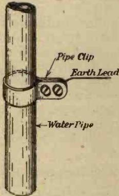
Fig. 1.—Clip on water pipe.
