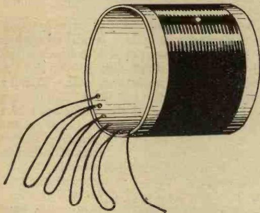
Fig. 3.—The complete inductance with tappings.
