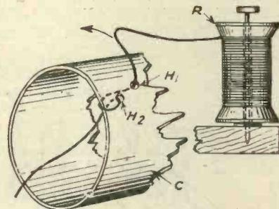
Fig. 3.—The first step in winding the coil.
