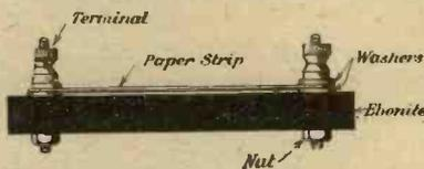
Fig. 1.—Elevation of grid leak.
