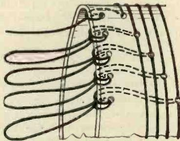
Fig. 9.—Appearance of finished tappings.
