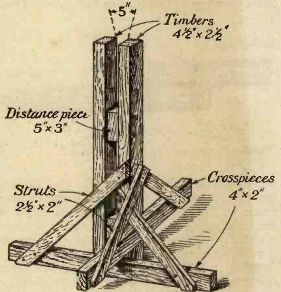
Fig. 4.—Details of the base structure.
