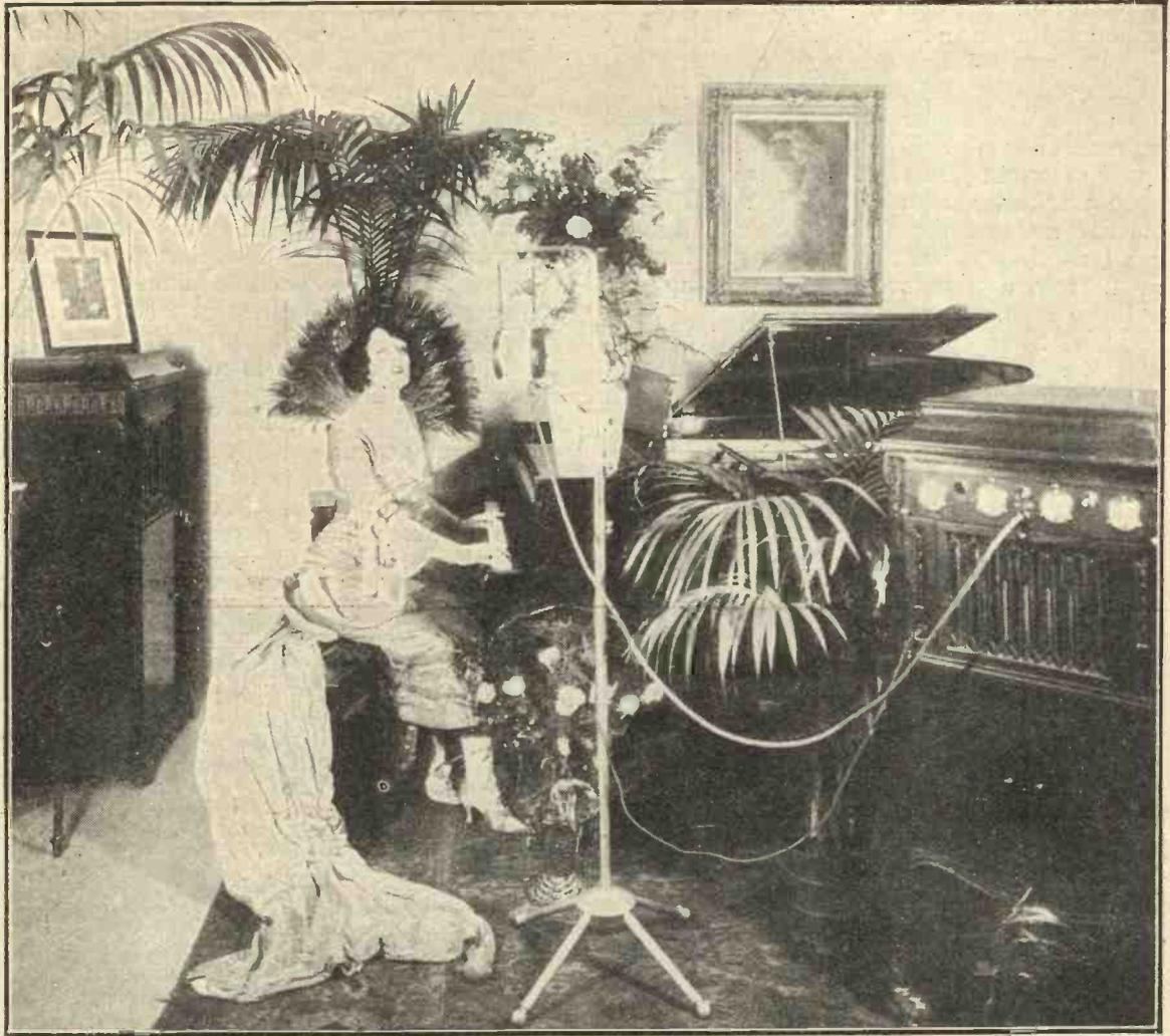
Fig. 3.—The Studio, with broadcasting in progress. Speech Amplifier on the right.
