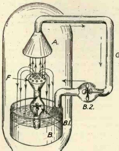
Fig. 12.—Analogy to show effect of a positive charge on the plate.
