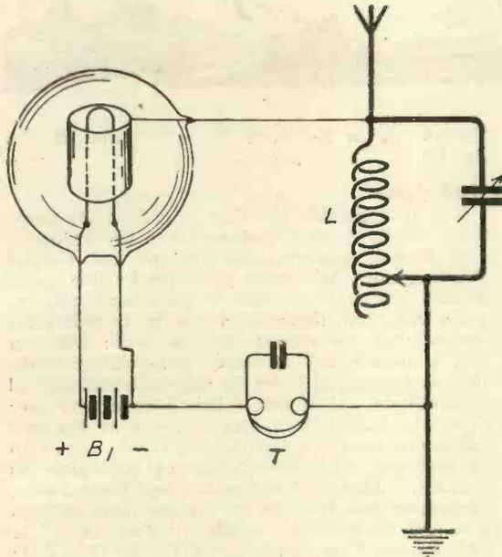
Fig. 14.—Circuit for use with 2-electrode valve.
