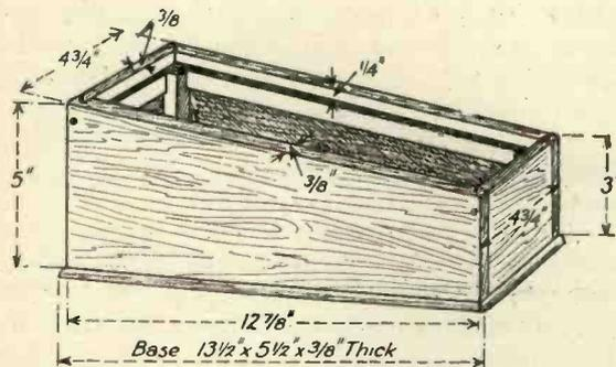
Fig. 3.—Details of the containing box.
