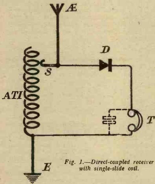
Fig. 1.—Direct-coupled receiver with single-slide coil.
