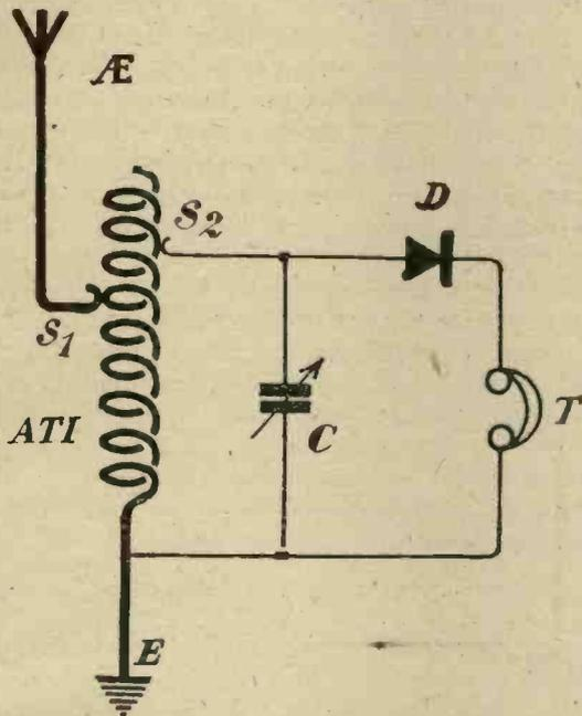
Fig. 3.—A two-circuit direct-coupled receiver.
