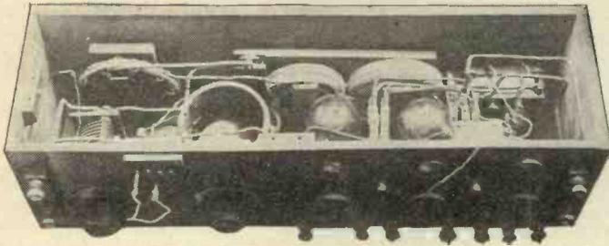
Fig. 1.—Internal arrangement of the receiver.
