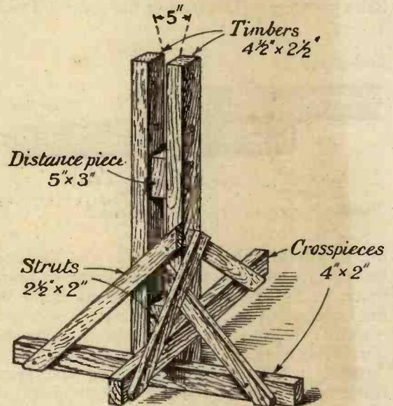
Fig. 4.—Details of the base structure.
