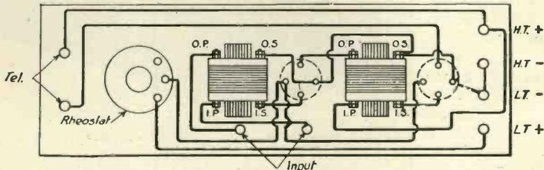
Fig. 6.—A "back-of-panel" wiring diagram.
