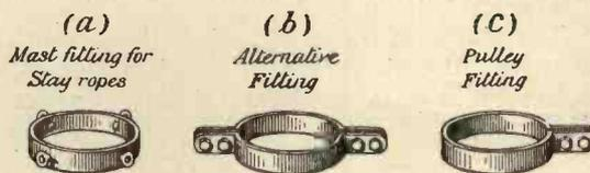
Fig. 7.—Iron fittings for the mast.
