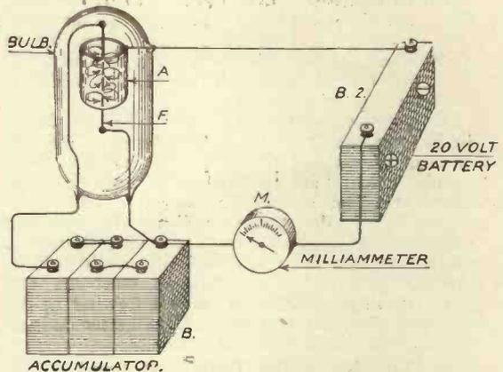
Fig. 11.—Negatively-charged plate repelling electrons.
