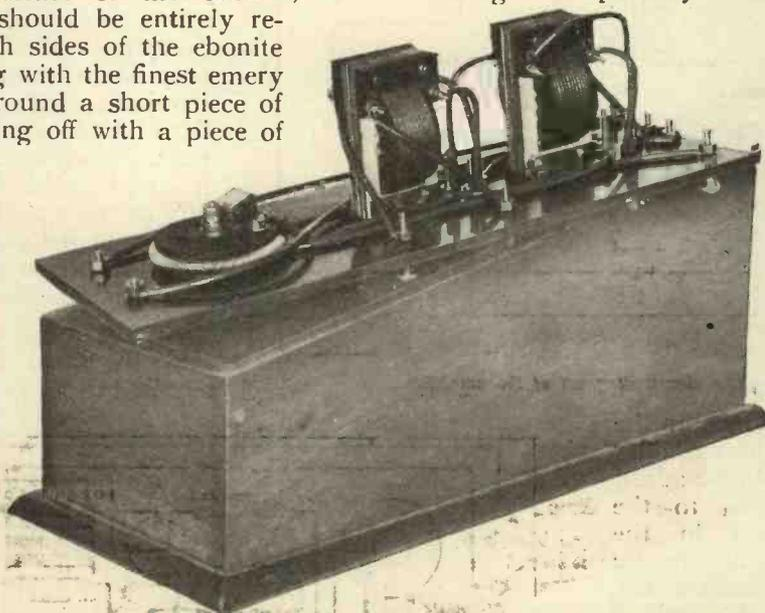
Fig. 2.—Back view of panel, showing components fitted in place and connected up.
