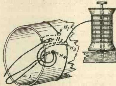
Fig. 6.—The first tapping completed.
