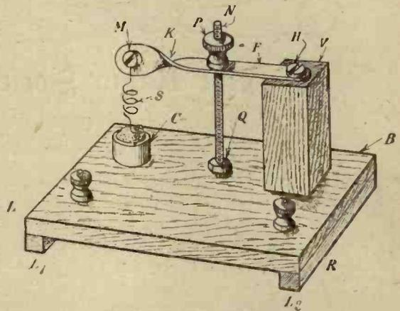
Fig. 8.—Showing the detector.
