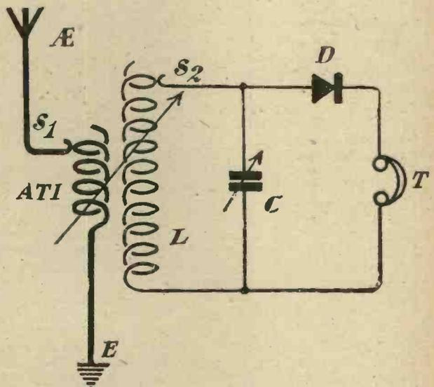
Fig. 4.—An inductively-coupled crystal receiver.
