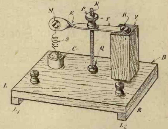
Fig. 8.—Showing the detector.
