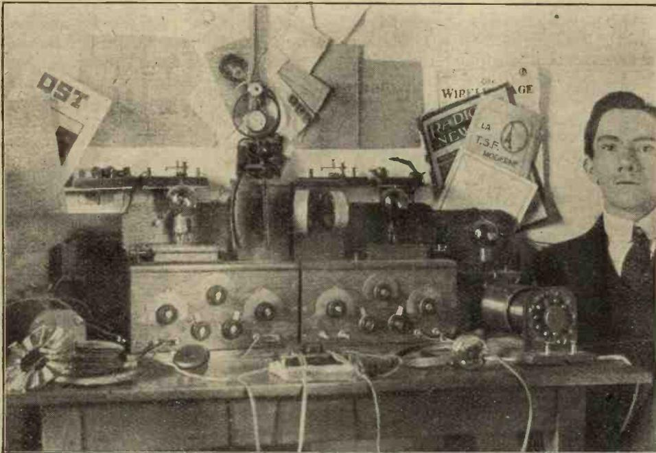
Fig. 2.—The complete installation; heterodyne on right.
