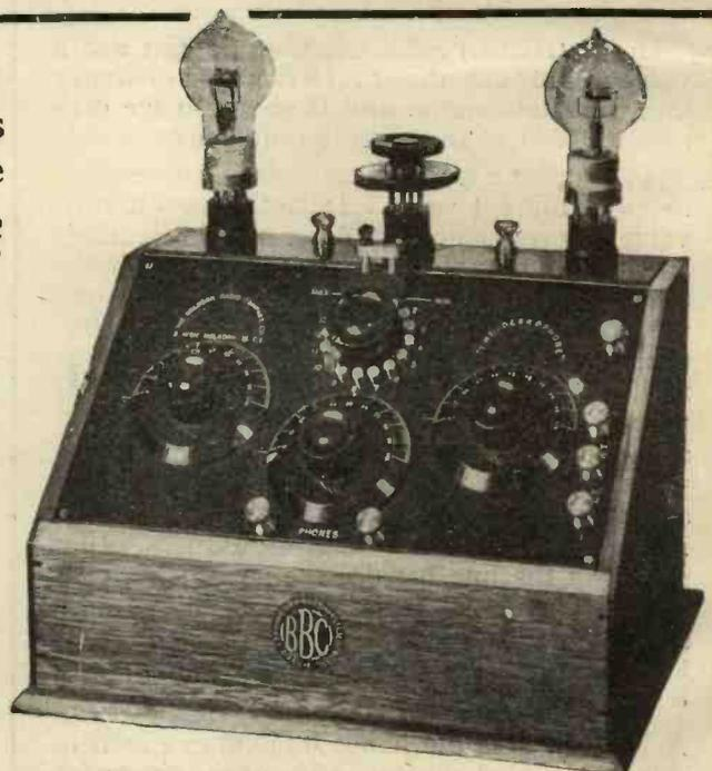
Two-Valve Set, Tuner, High Frequency Amplifier and Detector, complete with accessories, including Headphones, H.T. Battery, Accumulator, Aerial, Lead-in-Wire, and Insulators.
