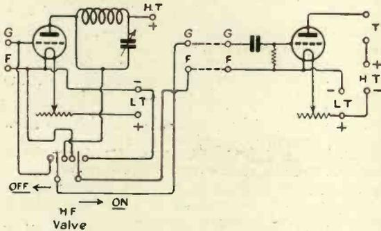
Showing the addition of a H.F. valve to the detector panel.
