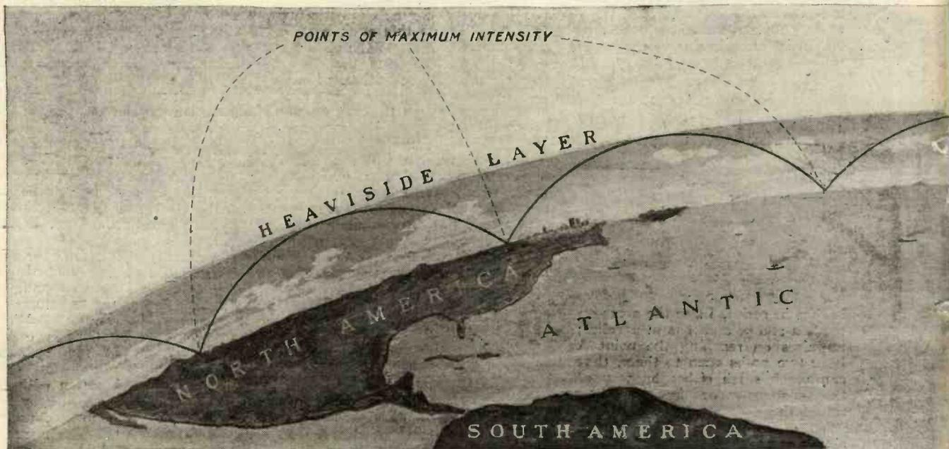
**O**UR knowledge of the way sound waves travel in the atmosphere may help towards an explanation of the many irregularities and occasional zones of silence observed in connection with the transmission of wireless signals.
