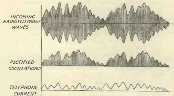
Fig. 15.—Graphic representation of the various currents in a broadcast receiver.
