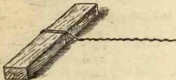
Fig. 2.—Timber with galvanised iron anchor-wire attached.
