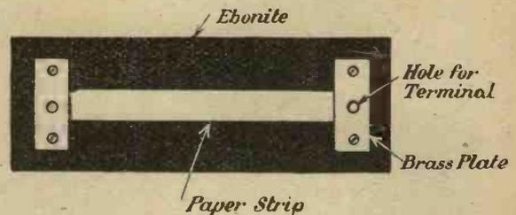
Fig. 2.—Plan of grid leak.
