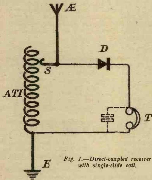
Fig. 1.—Direct-coupled receiver with single-slide coil.
