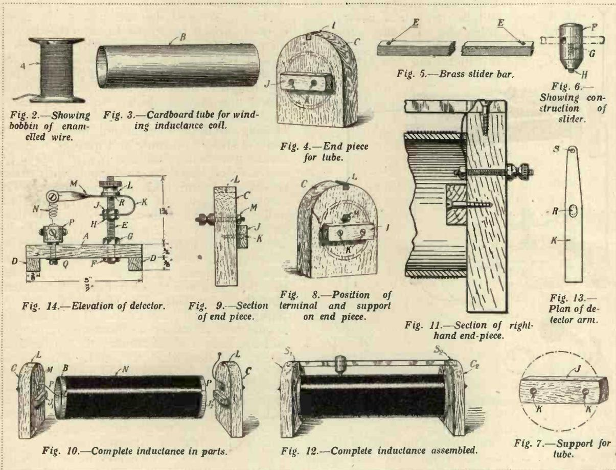
An ordinary piece of thin brass strip will do, and springiness may be imparted to it by hammering it. The strip K, before being bent, has the appearance shown in Fig. 13. The hole S, and the cut-out portion R, are arranged as shown. The bent strip is mounted on a piece of 2 B.A. brass studding marked E, and dimensioned as shown. This piece of studding is secured by means of two nuts F and G to the baseboard of the detector. The bent strip K is fixed to the vertical
