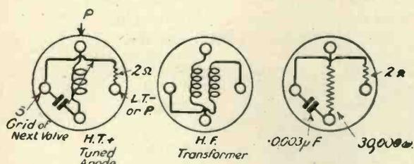
Fig. 9—Showing connections of inter-valve H.F. couplings.
