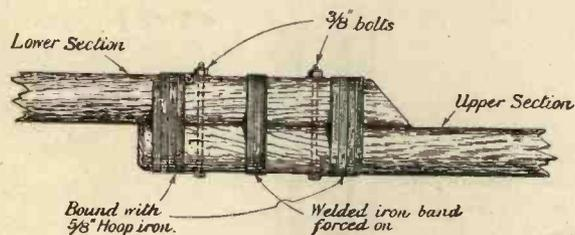
Fig. 5.—The joint in the mast.
