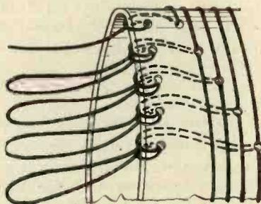
Fig. 9.—Appearance of finished tappings.
