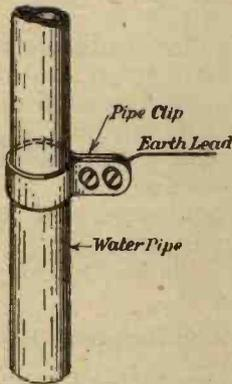
Fig. 1.—Clip on water pipe.
