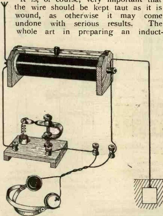
Fig. 1.—Pictorial diagram of connections.
