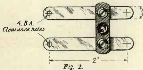
stud hole, care being taken to work the graphite well in at their ends so that contact may be as good as possible. Those on the right are made quite thin, those on the left about twice as broad. One thus obtains a great variety of resistances between the shortest thick line and the longest thin one.
