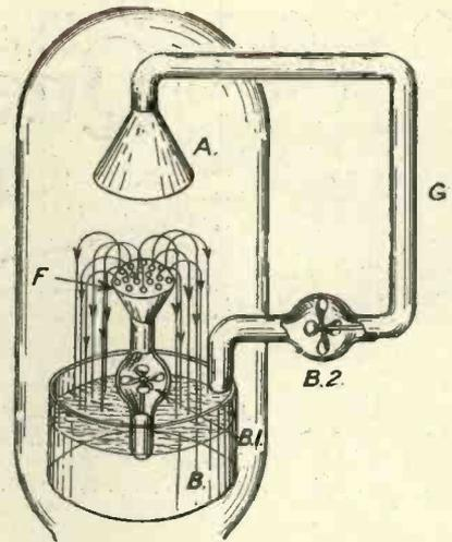
Fig. 13.—Water analogy corresponding to Fig. 11.
