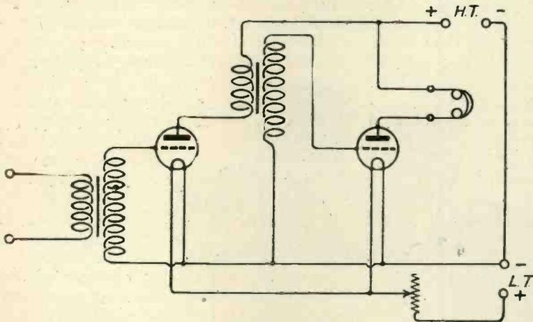
Fig. 5.—The circuit diagram of the amplifier.
