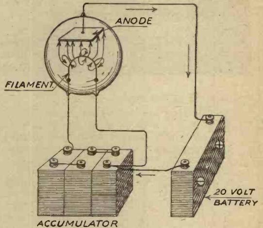
Fig. 9.—Electrons flowing to anode.
