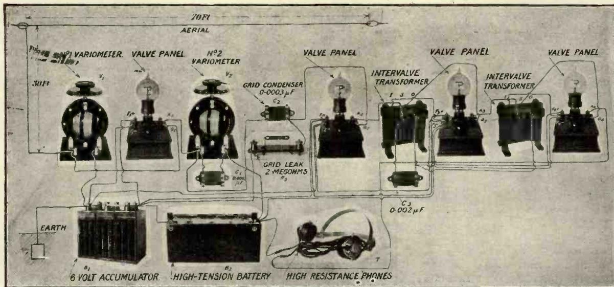
Fig. 6.—The four-valve receiver.
