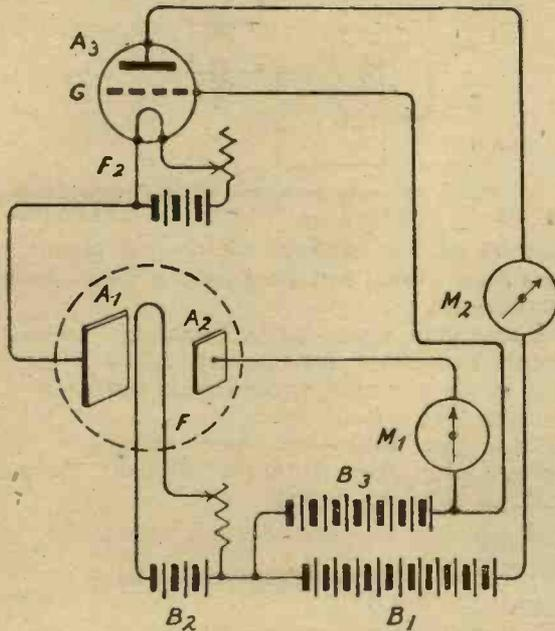
Fig. 5.—Static negative resistance device.
