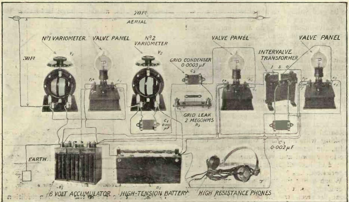
Fig. 4.—The complete 3-valve circuit.
