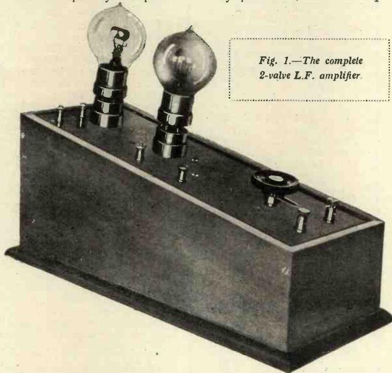
Fig. 1.—The complete 2-valve L.F. amplifier.
