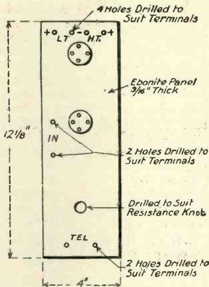
Fig. 4.—Drilling plan of the ebonite panel.
