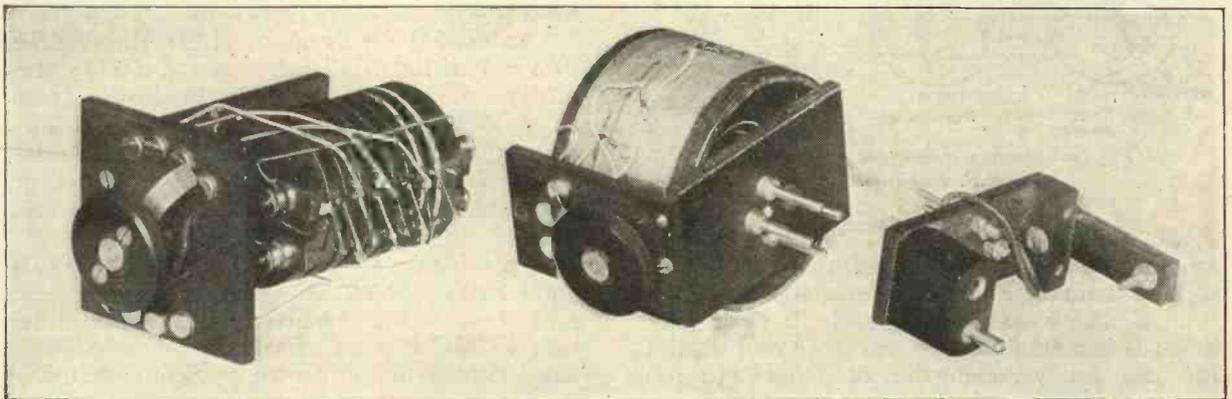
Fig. 8.—Photographs of different inter-valve H.F. couplings.
