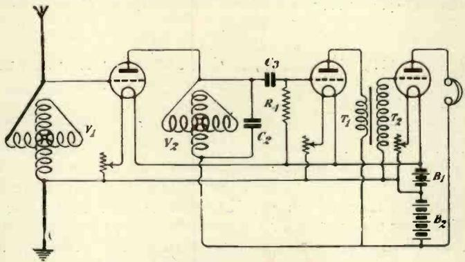
Fig. 5.—Circuit diagram of three-valve receiver.
