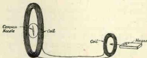
Fig. 10.—Compass needle placed at centre of coil, forming simple "galvanometer" or "ammeter." Inserting magnet in second coil causes momentary current in both coils and needle is deflected.
