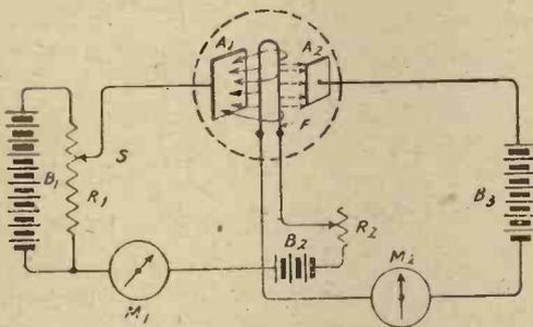
Fig. 2.—Obtaining characteristic curve.
