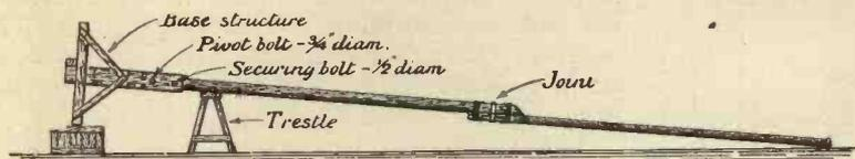
Fig. 6.—Fitting the base structure to the butt of the mast.
