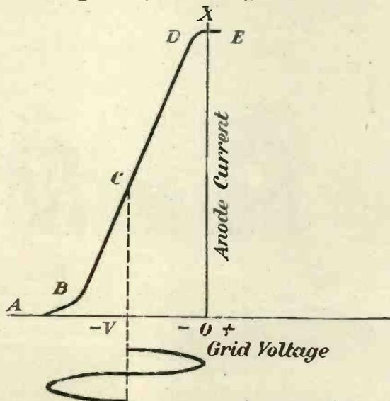
Fig. 1.—Characteristic curve of a power amplifier.
