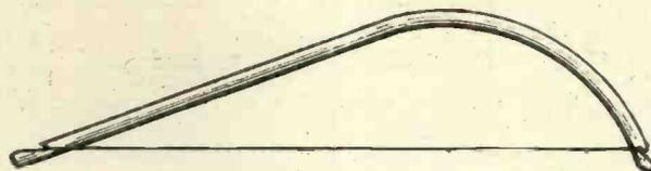
Fig. 8.—Drilling bow.
