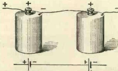
Fig. 8.—Pictorial representation (upper Fig.) and diagrammatic representation (lower Fig.) of two cells connected in series.
