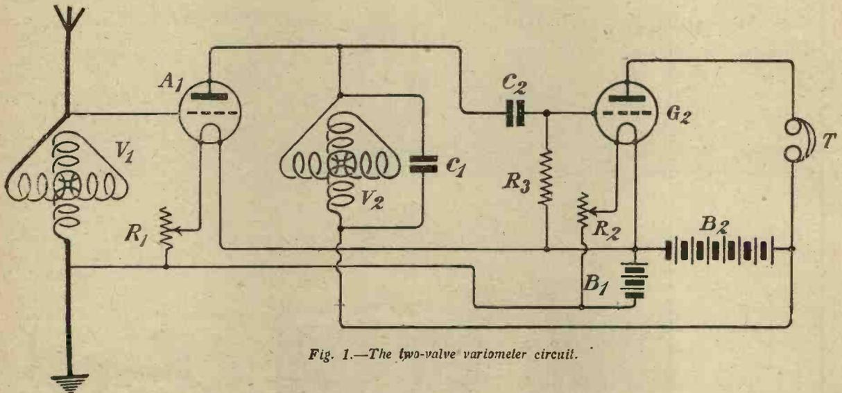
Fig. 1.—The two-valve variometer circuit.
