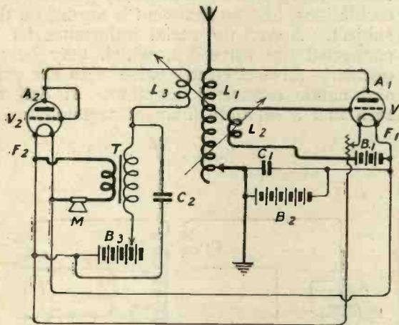
Fig. 5.—Circuit using a single accumulator.
