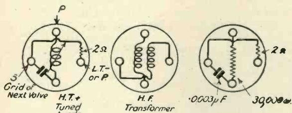
Fig. 9—Showing connections of inter-valve H.F. couplings.
