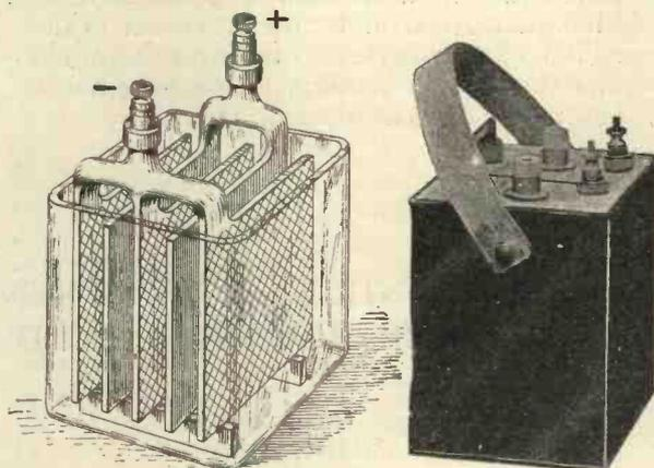
Fig. 1.—Showing arrangement of plates.
