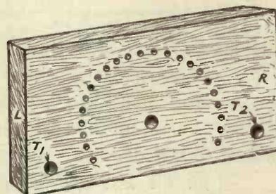
Fig. 15.—Holes drilled for selector switch and terminals.
