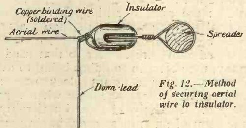
Fig. 12. — Method of securing aerial wire to insulator.
