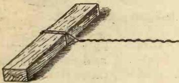
Fig. 2.—Timber with galvanised iron anchor-wire attached.
