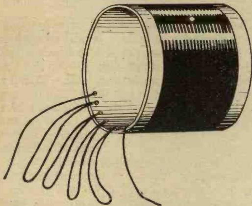
Fig. 3.—The complete inductance with tappings.
