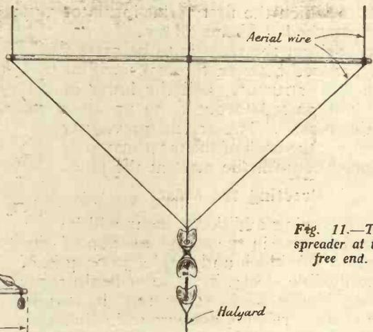
Fig. 11. — The spreader at the free end.
