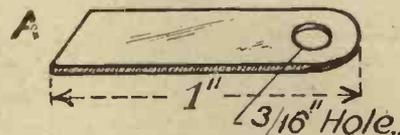
Fig. 7.—Connecting straps.
