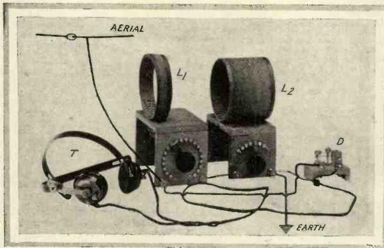
Fig. 1.—The complete receiver.
