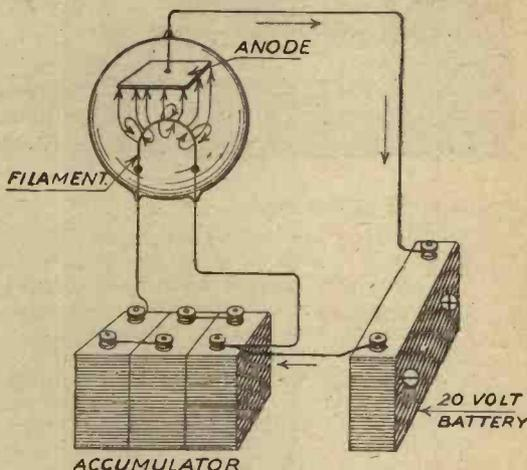
Fig. 9.—Electrons flowing to anode.
