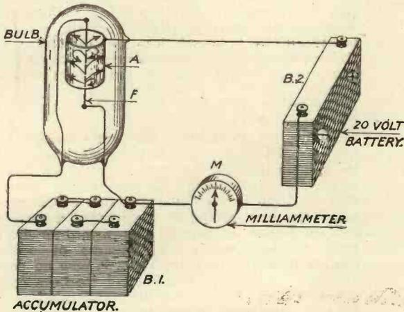
Fig. 10.—Positively-charged plate attracting electrons.
