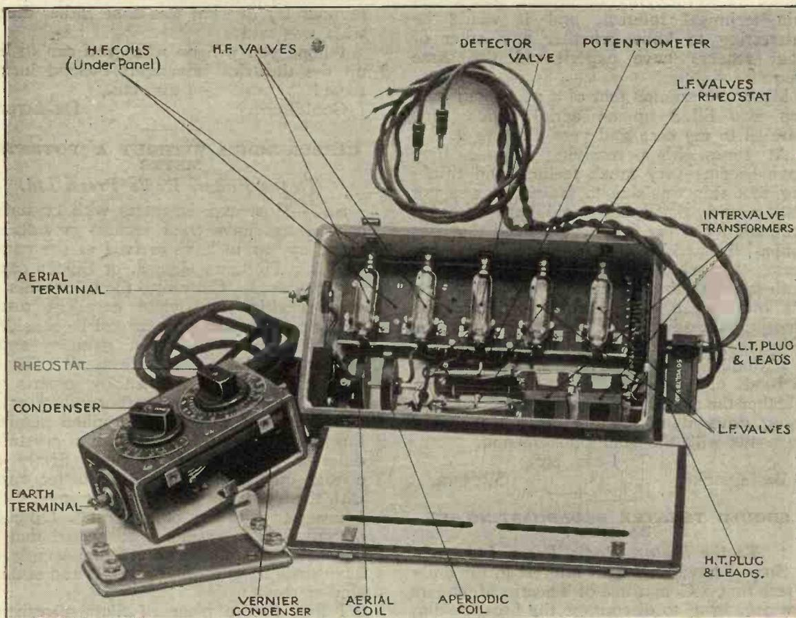
was intended for the reception of wireless telephony signals on a wavelength of 440 metres.
