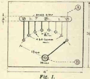
A piece of 1/4-inch ebonite measuring 3 1/2 inches by 4 is marked out and drilled as shown in the drawing. The central hole is for the spindle of a rotary switch arm, which can be bought complete with nut and bush for about 1s. from advertisers in this Journal. The circumferential holes, made with a 4 B.A. clearing drill, are for studs of the ordinary type, from eight to a dozen of which may be fitted.
