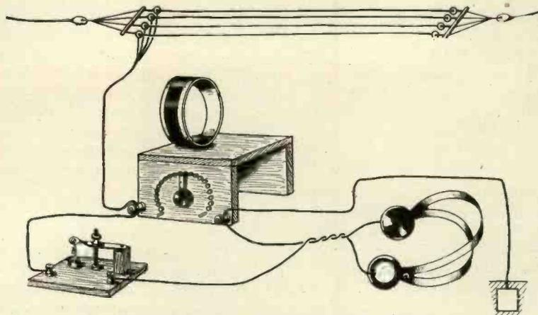
Fig. 4.—Arrangement for use on long aerials.
