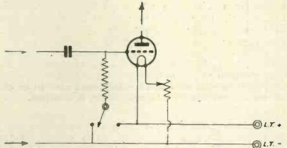
Your reaction coil appears to be much too large. The coupling with the anode coil should be just sufficient to raise signal strength to the maximum, and no more. Instead of connecting your gridleak as shown, one end of it should be attached to the positive filament leg. This will still further decrease any tendency to oscillate.
