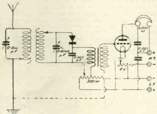
Coil L<sub>1</sub> might have 35 turns of No. 20 s.w.g. wire wound on a 3in. tube. Coil L<sub>2</sub> should have 50 turns of similar wire. The value of C<sub>1</sub> might be 0.0015 μF and C<sub>2</sub> 0.002 μF. High resistance telephones may, of course, be used in place of a telephone transformer, as shown above.
