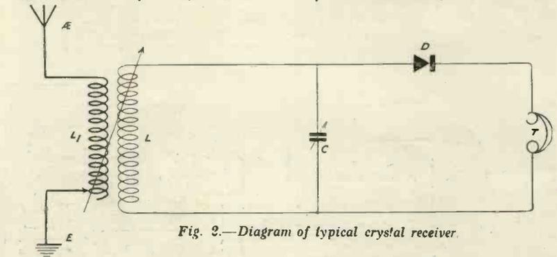
Fig. 2.—Diagram of typical crystal receiver.
