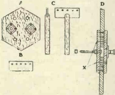
Fig. 3.—Parts required for constructing frame aerial.
