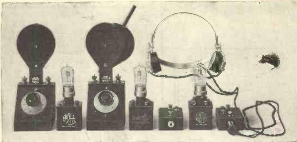
(1) Aerial Circuit. (2) H. F. Valve. (3) Tuned Anode and Reaction Unit. (4) Rectifier Unit. (5) D. F. Jack. (6) L. F. Unit. (7) S. F. Jack and Telephone Plug.
