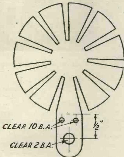
Fig. 4.—Former for the moving coils.
