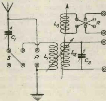
Fig. 6.—Circuit diagram of the tuner.
