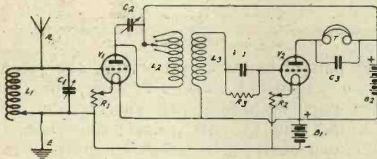
Fig. 3.—A tuned transformer coupling.
