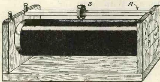
Fig. 1.—A "single slide" tuning inductance.
