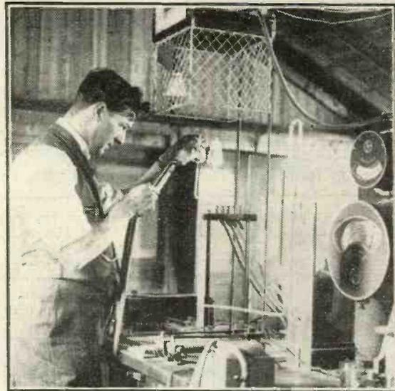
*The final process in making a valve. The air in the bulb is exhausted through a glass tube. A blowpipe is finally used to seal off the tube at the pip.*
