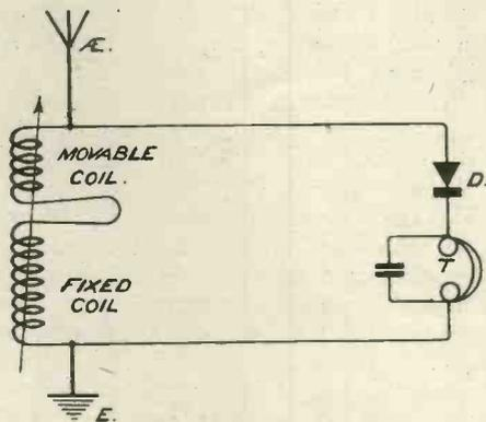
Fig. 15.—Circuit diagram of receiver with variometer.
