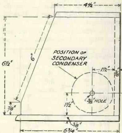
Fig. 3.—Dimensions of side of containing box
