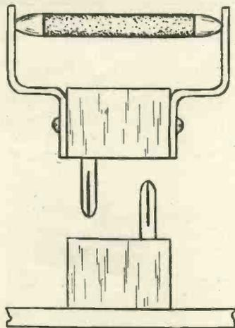
Fig. 4.—Method of mounting anode resistances.
