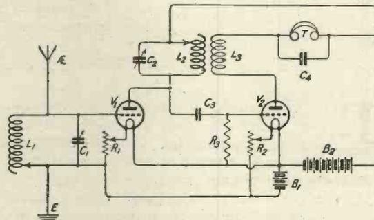
Fig. 4.—A circuit employing the approved type of reaction.
