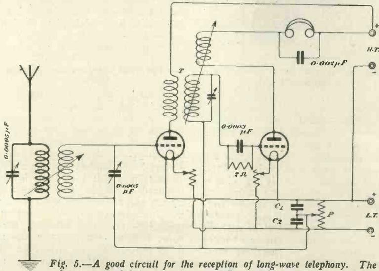
Fig. 5.—A good circuit for the reception of long-wave telephony. The valves are coupled by an air-core H.F. transformer,  $T$ , and the fine adjustment of reaction is provided by the potentiometer  $P$ .
