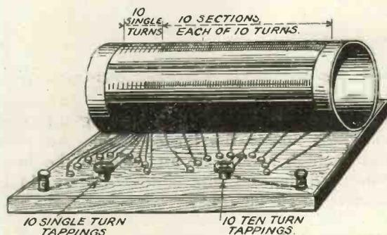
Fig. 8.—A tuning inductance with multiple and sub-multiple tapplings.
