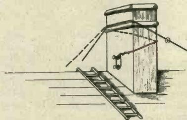
Fig. 18.—Using chimney ledge as anchorage for aerial.
