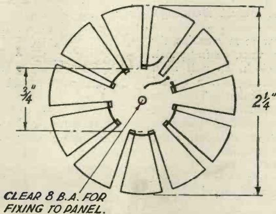
Fig. 3.—Former for the fixed basket coil.
