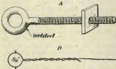
Fig. 15.—The eye-bolt and a wire loop.
