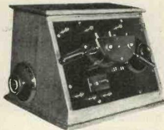
Fig. 1a.—A left-hand view showing secondary condenser.
