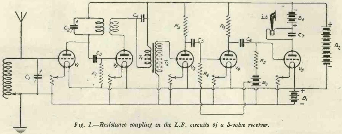
Fig. 1.—Resistance coupling in the L.F. circuits of a 5-valve receiver.
