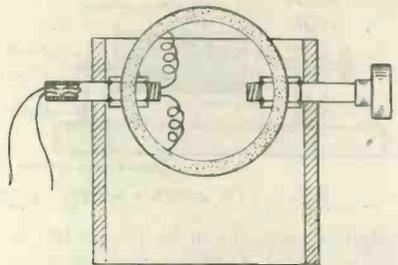
Fig. 6.—Suggestion for inner coil connections of a vario-coupler.
