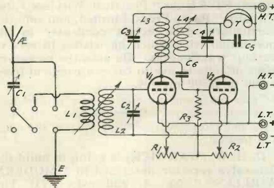
We give herewith a suitable circuit diagram for your purpose, showing how a two-valve receiver may be arranged in the most efficient manner. The values
