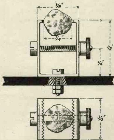
Fig. 1.—Elevation and plan of crystal holder.
