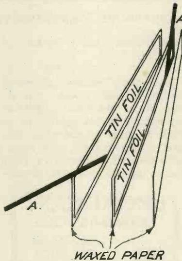
Fig. 9.—The assembly of the foils.
