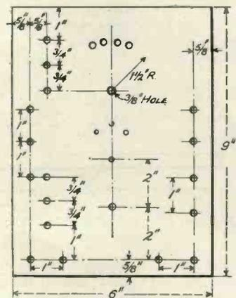
Fig. 5.—Dimensions of panel.
