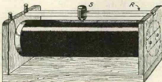
Fig. 1.—A "single slide" tuning inductance.
