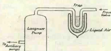
Fig. 5.—Mercury trap to prevent mercury vapour from reaching the exhausted vessel: used for production of very high vacua.
