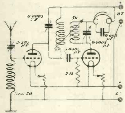
Fig. 2.—Method of controlling reaction by a variable condenser shunted across the reaction coil. Numbers indicate suitable sizes of Igranite coils for broadcast reception.
