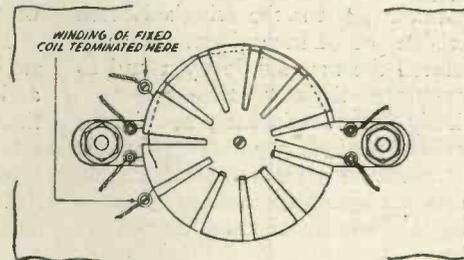
Fig. 5.—Assembly of the reaction coil and variometer.
