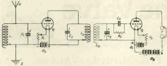
Fig. 2.—Tuned transformer coupling.
