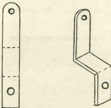
Fig. 5.—Showing how to bend the clips.
