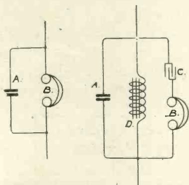
Fig. 7.—Showing the shunt device.
