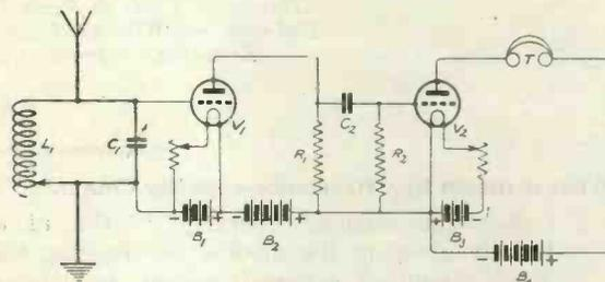
Fig. 3.—A theoretical circuit explaining resistance capacity coupling.
