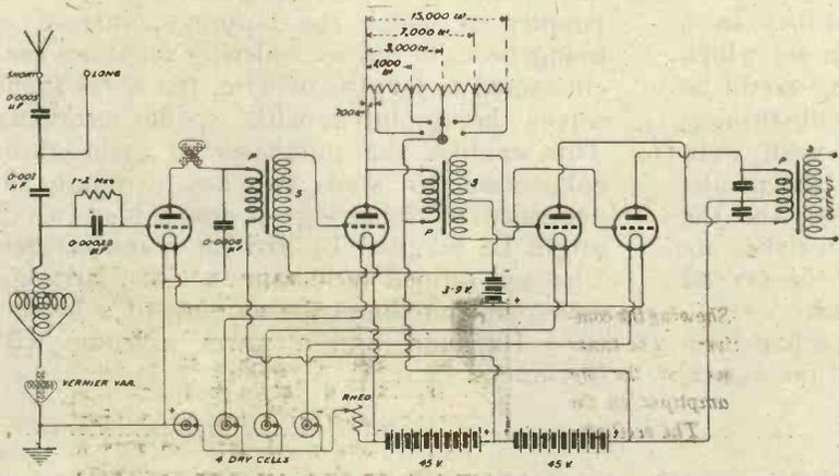
*On the left, a circuit employing the “pull-push” method of amplification. The filament circuits are arranged for dull-emitter valves. The resistance across the transformer primary is for the purpose of adjusting the output to the desired volume.*
