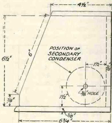
Fig. 3.—Dimensions of side of containing box
