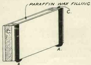
Fig. 10.—Finished condenser.
