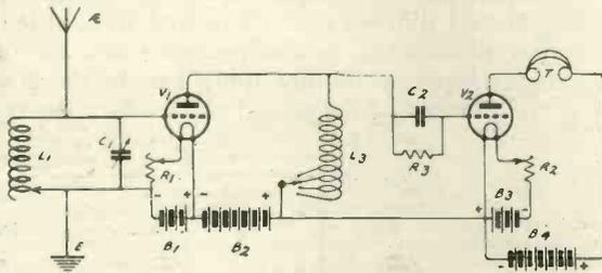
Fig. 1.—Theoretical circuit illustrating reactance-capacity coupling.
