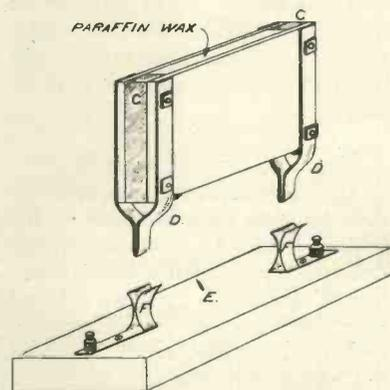
Fig. 12.—An interchangeable mounting for the condensers.
