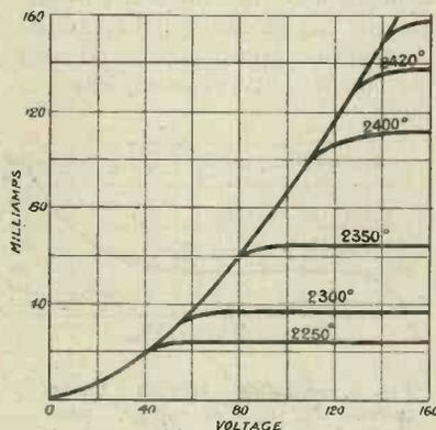
Fig. 1.—Showing maximum emission (saturation current) for various temperatures of filament (Langmuir).
