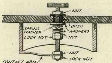
Fig. 14.—Sectional view of potentiometer.
