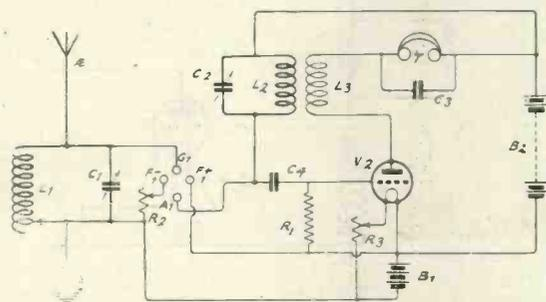
Fig. 1.—The ST34 circuit with the first valve removed.
