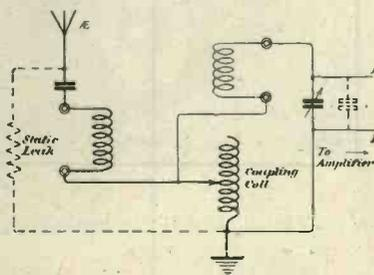
Fig. 3.—Diagram of the tuner showing one of the inductances in each circuit.
