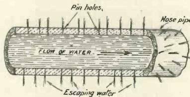
Fig. 5.—Water escaping through pinholes in hose-pipe, illustrating, in a rough way, emission of electrons from hot wire.
