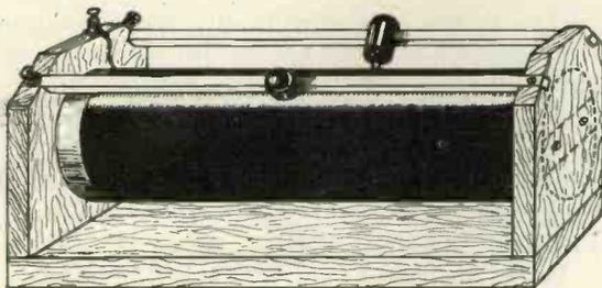
Fig. 6.—A simple but effective tuner employing two sliders.
