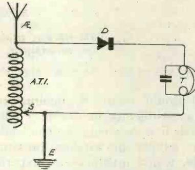
Fig. 5.—A simple crystal receiver circuit.
