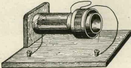
Fig. 14.—An easily constructed but efficient variometer.
