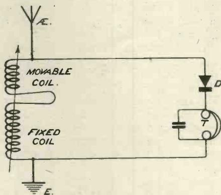
Fig. 15.—Circuit diagram of receiver with variometer.
