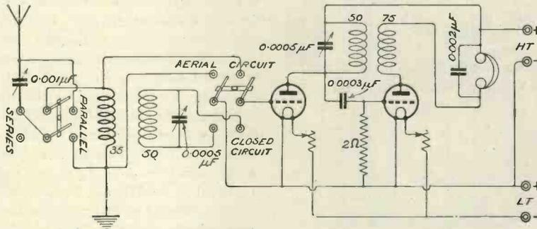
Fig. 1.—The theoretical circuit, showing switching.
