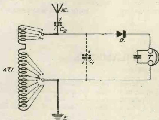
Fig. 9.—The circuit arrangement when a tapped inductance is used.
