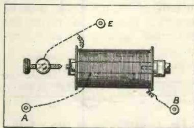
Fig. 2.—Showing connections of buzzer.
