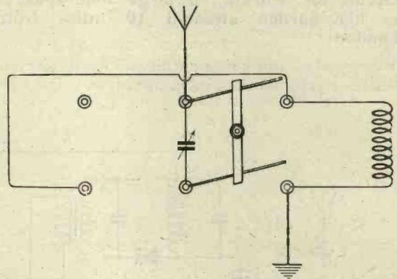
J. G. (WATFORD) asks for the correct connections of a series-parallel switch. See the accompanying diagram.
