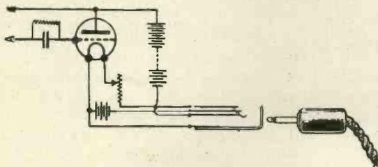
Fig. 4.—A "single filament" jack.
