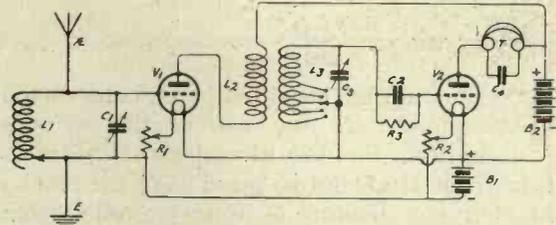
Fig. 4.—Transformer with a tuned secondary (compare with Fig. 3).
