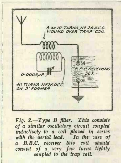
Fig. 2.—Type B filter. This consists of a similar oscillatory circuit coupled inductively to a coil placed in series with the aerial lead. In the case of a B.B.C. receiver this coil should consist of a very few turns tightly coupled to the trap coil.
