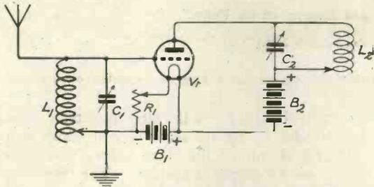
Fig. 3.—A simple amplifier circuit without reaction.
