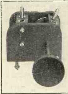
Fig. 1.—A coil holder giving fine adjustment.
