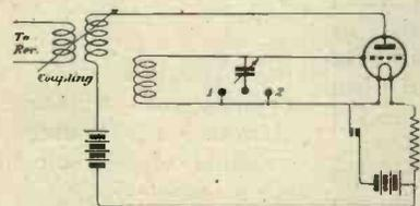
Fig. 1.—Circuit of the local oscillator.
