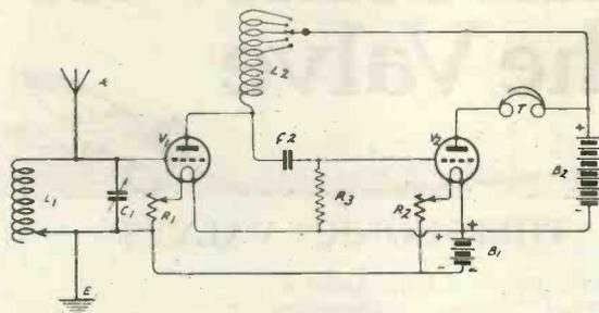
Fig. 2.—A practical application of reactance-capacity coupling.
