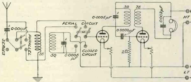
Fig. 1.—The theoretical circuit, showing switching.
