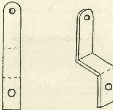
Fig. 5.—Showing how to bend the clips.
