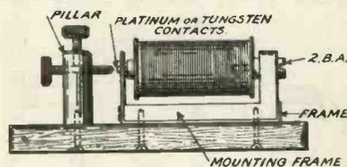
Fig. 1.—The complete buzzer.
