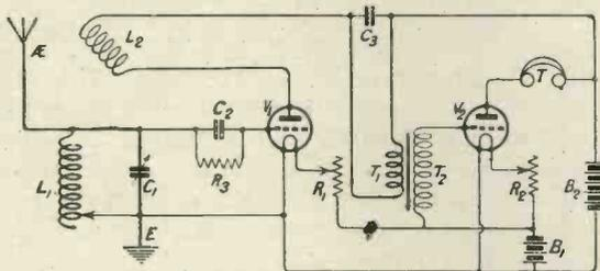
Fig. 3.—The addition of low-frequency amplification to the circuit of fig. 2.
