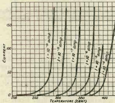
Fig. 2.—Showing the rapid increase in the emission from sodium with rise of temperature (Richardson).
