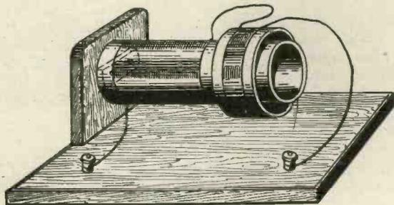
Fig. 14.—An easily constructed but efficient variometer.
