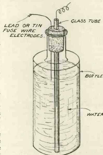
Fig. 8.—The completed resistance.
