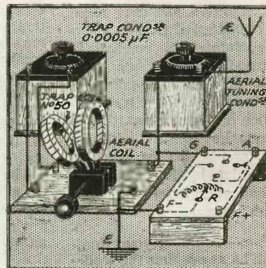
(Above) Type C filter inductively coupled in shunt with the aerial lead. This is a very useful arrangement, and is very widely known. American writers consider this the best method for reducing interference at amateur stations working the immediate
