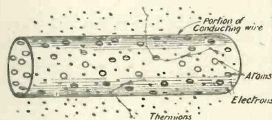
Fig. 4.—Electrons forming heating-current collide with atoms of filament, and raise temperature, some electrons being ejected (thermions).
