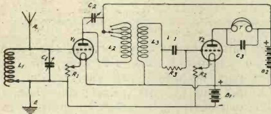
Fig. 3.—A tuned transformer coupling.
