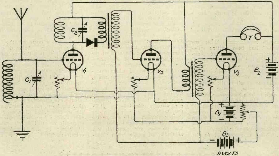
Fig. 1.—A method of obtaining exact adjustment of grid potential.
