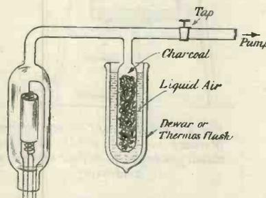
Fig. 3.—Illustrating the method of employing charcoal cooled by liquid air, for absorbing the residual gas which cannot be removed by pump.
