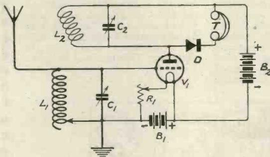
Fig. 1.—A simple valve-crystal receiver with reaction.
