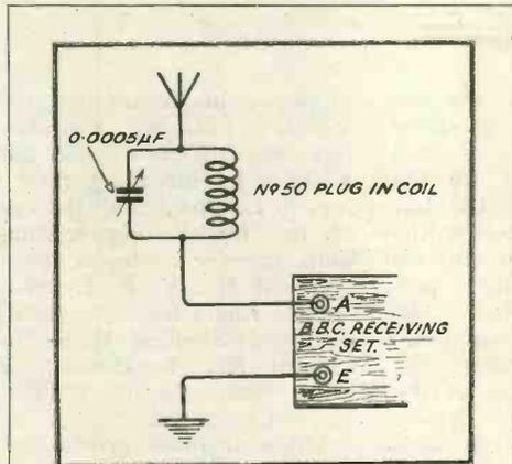
Fig. 1.—Type A wave-filter—a simple oscillatory circuit connected in series with the aerial lead. When this circuit is tuned to the interfering wave, it will act as a trap for this wave and will very largely reduce the jamming.
