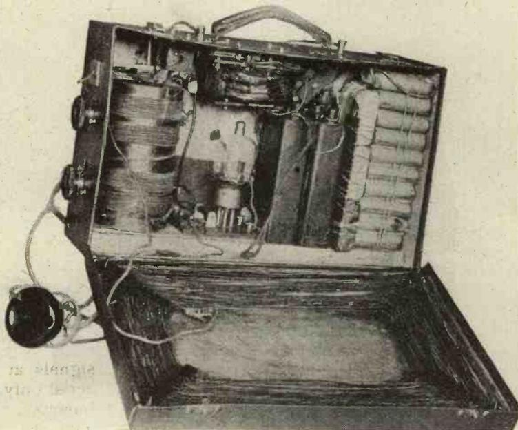
the single-valve Armstrong or flivver circuit, in its later stabilised version, offers great attractions: the modest demands on the low-tension supply of the one valve, the excellent results obtainable on a tiny enclosed aerial, and the inherent stability and simplicity of tuning when properly designed and adjusted, all point to the Armstrong as an ideal portable short-wave receiver, and now that the last drawback of the circuit—the continuous whistle of the quenching oscillation—has
