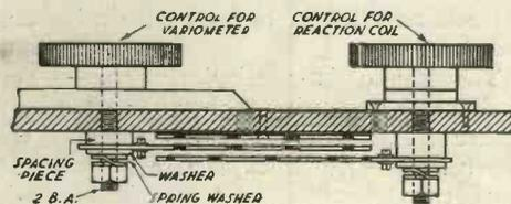
Fig. 6.—Section of variometer and reaction coil.
