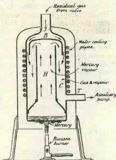
Fig. 4.—Principle of Langmuir pump. Mercury vapour "wind" blows residual gas before it, vapour afterwards condensing.
