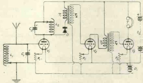
Fig. 2.—A three-valve tuned anode receiver employing a crystal detector.
