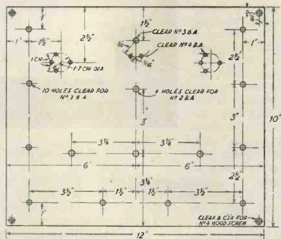
Fig. 2.—Plan of the panel.
