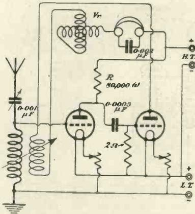
Fig. 4.—Another good circuit for long-wave telephony. Interval coupling is provided by resistance  $R$ , while the variometer  $V_r$  controls the reaction.
