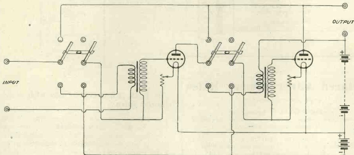
**WATMEL VARIABLE GRID LEAK** (Patent applied for.)
