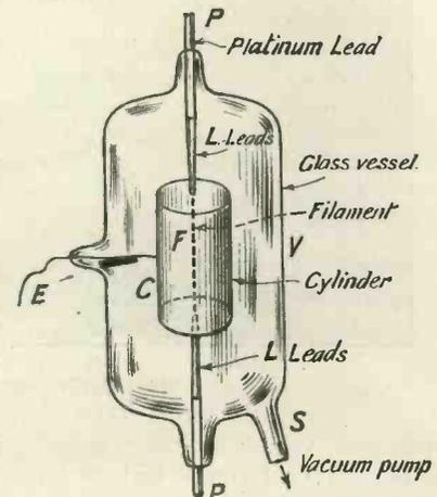
Fig. 2.—Simple arrangement for studying emission from a wire under various conditions.
