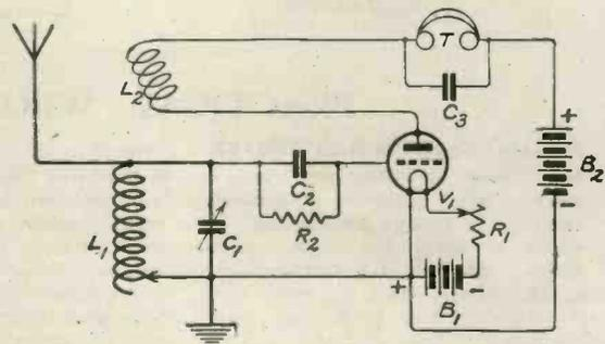
Fig. 2.—A single valve reaction circuit.
