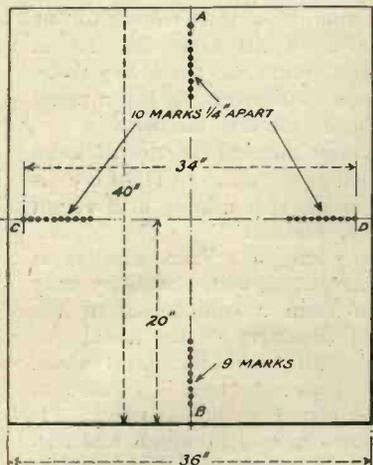
Fig. 1.—Dimensions of the holland foundation.
