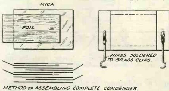
Fig. 4.—The arrangement of parts for making a telephone condenser.
