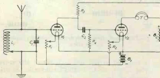
Fig. 4.—A practical circuit illustrating resistance capacity coupling.
