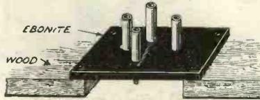
Fig. 4.—Arrangement of valve legs on wooden panels.
