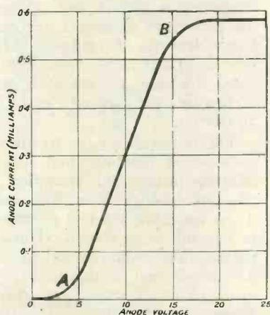
Fig. 1.—Characteristic curve of 2-electrode valve (or triode with grid and anode connected together).
