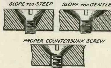
Fig. 7.—Illustrating correct and incorrect countersinks.
