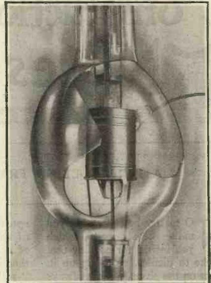
A broken Marconi transmitting valve, showing the arrangement of the electrodes.
