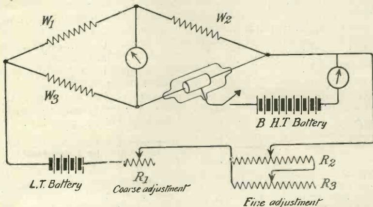
Fig. 3.—Arrangement for heating filament and Wheatstone bridge for accurate determination of temperature (by resistance). Emission current measured on galvanometer.
