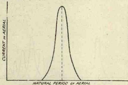
Fig. 1.—Showing the effect of aerial resistance on an imposed H.F. current.
