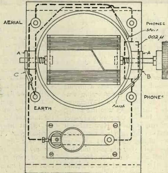
Fig. 1.—Underside of baseboard showing wiring.
