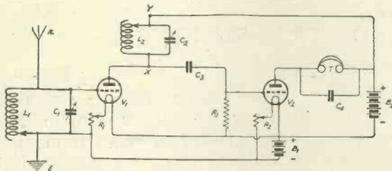
Fig. 1.—"Tuned anode" H.F. coupling.
