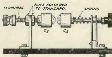
Fig. 6.—The converted Perikon detector.
