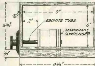
Fig. 4.—Arrangement for fitting the secondary condenser.
