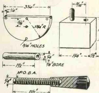
Fig. 5.—Components for coil mounting.
