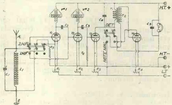
The arrangement you indicate should ensure satisfactory results, but the condensers coupling the anode coils are much too large. These should have a value not greater than 0.00025  $\mu$ F, and be arranged as shown in diagram above.
