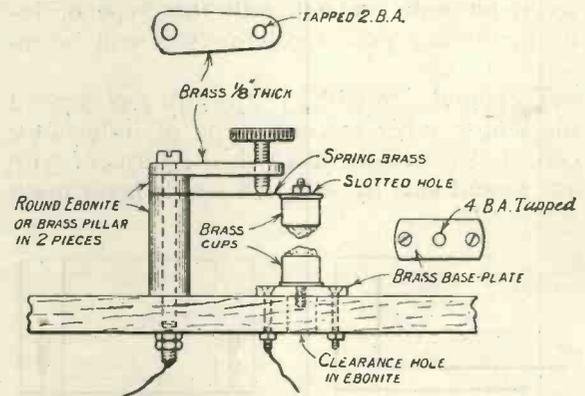
Fig. 3.—A "combination" detector employing two crystals; sometimes called a "perikon" detector.
