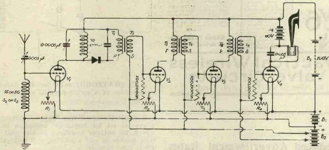
for Igranic and Burndept coils are shown in the figure, together with condenser, battery, and resistance values. The battery  $B_3$  may be variable up to 9 volts.
