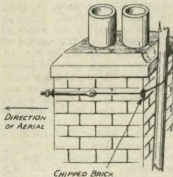
Fig. 16.—Method of fixing pole.
