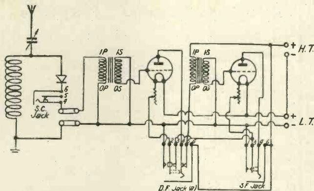
Fig. 5.—A "double filament" jack
