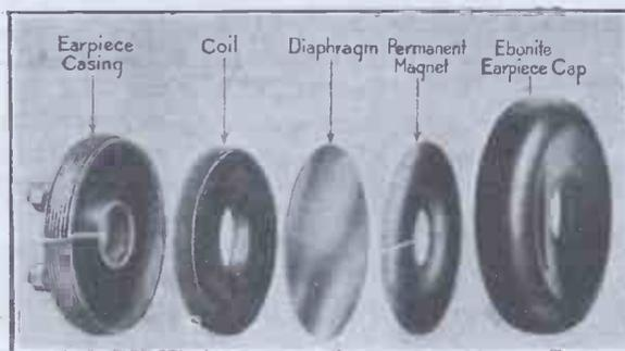
Photograph showing component parts of the Dynaphone Earpiece in their order of assembly.
