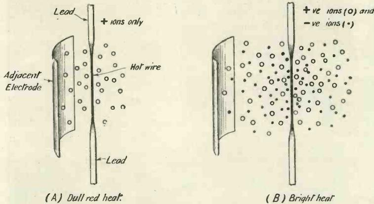
Fig. 1.—A fresh wire, before prolonged heating has driven out all traces of gas and impurities: (A) at dull-red heat only +ve ions emitted, (B) at bright heat +ve and -ve ions emitted.
