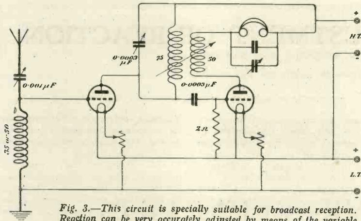
Fig. 3.—This circuit is specially suitable for broadcast reception. Reaction can be very accurately adjusted by means of the variable telephone condenser.
