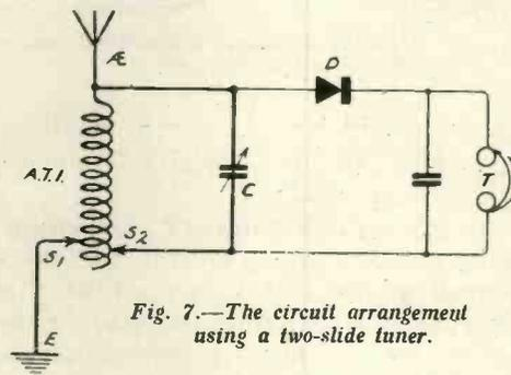
Fig. 7.—The circuit arrangement using a two-slide tuner.
