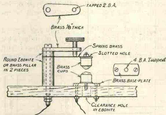
Fig. 3.—A "combination" detector employing two crystals; sometimes called a "perikon" detector.
