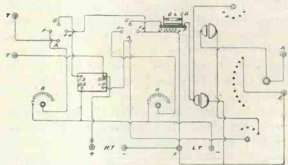
Fig. 6.—A pictorial arrangement showing the actual connections to the various components as seen from the underside of the panel.
