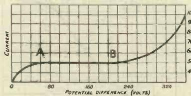
Fig. 3.—Relation between anode-current and applied voltage, when filament is cold and current is carried by ionisation of residual gas only.
