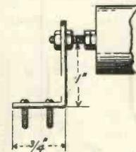
Fig. 9.—Clip for mounting the transformer.
