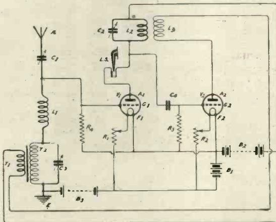
Fig. 1.—The ST75 circuit showing the position of the extra resistance  $R_1$ .
