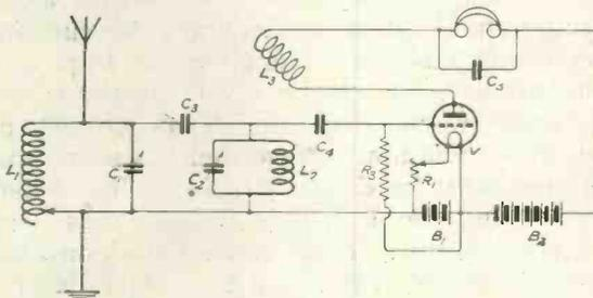
Fig. 3.—The final arrangement of the circuit.
