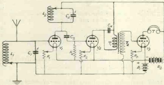
Fig. 1.—A three-valve tuned anode receiving circuit.
