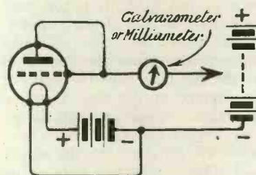
Fig. 2.—Simple method of determining characteristic curve of valve
