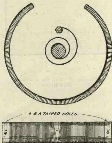
Fig. 13.—Illustrating arrangement of the resistance element.
