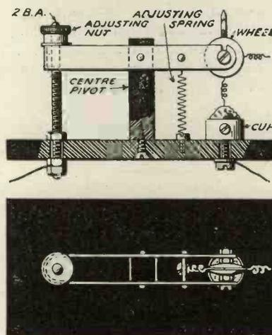
Fig. 8.—A detector suitable for use with the rotating wheel.
