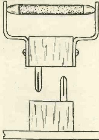
Fig. 4.—Method of mounting anode resistances.
