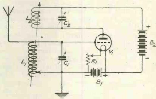
Fig. 4.—Showing how reaction is obtained by coupling anode and grid coils.
