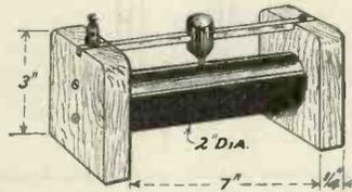
Fig. 2.—The finished potentiometer.
