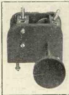
Fig. 1.—A coil holder giving fine adjustment.
