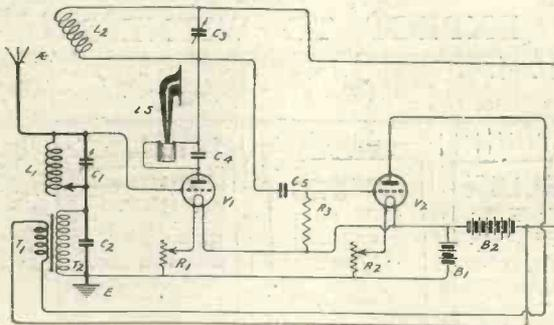
Fig. 1.—The ST150 Circuit.
