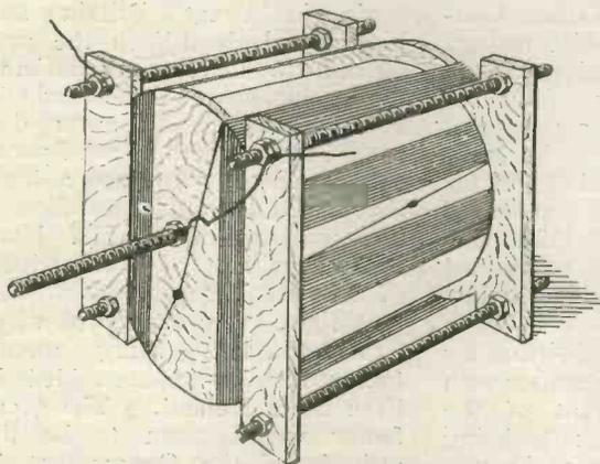
Fig. 1.—The completed variometer.
