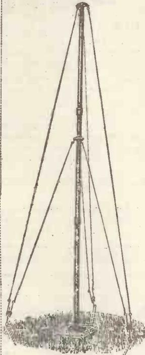
This is a wooden Mast light and strong, in three sections of 2 1/2 in. diameter fir with steel sockets and screws for fixing and all finished grey lead paint, approximately 30 ft. in height, with iron ground socket, six galvanized strand wire guys. Complete with hooks, three double straining screws, three iron ground stakes, cord cleat and galvanized pulley.
