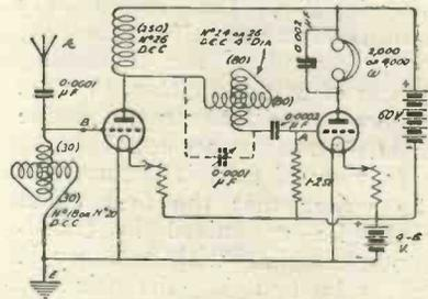
Fig. 4.—A practicable non-oscillating broadcast receiver.
