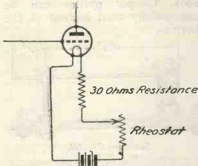
Fig. 5.—Illustrating position of the extra resistance.
