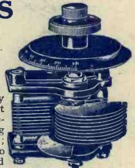
With Vernier Adjustment (as illustrated). The auxiliary knob controls the Vernier vane.
