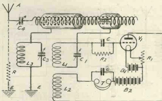
Fig. 2.—Receiving circuit with rejector between guard ring and earth.
