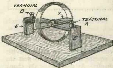
Fig. 5—The Galvonometer.
