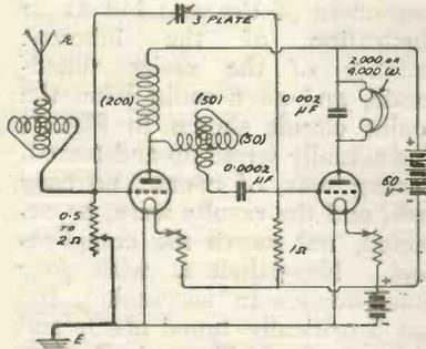
Fig. 1.—A complete short-wave receiver, 150/220 metres.
