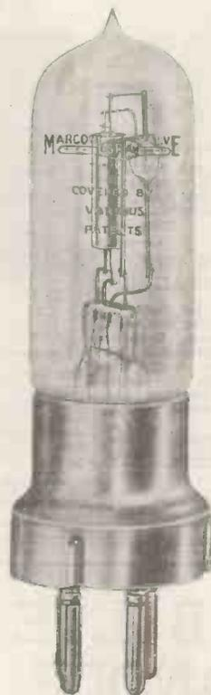
Three ordinary dry cells in series will run one of these valves for 800 hours. The current consumption is 0.06 amp. Filament voltage 2.4 to 3.0. Plate voltage 30/80.
