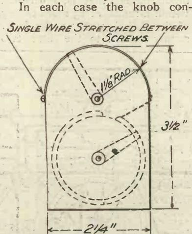
Fig. 3.—An alternative method of mounting the vernier attachment.
