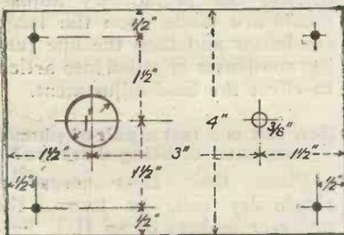
Fig. 24.—Drilling dimensions of the panel.
