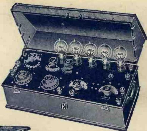
Five valve set in case, with cover not interfering with valves or leads. Wavelength range 300-4,000 metres. PRICE £31:5:0
