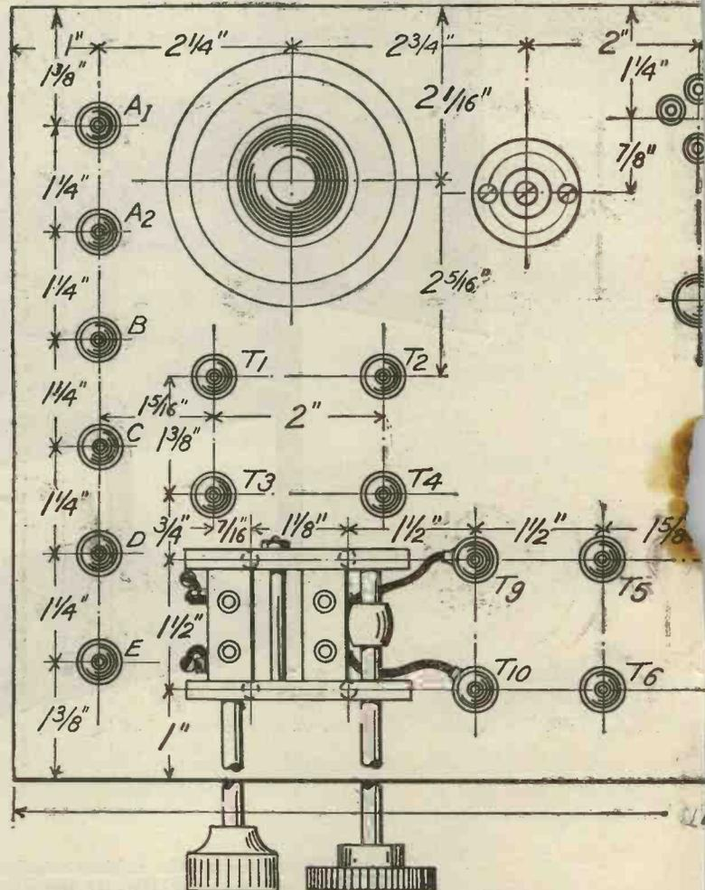
Fig. 3.—A half-size drawing, showing the layout of the parts on the panel.
