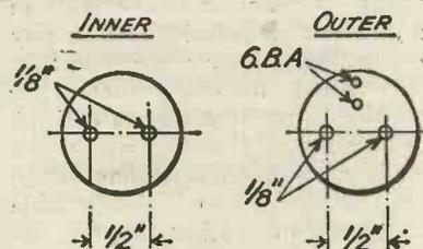
Fig. 1.—Construction of outer and inner tube ends.
