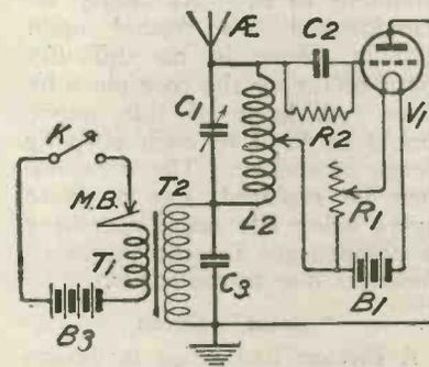
Fig. 19.—A transmitter circuit in which an induction coil is used to supply H.T. voltage for the plate of the oscillating valve.
