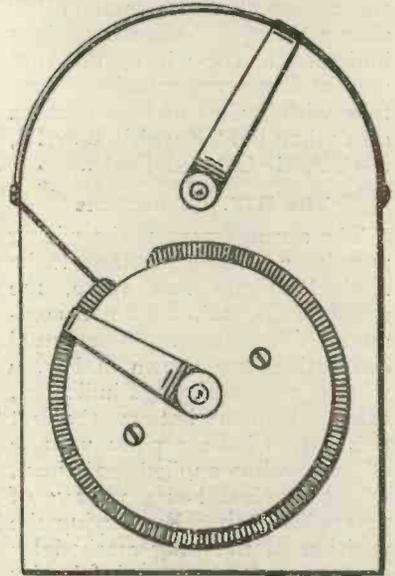
Fig. 4.—Showing how a vernier attachment may be added to a rheostat of the ordinary type.
