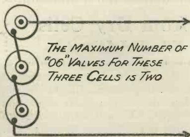
Fig. 3.—Arrangement of dry cells for two ".06" valves.
