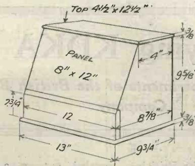
Fig. 8.—Constructional details of the containing box.
