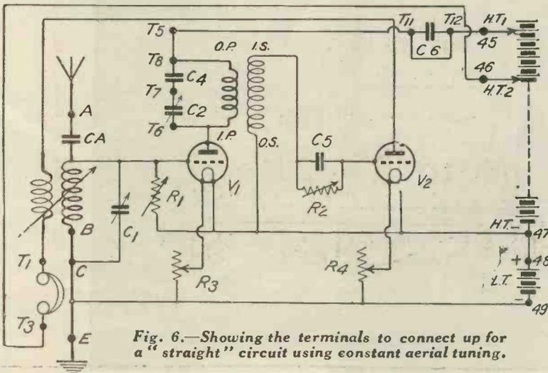
Fig. 6.—Showing the terminals to connect up for a "straight" circuit using constant aerial tuning.
