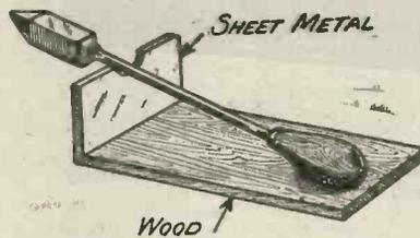
Fig. 2.—A convenient form of iron rest.
