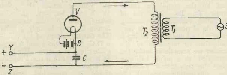
Fig. 20—Illustrating the theory of valve rectification
