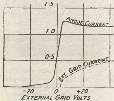
Fig. 1.—Characteristic curve of a double-grid valve.
