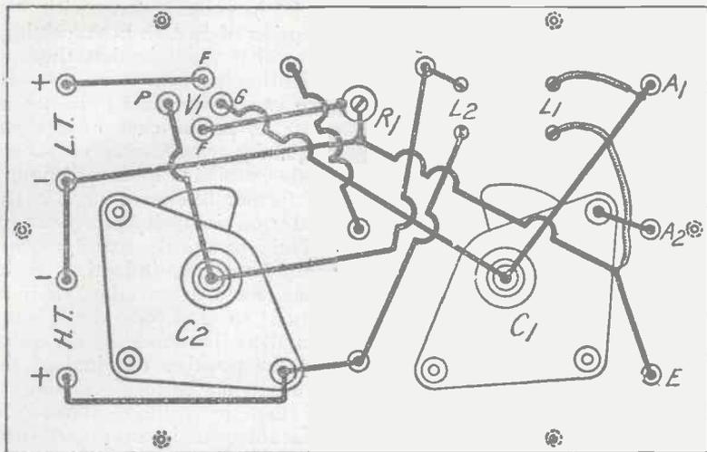
Fig. 8.—Wiring diagram of the valve and crystal receiver.
