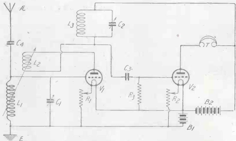
Fig. 1.—A popular method of stabilising a tuned anode circuit which is in common use in America.
