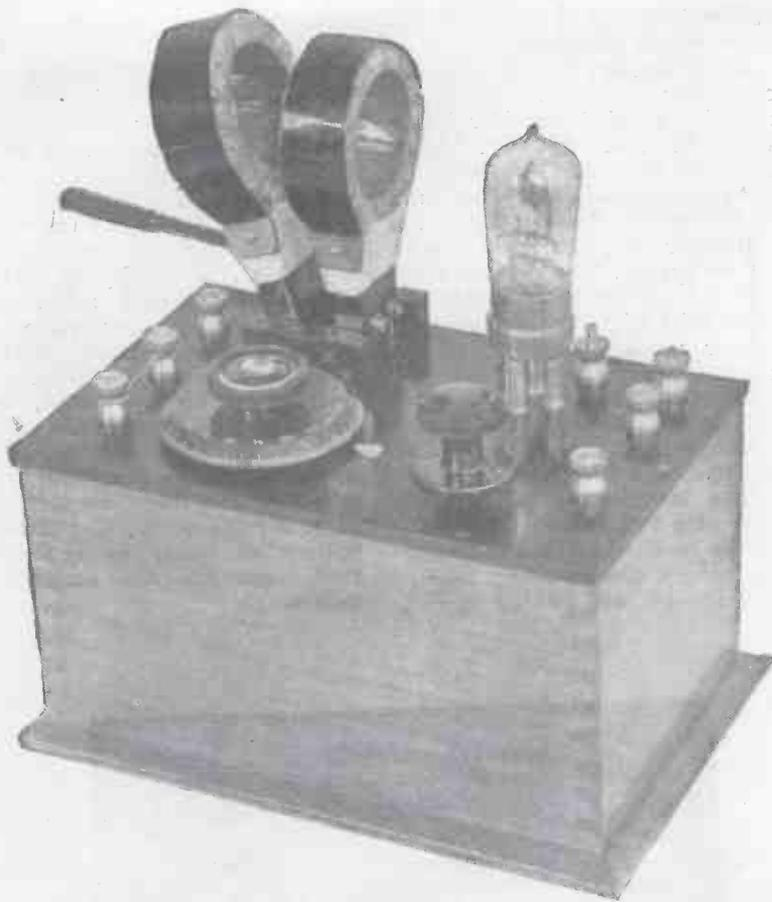
Fig. 1.—A single valve reaction receiver made up in a compact form for easy construction.
