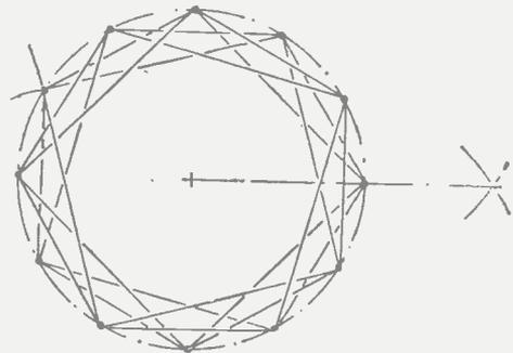
Fig. 3.—The appearance of the wound coil should be somewhat similar to this illustration.
