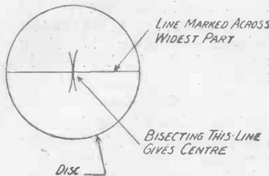
Fig. 1.—Indicating method of finding the centre.
