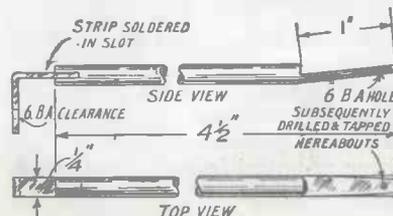
Fig. 3.—The dimensions of the brass radial arms.
