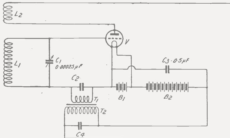
Fig. 3.—An experimental buzzer wavemeter circuit described.
