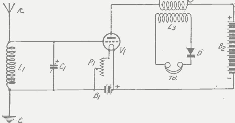
Fig. 9.—A diagram showing a detector circuit inductively coupled to the tuned anode circuit of the H.F. valve.
