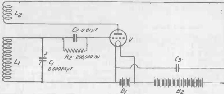
Fig. 4.—The Buzzerdyne circuit. The coils L1 and L2 are those of a plug-in transformer.
