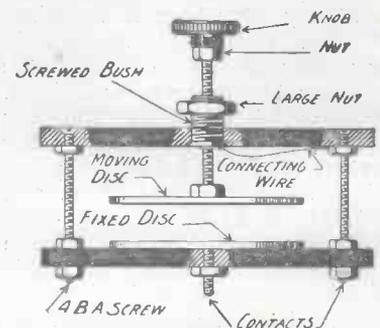
Fig. 5.—The assembly of the condenser.
