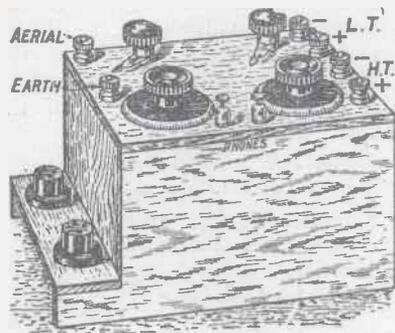
Fig. 3.—The framework, complete with panel and components mounted up.
