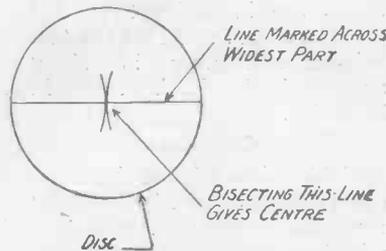
Fig. 1.—Indicating method of finding the centre.
