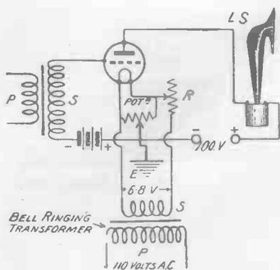
Fig. 1.—Circuit arrangement used to supply the filament current from the A.C. mains. The step-down transformer and potentiometer make this possible.
