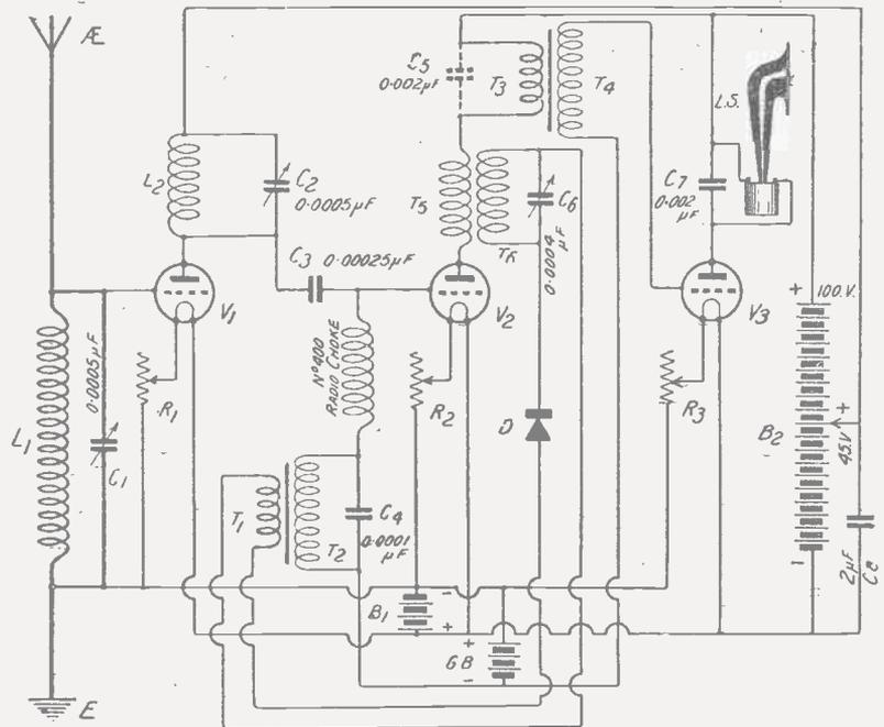
Fig. 1.—The reflex circuit referred to by "Medico."
