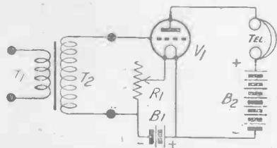
Fig. 1.—Maintaining the grid at a negative potential.
