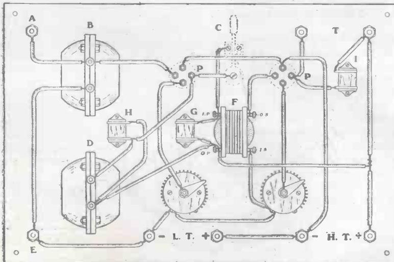
Fig. 3.—Practical Back of Panel Wiring Diagram.
