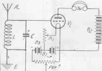
Fig. 3.—Rectification by the potentiometer method.
