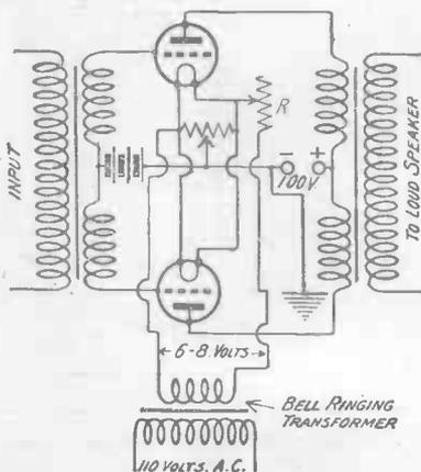
Fig. 2.—The circuit employed to supply current for the filaments of the valves in a push-pull amplifier from an 110 v. A.C. main.
