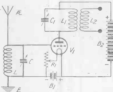
Fig. 2.—A high-frequency amplifier arrangement.
