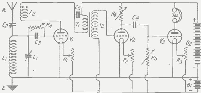
Fig. 1.—A circuit incorporating detector and two low-frequency stages.
