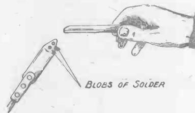
Fig. 2.—Illustrating how blobs are formed if the iron has not been properly cleaned.
