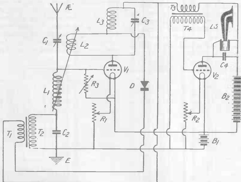
*Fig. 1.—The ST100 circuit, showing the variable resistance  $R_3$  and arrangement of anode coil for obtaining selectivity.*
