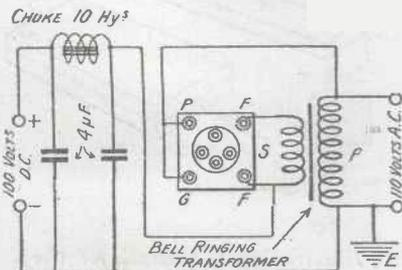
Fig. 3.—Method of obtaining rectified A.C. directly from the mains for amplifier plate voltage.
