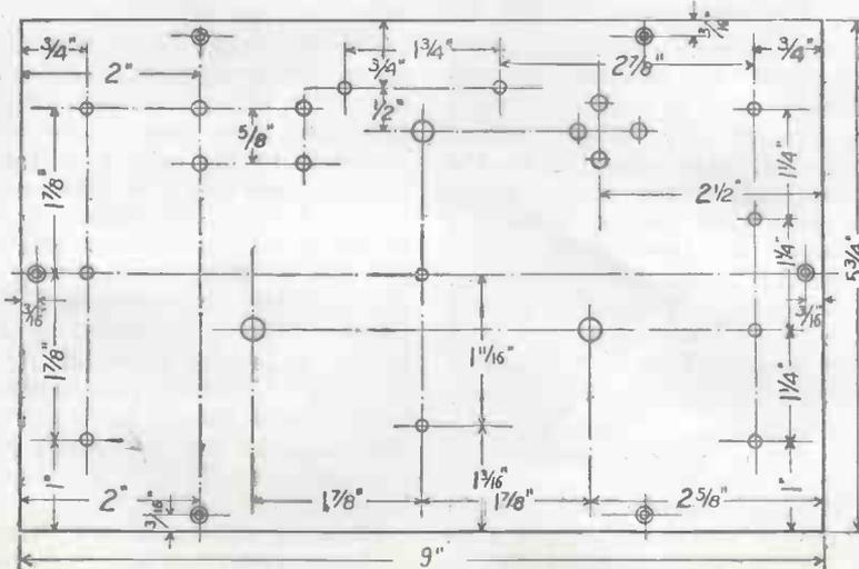
Fig. 6.—A drilling diagram of the ebonite panel.
