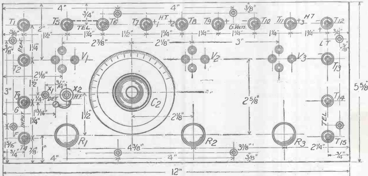
Fig. 3.—Drilling lay-out and terminal markings.
