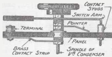
Fig. 1.—The double-purpose switch.
