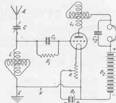
Fig. 7.—The tuned-anode method of obtaining reaction effect.
