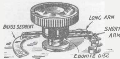
Fig. 2.—Details of the switch.
