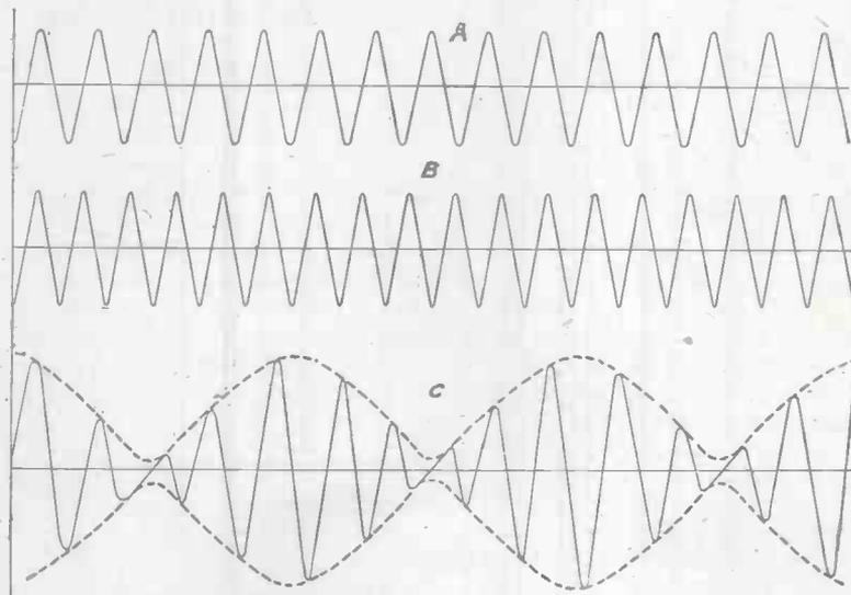
Fig. 9.—Showing "beats" produced by interference between superimposed oscillations of slightly different frequencies.
