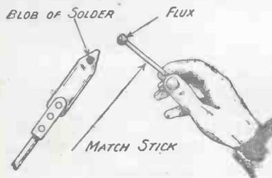
Fig. 1.—A suggested method for tinning the iron.
