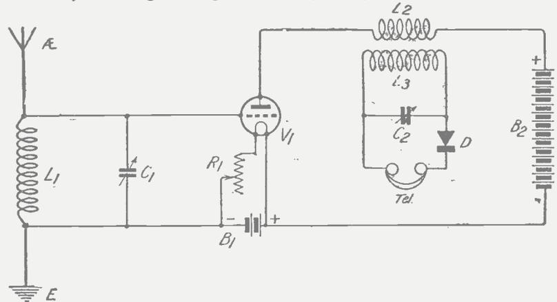
Fig. 11.—A circuit in which the coupling between the anode and detector circuits is effected by means of a high frequency transformer.
