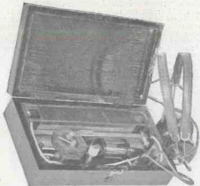
Fig. 1.—Terminals, coil and detector are all contained within the dustproof case.
