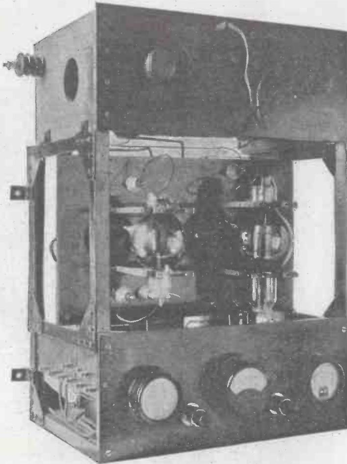
The 2,100-metre long-wave transmitter on board the "Arctic."
