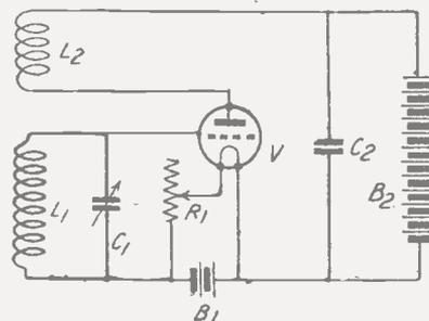
Fig. 2.—A simple heterodyne wavemeter circuit.
