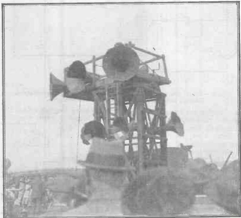
Our photograph shows the giant loud speakers used on the occasion of the high-power broadcasting demonstration on Walney Island, near Barrow-in-Furness. The battery of loud speakers consisted of eight individual horns.
