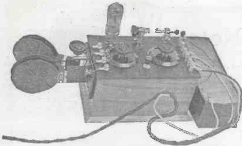
Fig. 1.—A simple and efficient receiver using one valve and a crystal detector.
