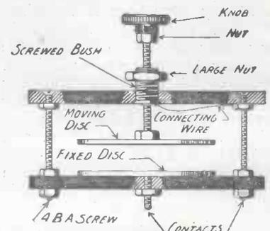
Fig. 5.—The assembly of the condenser.
