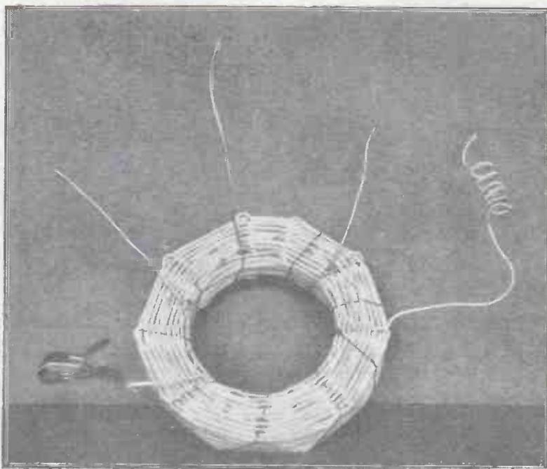
Fig. 1.—Note the position of the tappings. The "spring clip" terminal is convenient for experimental connections upon the coil.
