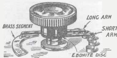
Fig. 2.—Details of the switch.
