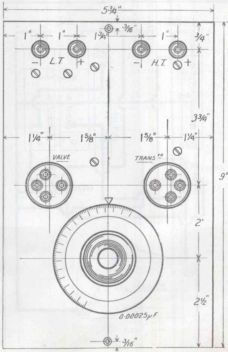
Fig. 5.—Drilling plan of the panel.
