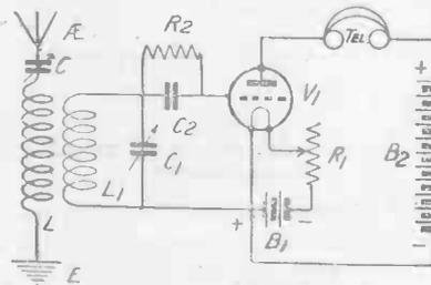
Fig. 6.—Grid condenser rectification.
