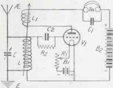
Fig. 8.—How continuous oscillations can be generated.
