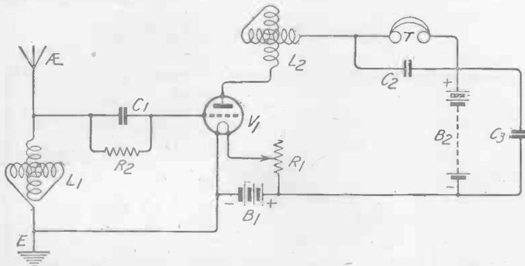
Fig. 2.—Illustrating an early American circuit using variometers. Though selective, this circuit is rather unstable.
