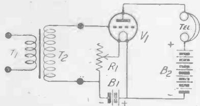
Fig. 1.—Maintaining the grid at a negative potential.
