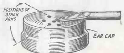
**Fig. 6.—How to fix the radial arms to the ebonite earcap.**
