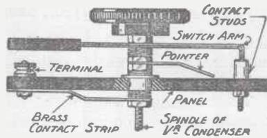
Fig. 1.—The double-purpose switch.
