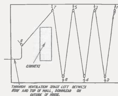
Fig. 4.—A roof aerial with a down lead on the outside of the house.
