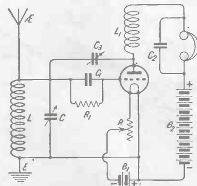
Fig. 9.—Electrostatic reaction obtained by means of variable condenser and choke coil.
