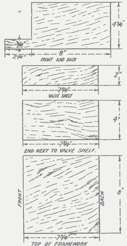
Fig. 2.—Details of the construction of the framework.
