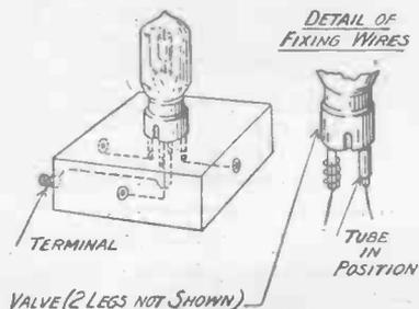
The method of mounting the valve may be seen above.
