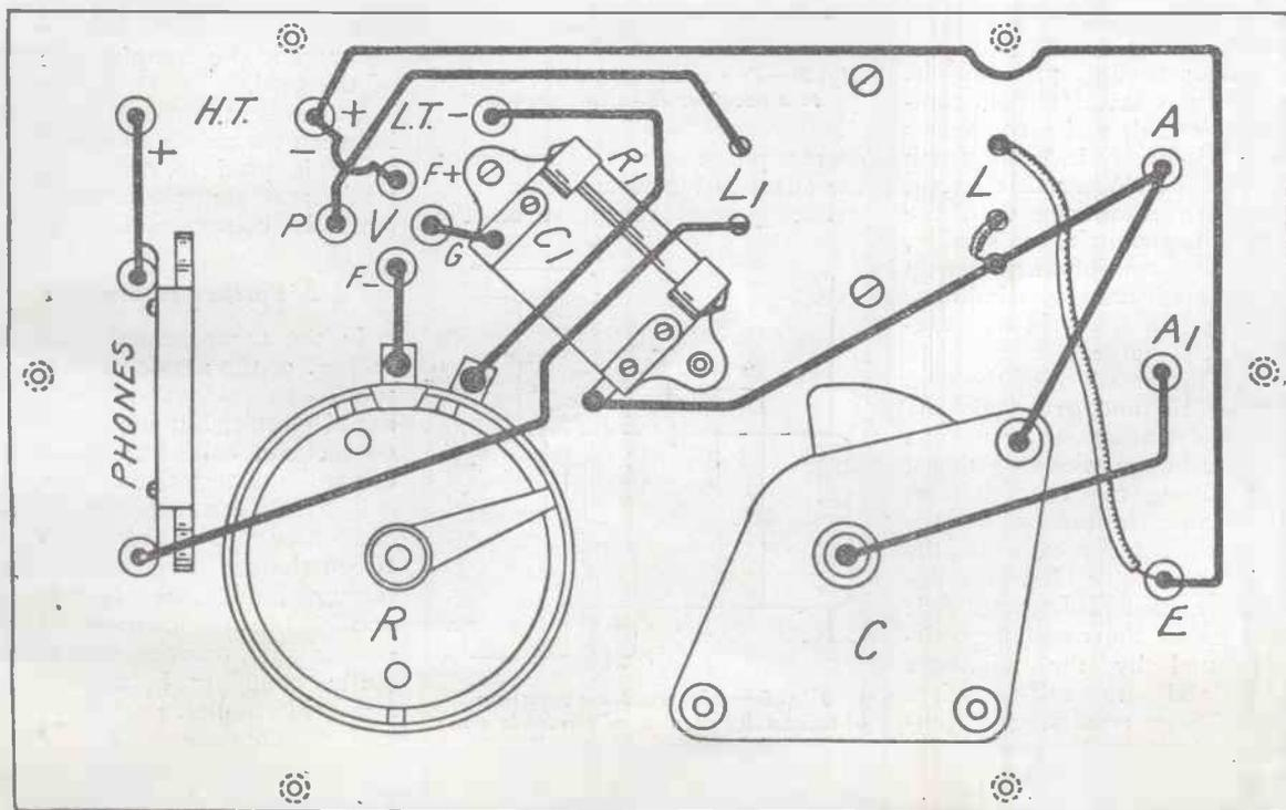
Fig. 6.—Back-of-panel wiring diagram of the single-valve receiver.
