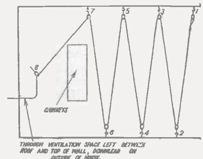
Fig. 4.—A roof aerial with a down lead on the outside of the house.
