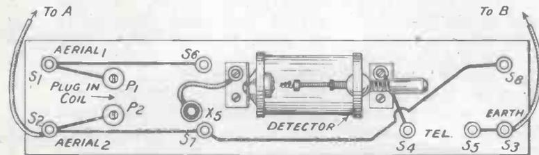
bled is the crystal detector. The connections for the detector are made as follows. Pass a wire from socket S1 to S6 and on to the pin P1. Pass a further wire from the pin P2 to socket S2, and on to S7, and on again to S8. The detector is connected on the
