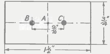
Fig. 3.—Dimensions for a jig for inductance coil sockets.
