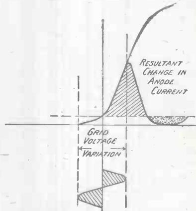
Fig. 4.—Effect of variation of grid potential.
