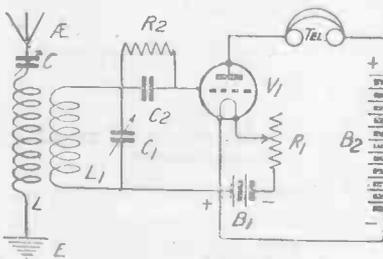
Fig. 6.—Grid condenser rectification.
