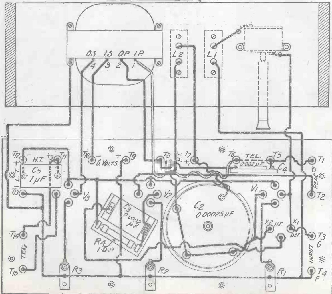
Fig. 4.—Wiring diagram showing connections to coils, neutrodyne condenser and transformer mounted on side of the case.
