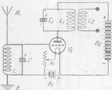
Fig. 2.—A high-frequency amplifier arrangement.
