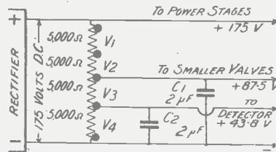
Fig. 5.—Potentiometer for obtaining several values of plate voltage simultaneously. C1 and C2 are bypass condensers.
