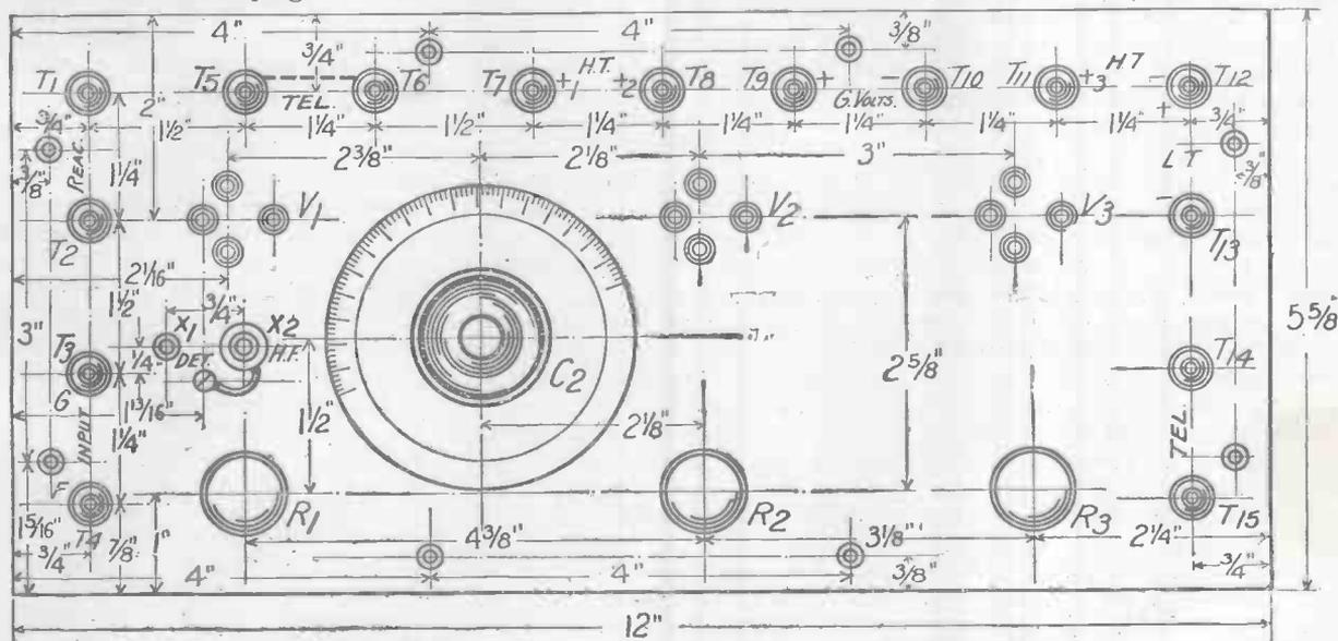
Fig. 3.—Drilling lay-out and terminal markings.
