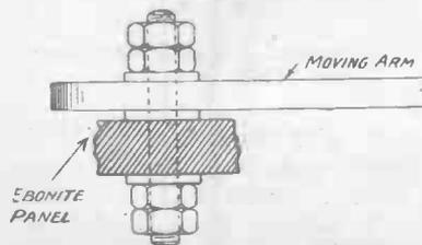
Fig. 4.—The pivot shown at A in Fig. 1.
