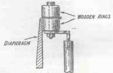
Fig. 4.—How the radial arms are fixed to the diaphragm frame.
