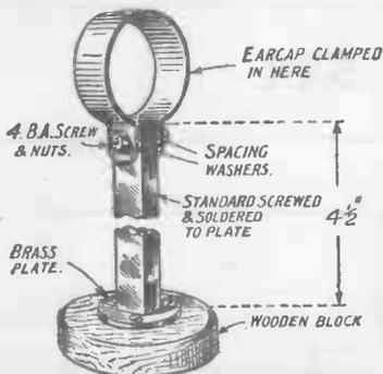
**Fig. 5.—Details of the standard and earpiece clamp.**
