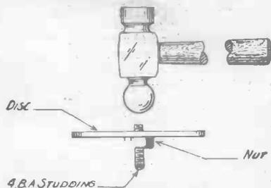
Fig. 2.—How the riveting is done.
