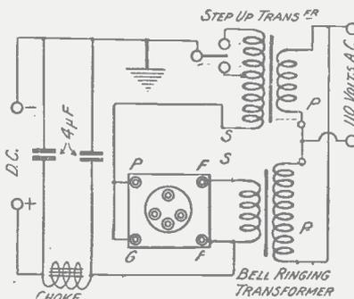
Fig. 4.—Method of obtaining rectified A.C. when using a step-up transformer.
