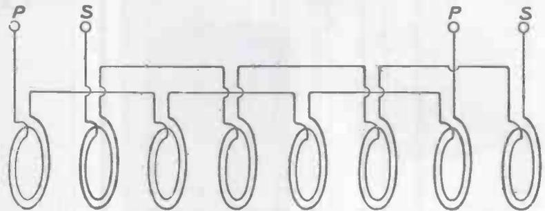
Fig. 2.—Showing how the primary and secondary slots are connected.
