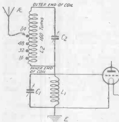
Fig. 6.—The connections of the trap illustrated in the photographs.
