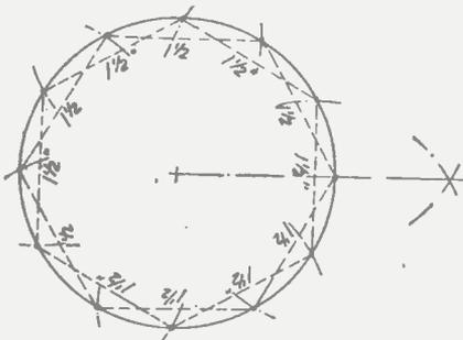
Fig. 1.—Showing how the positions for the nails are found.
