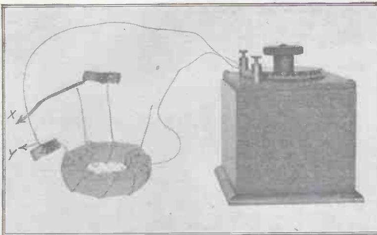
Fig. 2.—The leads X and Y are connected to the aerial and the aerial terminal of the set respectively. Compare with Fig. 6.
