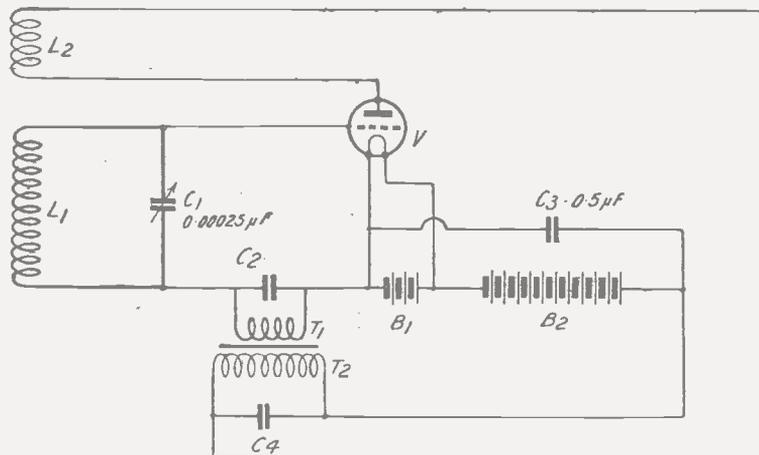
Fig. 3.—An experimental buzzer wavemeter circuit described.
