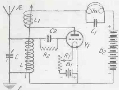
Fig. 8.—How continuous oscillations can be generated.
