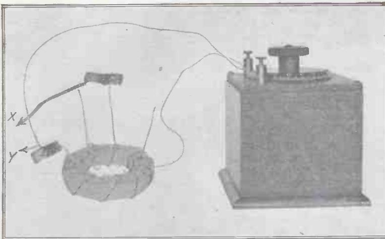
Fig. 2.—The leads X and Y are connected to the aerial and the aerial terminal of the set respectively. Compare with Fig. 6.
