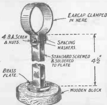
**Fig. 5.—Details of the standard and earpiece clamp.**
