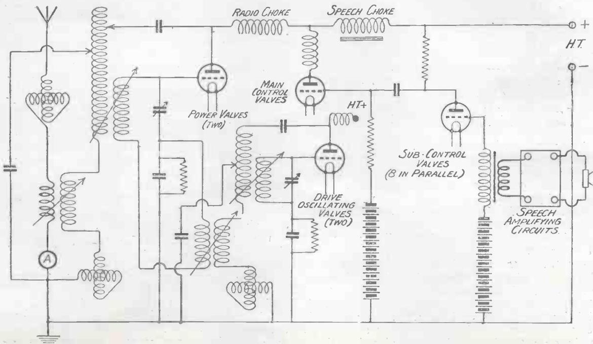
A diagram of the 5XX transmitter circuit. For simplicity, the rectifying valves, smoothing circuits, and the filament connections have been omitted. Choke control is used.
