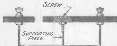
Showing how long leads may be supported to overcome microphonic effects caused through the wire.
