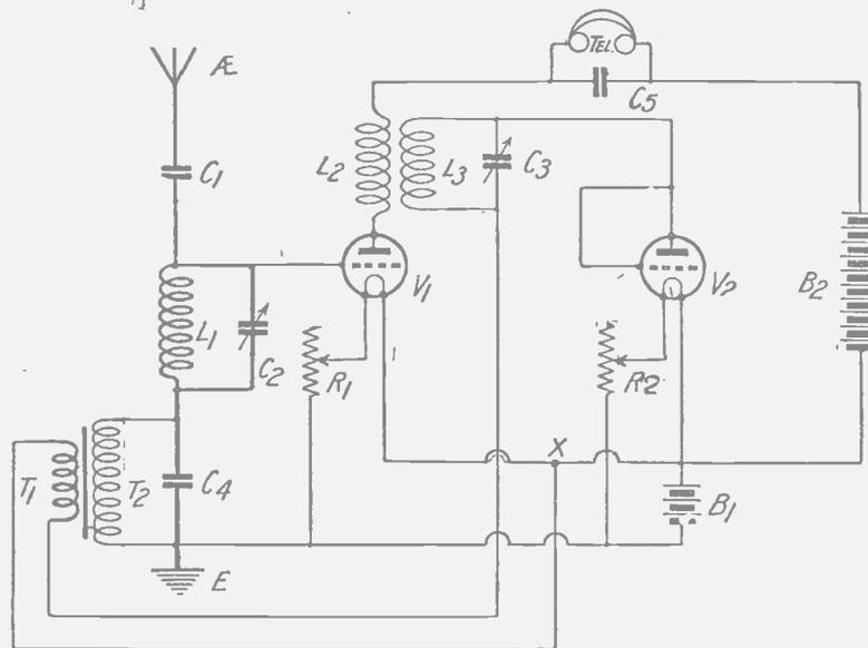
**Fig. 1.—A simple reflex circuit, in which the usual crystal detector is replaced by a two-electrode valve.**
