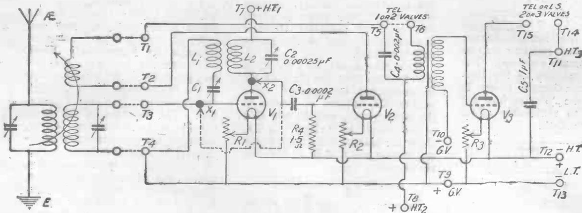
Fig. 2.—Complete circuit diagram, including tuner (a separate unit).
