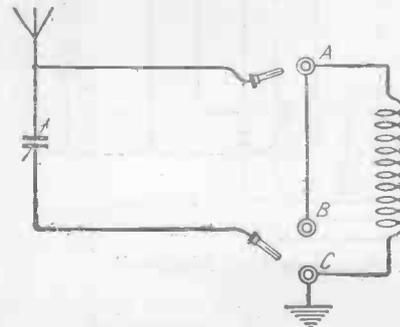
Fig. 2.—The series-parallel arrangement suggested by Mr. Kyffin.
