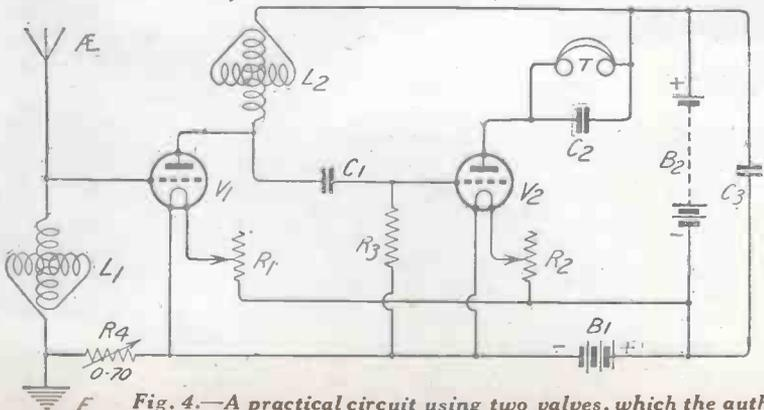
Fig. 4.—A practical circuit using two valves, which the author claims to be as sensitive as many three-valve arrangements.
