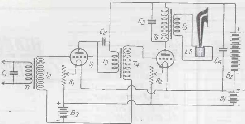
Fig. 1.—The circuit arrangement of the note magnifier.
