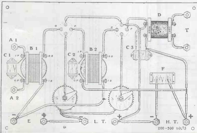
Fig. 3.—Practical back-of-panel wiring diagram.
