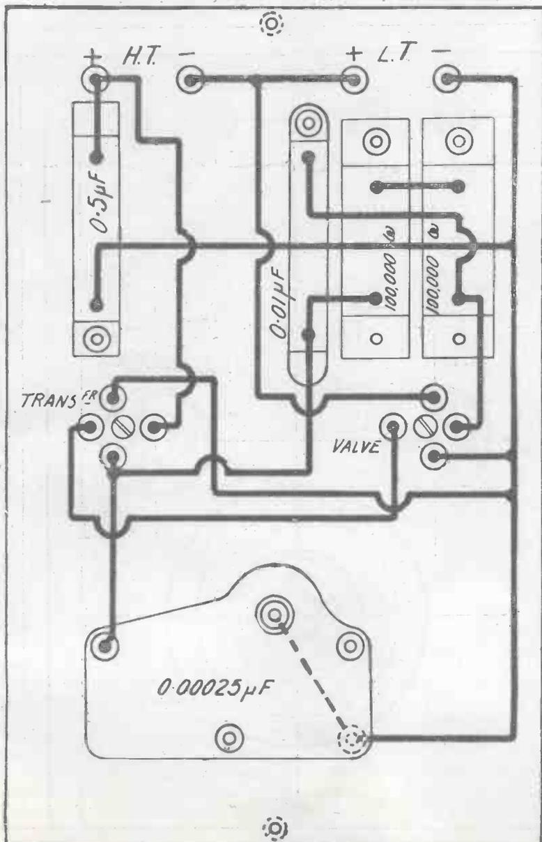
Fig. 6.—Practical wiring diagram.
