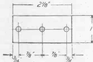
Fig. 3.—The layout of the top and bottom ebonite pieces.
