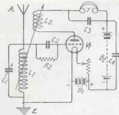
Fig. 1.—Showing an ordinary English magnetically coupled circuit.
