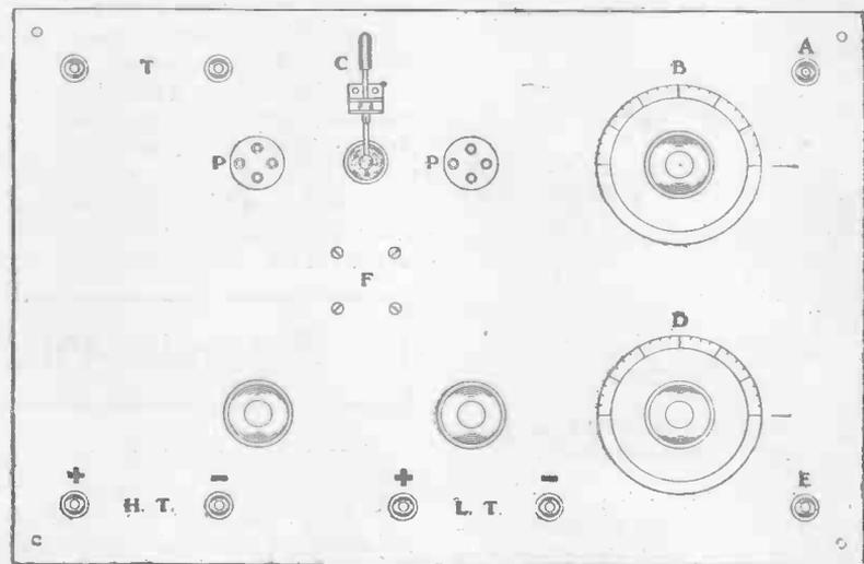
Fig. 2.—Panel Layout, Showing Position of Components.
