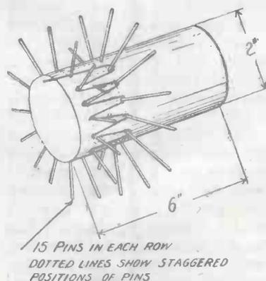
Fig. 7.—Showing how a zig-zag turn is wound in the lattice method.
