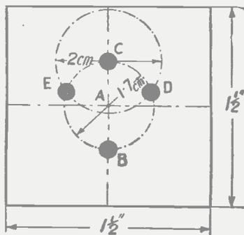
Fig. 1.—The position of valve legs is determined by measurement.
