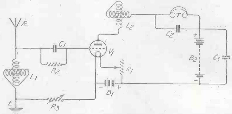
Fig. 3.—Showing a modified arrangement which, besides being selective, has high amplifying powers.
