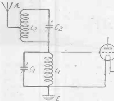
Fig. 5.—The type D wave-trap.
