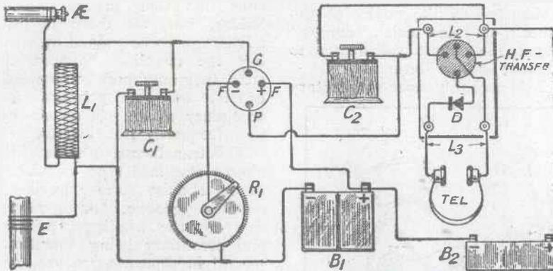
Fig. 10.—A pictorial representation of the circuit given in Fig. 9.
