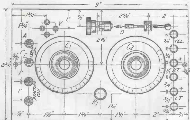
Fig. 3.—The layout of the panel, indicating positions of components and purposes served by the terminals. Blue print No. 60a.
