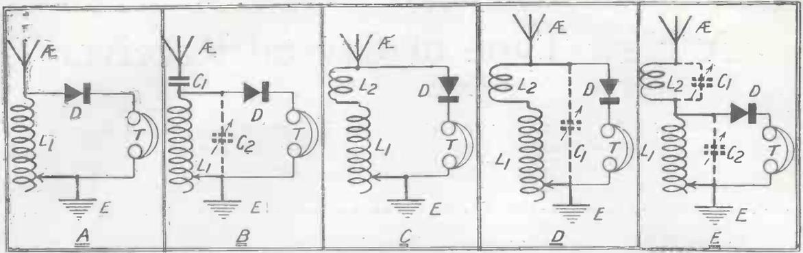
Fig. 9.—Examples of various types of circuits which may be obtained.
