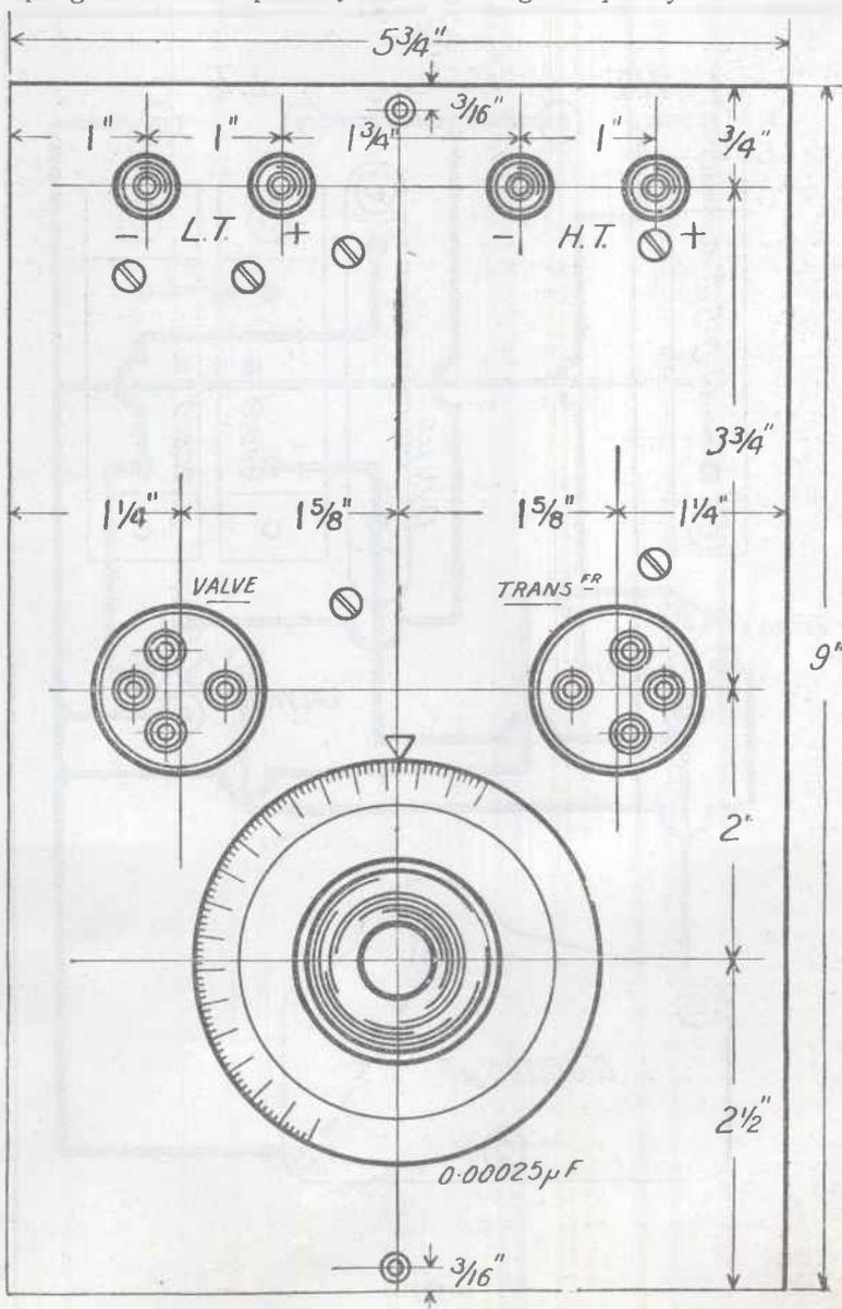
Fig. 5.—Drilling plan of the panel.
