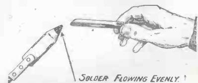
Fig. 3.—Showing how the solder will run freely when the iron has been cleaned before tinning.
