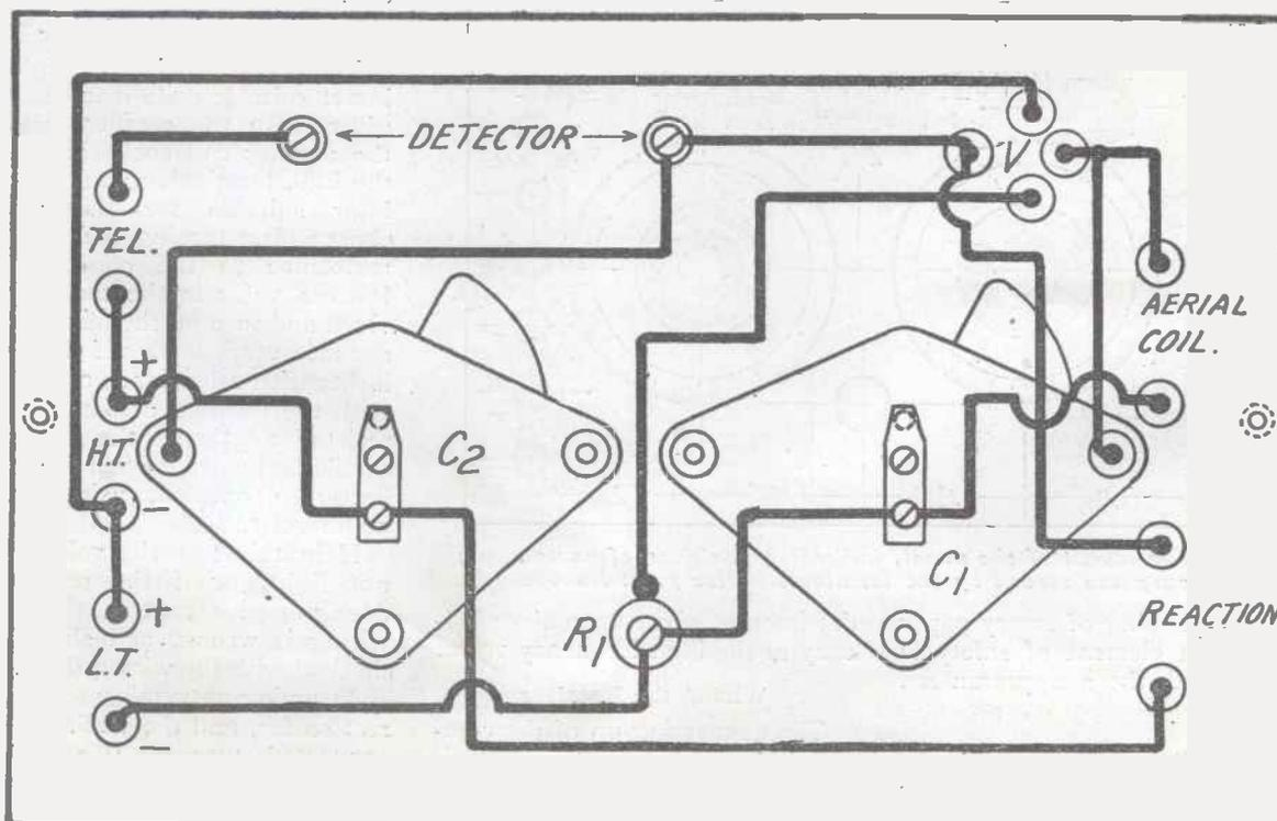
Fig. 5.—Practical back-of-panel wiring diagram. Blueprint No. 60b.
