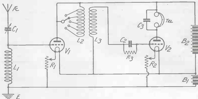
Fig. 1.—Illustrating the arrangement of the switch upon a semi-tuned transformer.
