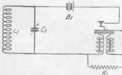
*Fig. 1.—A simple buzzer wavemeter circuit.*
