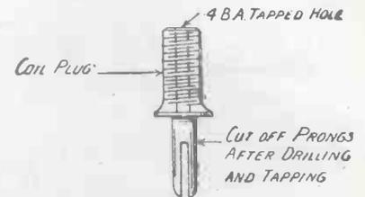
Fig. 4.—Details of the back.
