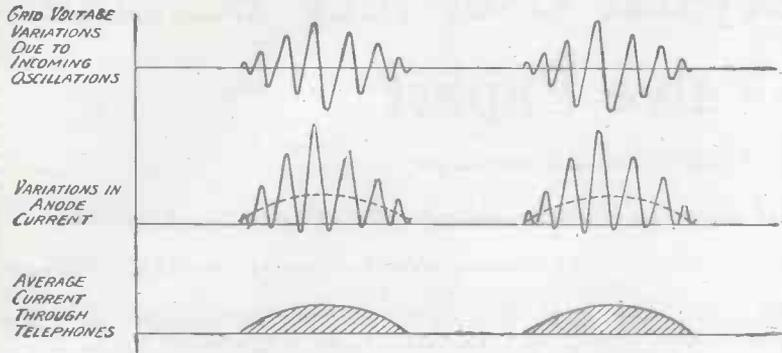
Fig. 5.—Effect produced by two complete trains of waves.
