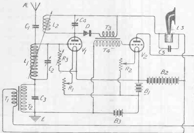
*Fig. 1.—A form of circuit which compares favourably with the well-known ST100.*
