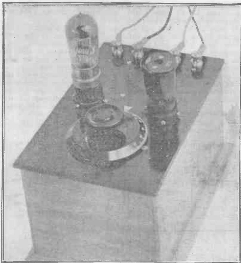
*The Buzzerdyne is compact, even for a wavemeter.*
