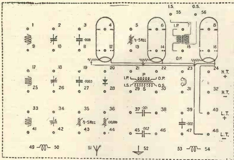
Fig. 1—The terminal board.
