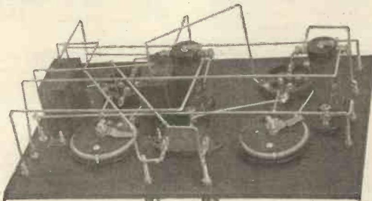
Fig. 8.—Perspective view of back-of-panel wiring.
