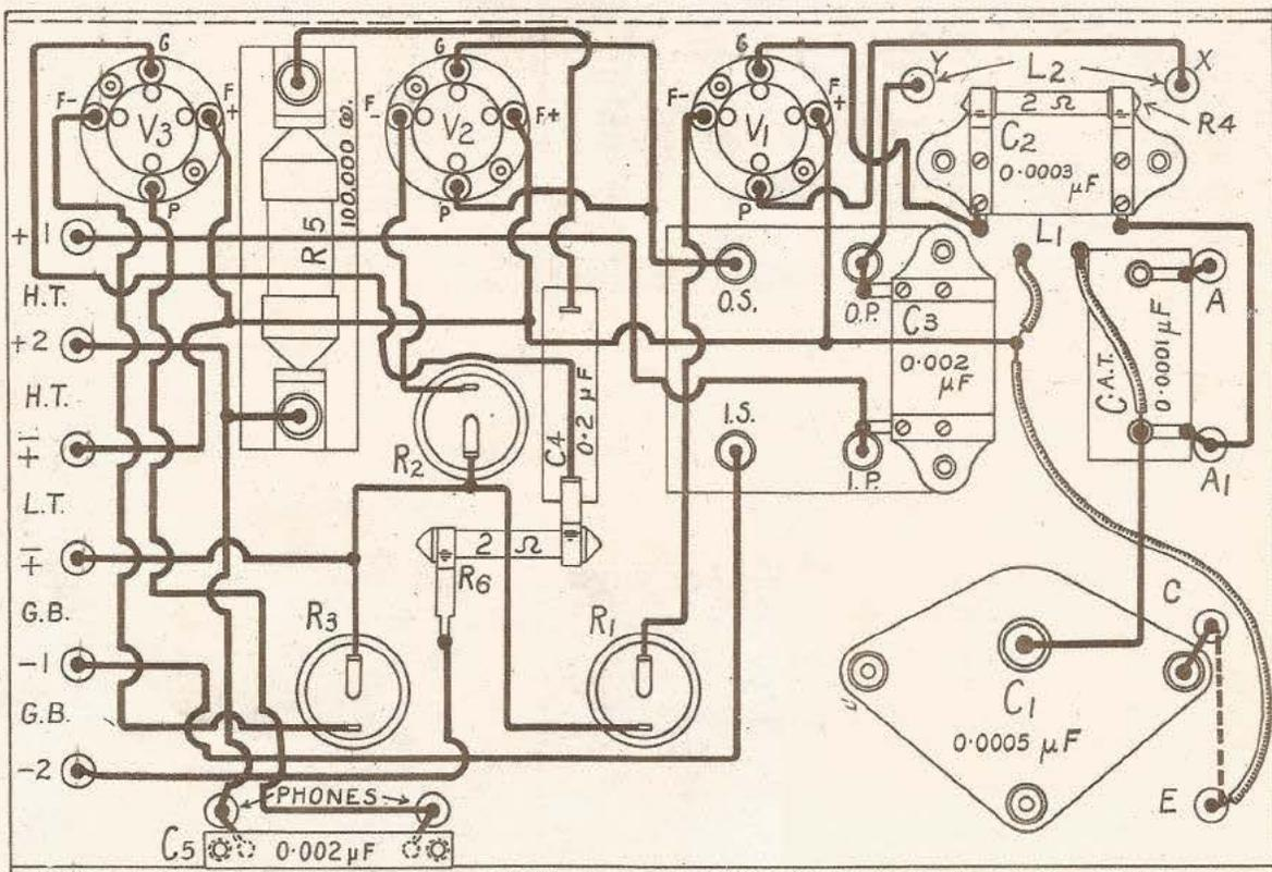
Fig. 7.—Practical wiring diagram. Blueprint 68b.
