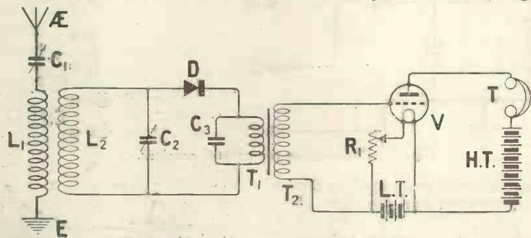
Fig. 2.—The circuit arrangements.
