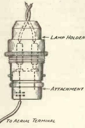
Fig. 2.—Principle of the plug-in attachment.
