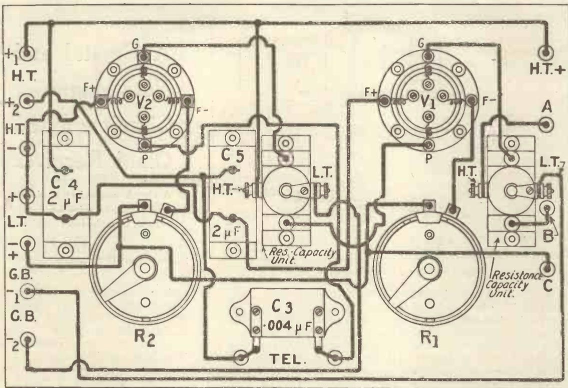
Fig. 6.—Practical wiring diagram.
