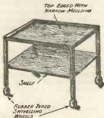
Fig. 1.—The type of wireless table referred to in the article.
