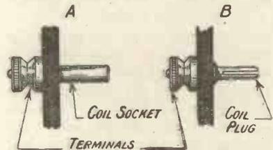
A good device in both of these instances is to in the first case employ a socket for the aerial connection, and a plug for the earth connection, and likewise in the latter case, thus obviating the possibility of linking up incorrectly. H. B.
