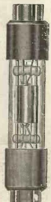
By virtue of the high electronic emission of the MYERS it is possible to obtain perfect results with only 2½ volts on the filament.
