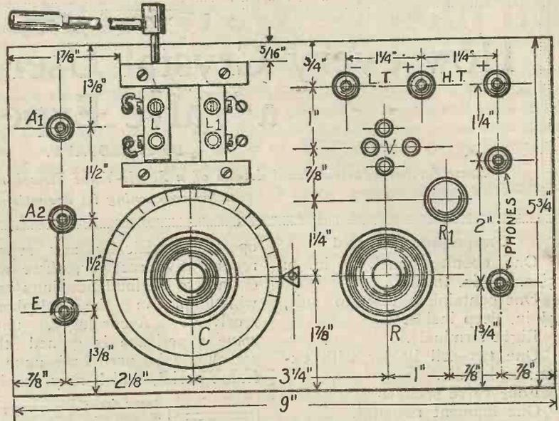
Fig. 7.—The layout of the panel showing dimensions.
