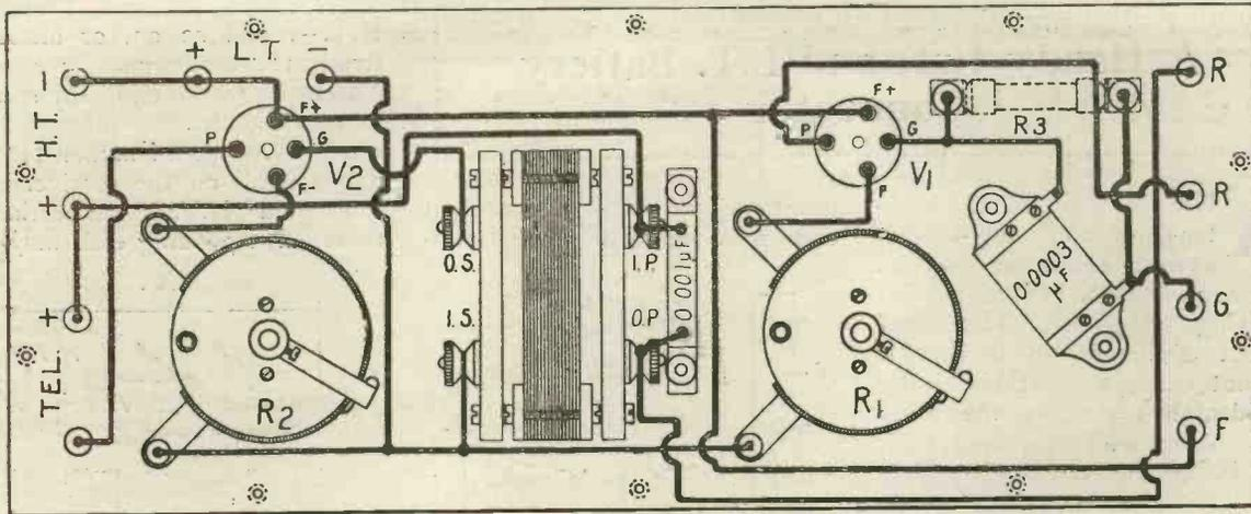
Fig. 8.—Practical back of panel wiring diagram.
