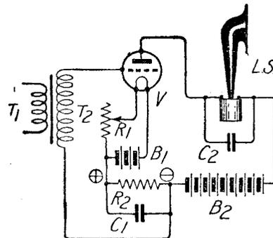
Fig. 1.—An interesting method of obtaining grid bias.
