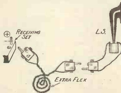
Fig. 2.—Method of making extensions.
