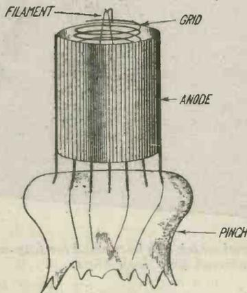
Fig. 2.—The electrodes of a power valve.
