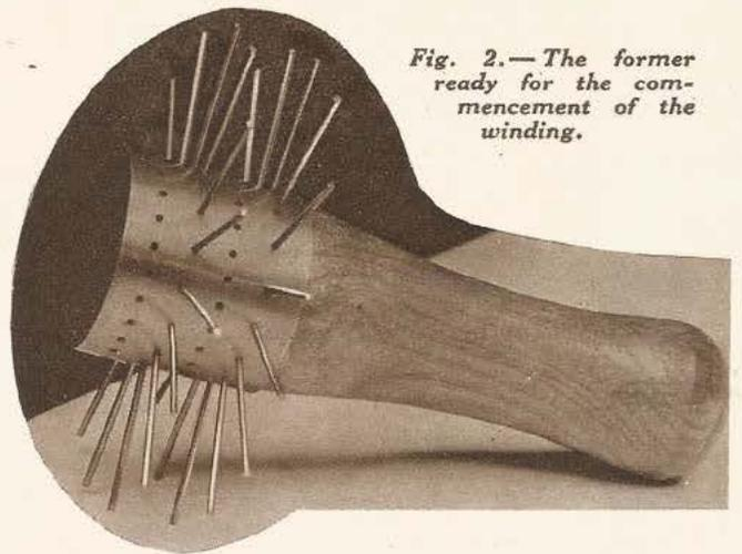
Fig. 2.—The former ready for the commencement of the winding.
