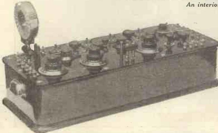
*The Four-Valve Family Receiver as made up by Mr. Guidalevitch.*
