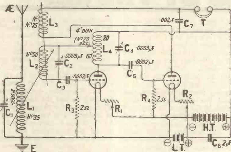
Fig. 3.—A practical "neutral-grid" broadcast receiver.
