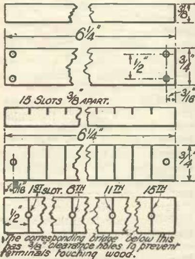
Figs. 1, 2, 3, illustrating the wood strips, the ebonite bridges and position of terminals.
