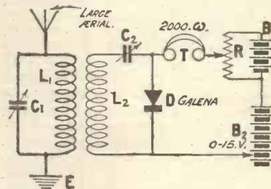
Fig. 3.—The circuit employed by Dr. Pickard in his successful attempts to receive C.W. signals on a crystal.
