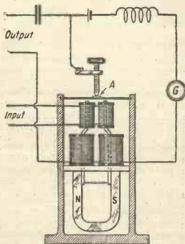
Fig. 1.—The patent drawing of S. G. Brown's microphone amplifier. The instrument Dr. Pickard found to be a sensitive detector of oscillations.
