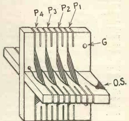
Fig. 4.—The secondary winding completed.
