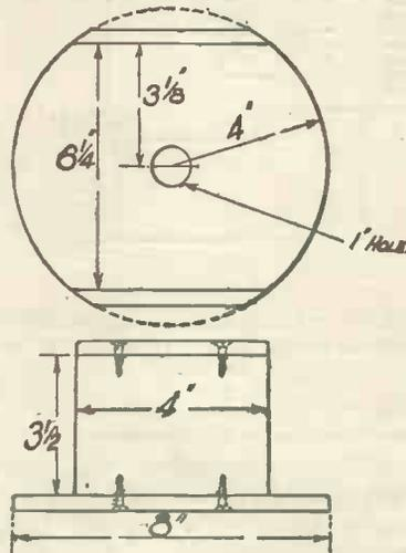
Fig. 4.—Constructional details of the disc and side pieces.
