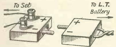
Fig. 4.—A useful safety adapter for L.T. connections.
