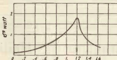
Fig. 2.—Characteristic curve of a galena crystal.
