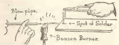
Fig. 2.—Sweating a small spring to a strip of brass.
