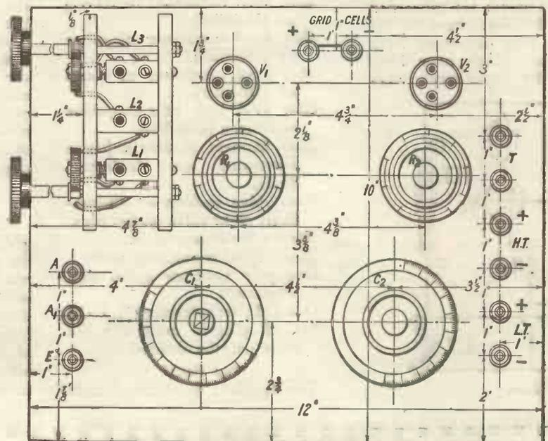
Fig. 4.—The panel layout. Blueprint No. 83a.
