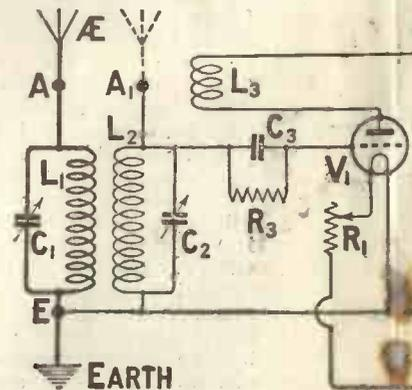
Fig. 2.—The theoretical circuit diagram.
