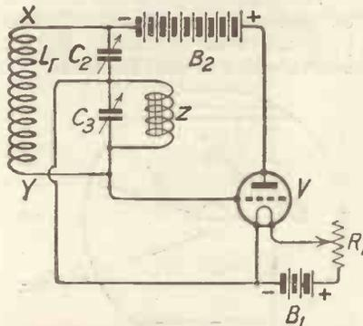
Fig. 31.—A single valve regenerative circuit using two condensers in series.
