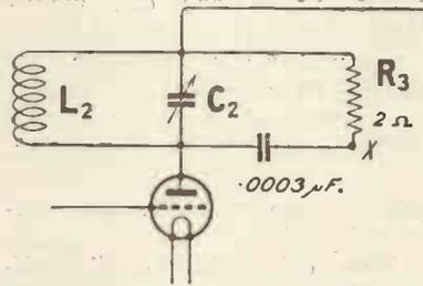
Fig. 2.—Showing that  $R_3$  is virtually in parallel with  $L_2 C_2$ .
