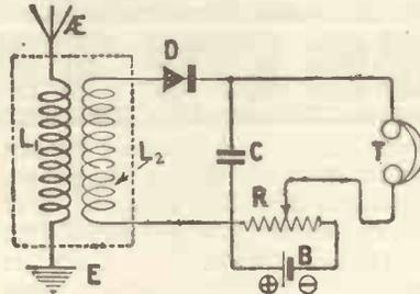
Fig. 5.—A copy of the circuit contained in a patent issued to Dr. Pickard on oscillating crystal circuits.
