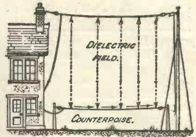
Fig. 2.—The effect of insulated counterpoise.
