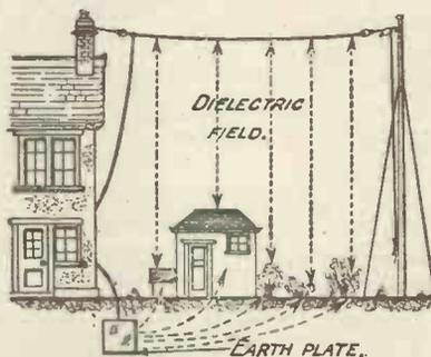
Fig. 1.—Illustrating the current paths in earth, and partly conducting objects.
