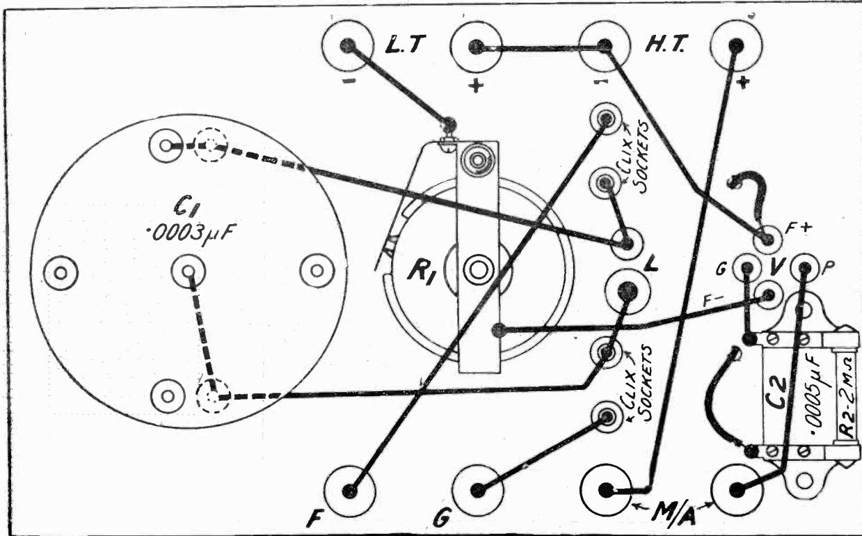
The wiring of the unit. L indicates the coil socket.
