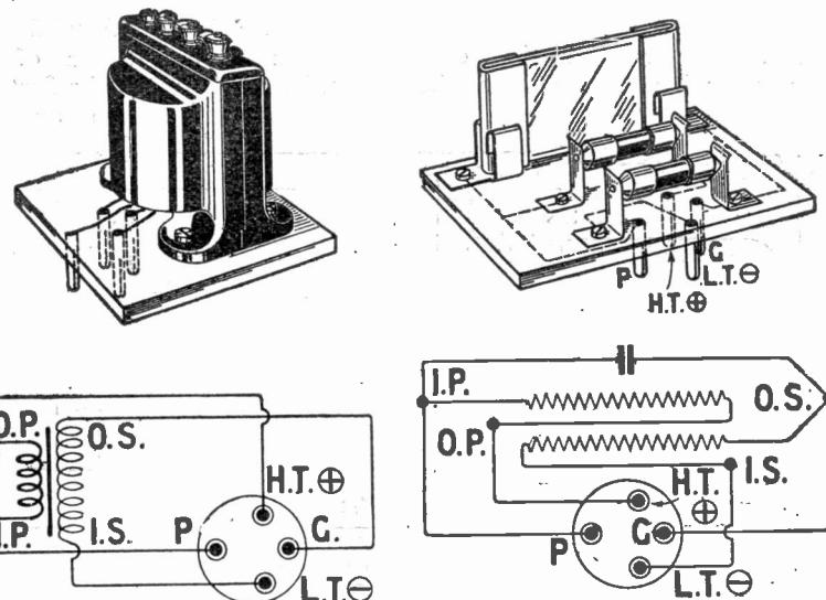
Figs. 5 and 6.—Illustrating how the interchangeable units are mounted and connected.
