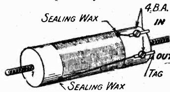
*Fig. 5.—Showing method of securing the wire in the choke coil.*
