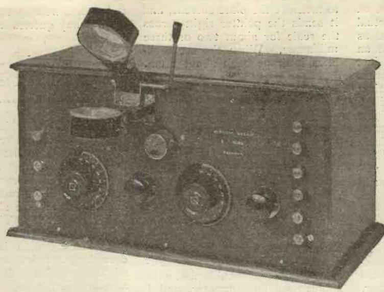
Fig. 1.—The handsome appearance of the receiver may be seen in this photograph. The novel form of crystal detector seen in the centre of the panel should be noted.
