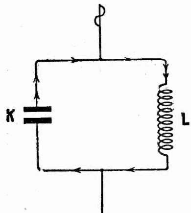
Fig. 6.—True direction of current flow in an oscillatory circuit.
