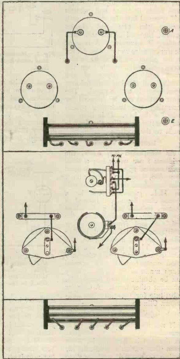
Fig. 2.—Disposition of parts on back of panel.
