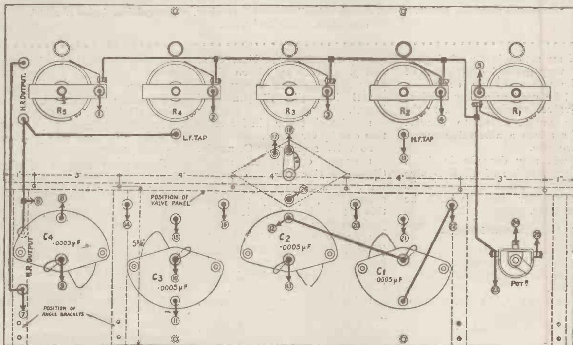
Fig. 2.—The wiring arrangements behind the main panel, which should be used in conjunction with the valve panel seen in Fig. 3. The numbers on this drawing indicate that these connections are continued to similar numbers on the valve panel. Blue print 94b.
