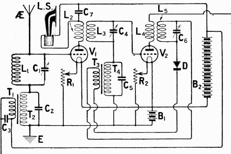
**Fig. 3.—A modification of the Grimes Inverse Duplex circuit.**
