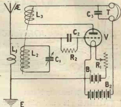
**Fig. 6.** — A circuit employing trap tuning is also a very effective means of obtaining selectivity.
