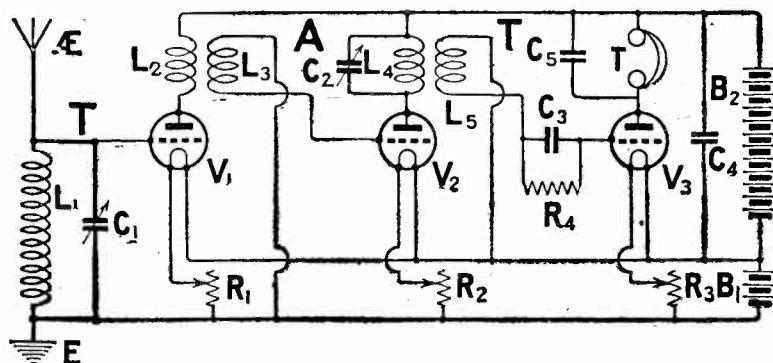
Fig. 2.—A T.A.T. circuit in which H.F. transformer coupling is employed.
