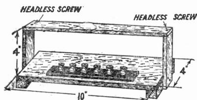
*Fig. 1.—Shows the main dimensions of the wooden frame.*
