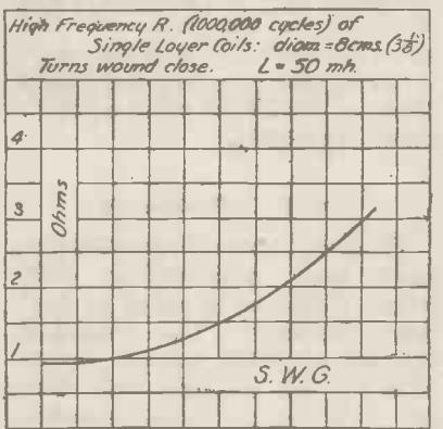
Fig. 5.—Showing the H.F. resistance of coils wound upon the same former with different gauges of wire to produce an inductance of 50 microhenries.
