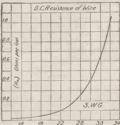
Fig. 9.—The variation of  $R_o$  and resistance ratio for single-layer coils.
