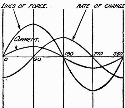
Fig. 2.—Illustrating the relation between magnetic field and its rate of change.
