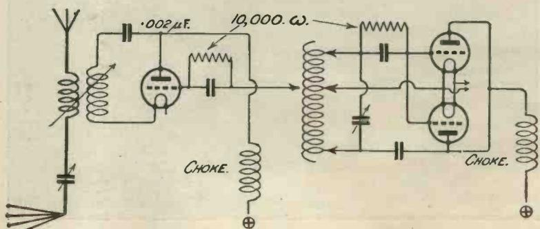
*The Master Oscillator circuit used at 2DX.*
