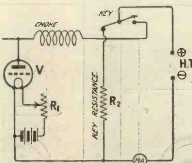
Fig. 4.—One method of keying in the H.T., with back-load connection. This method needs a carefully shielded keylever to avoid risk of shock to the operator.
