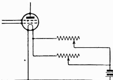
Fig. 2.—The reaction control.
