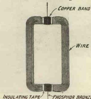
Fig. 3.—The finished coil will have this shape.
