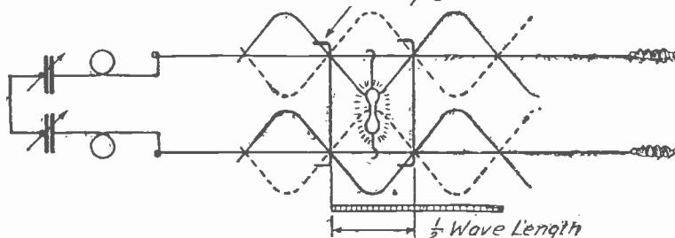
Fig. 8.—Illustrating the theory of the method of measuring short wavelengths.
