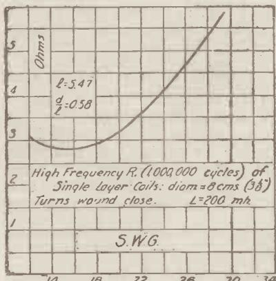
Fig. 7.—Curve produced when using a coil of 200 microhenries.
