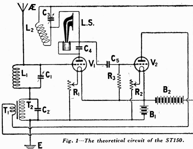
Fig. 1—The theoretical circuit of the ST150.
