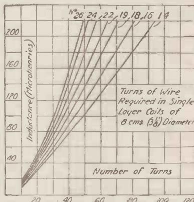
Fig. 8.—Showing number of turns required in single-layer coils of the same diameter to give different values of inductance.
