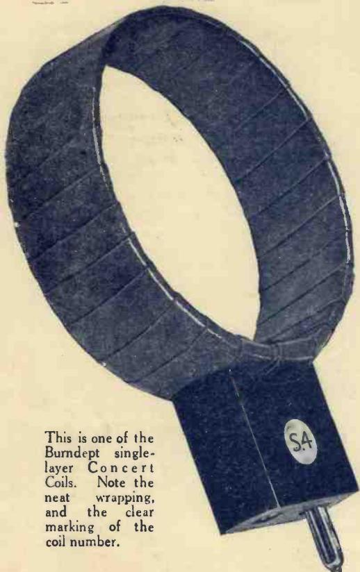
This is one of the Burndep single-layer Concert Coils. Note the neat wrapping, and the clear marking of the coil number.
