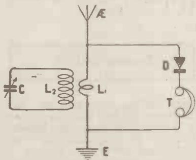
*Fig. 1 shows the method of applying trap tuning to the aerial circuit.*
