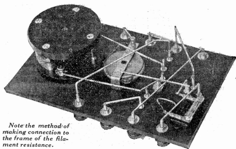
Note the method of making connection to the frame of the filament resistance.
