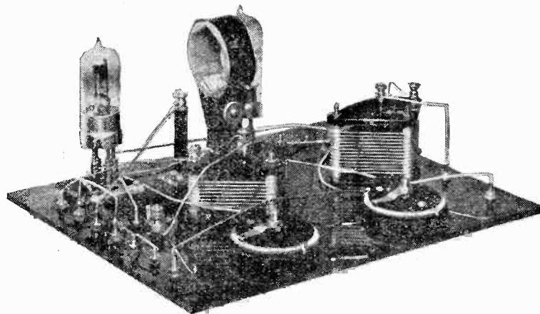
*Showing the valves and anode coil.*
