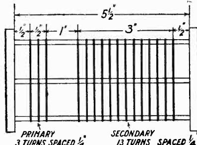
Fig. 2.—Illustrating the method of winding the coil.
