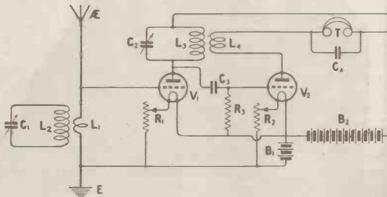
*Fig. 3.—Trap aerial tuning applied to the ST34 circuit.*
