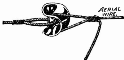
*Fig. 2.—A better arrangement for connecting the down lead.*
