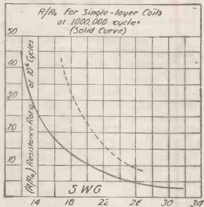
Fig. 10.—Showing the variation in  $R/R_o$  for single-layer coils at 1,000,000 cycles.
