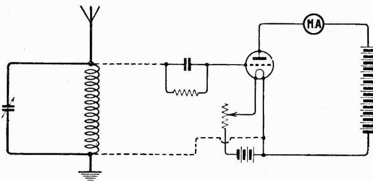
Fig. 1.—The connections of the simple circuit required in making the measurements described in this article.
