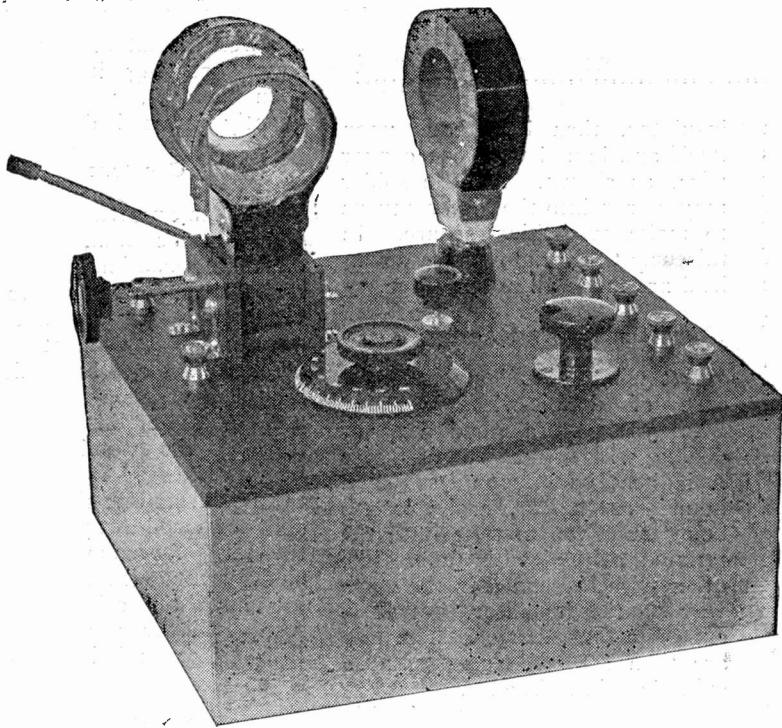
*Fig. 1.—The Ultraaudion circuit as constructed, the valve being beneath the panel.*
