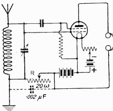
Fig. 3.—An alternative method of control.
