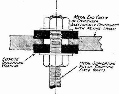
*This diagram shows the method of clamping the fixed plates of Burn-dept condensers.*
