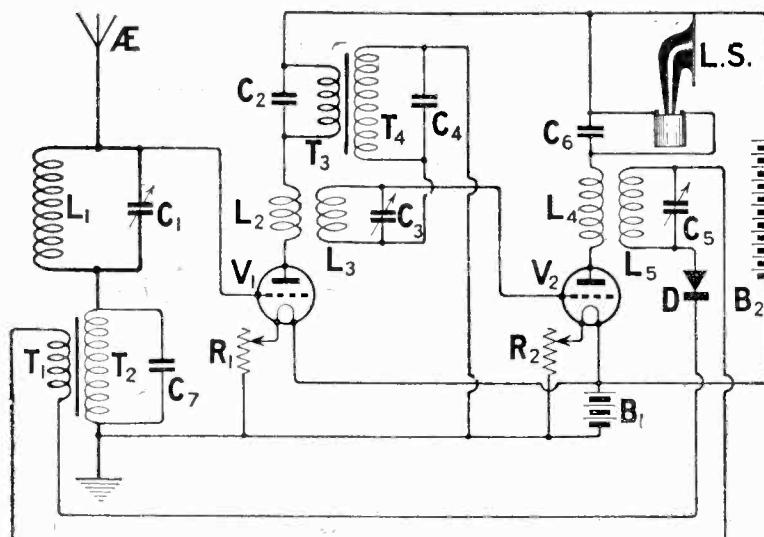
Fig. 1.—A circuit in which the two valves are being used as simultaneous high- and low-frequency amplifiers.
