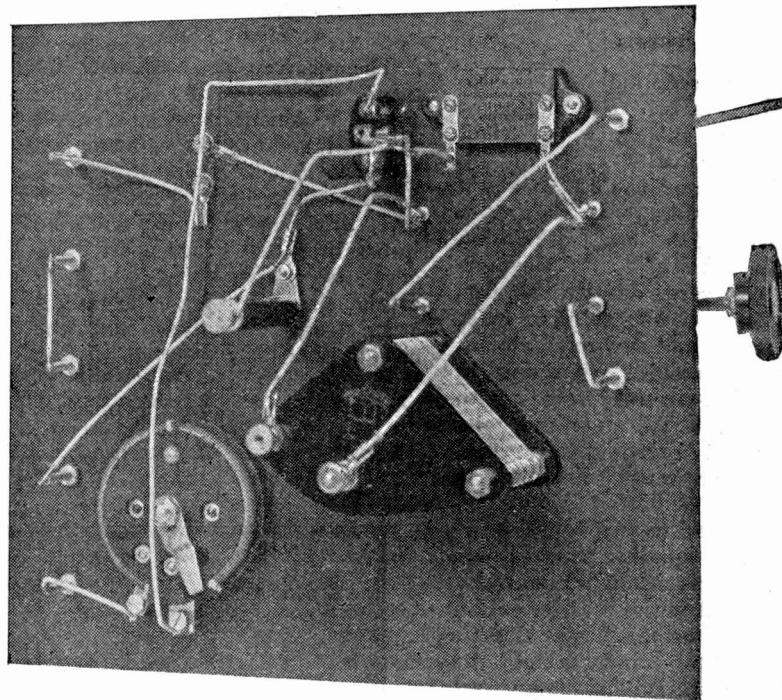
Fig. 3.—Back-of-panel wiring.
