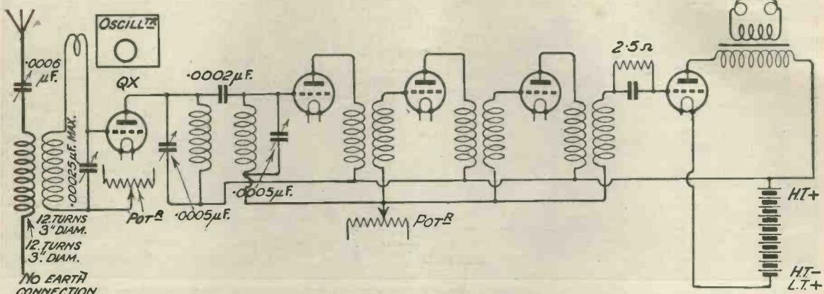
The essentials of the supersonic heterodyne receiver at 2DX. For simplicity the filament connections and L.T. batteries have been omitted.
