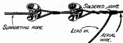
*Fig. 1.—A common form of down-lead connection.*
