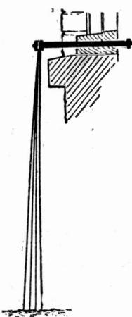
Fig. 1.—How the earth connection may be brought into the house to keep it clear of the wall.
