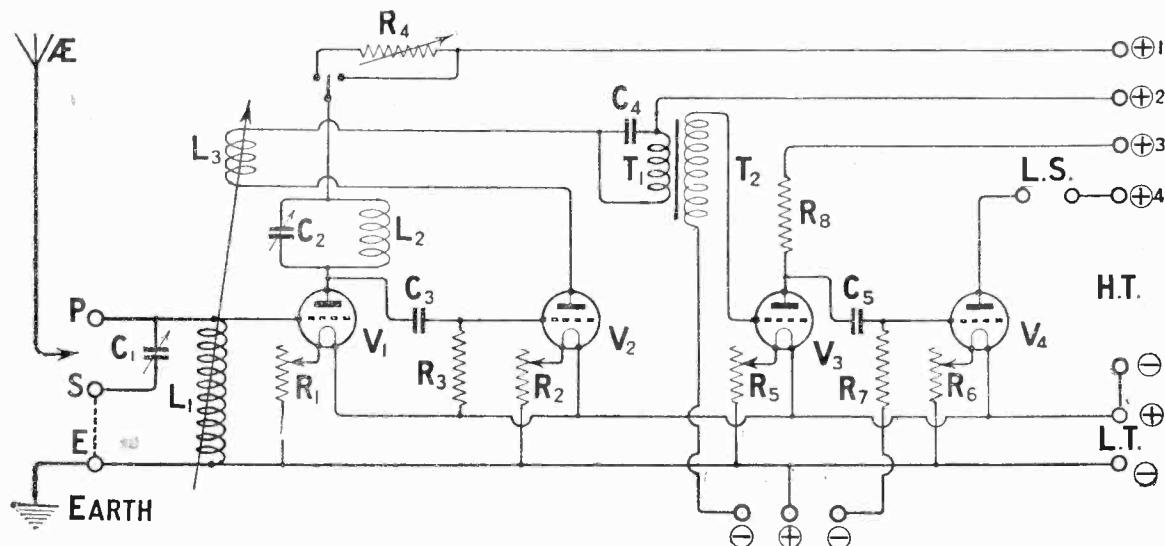
Fig. 4.—Showing the connections necessary when a two-valve amplifier is added, the last stage of L.F. being resistance coupled.
