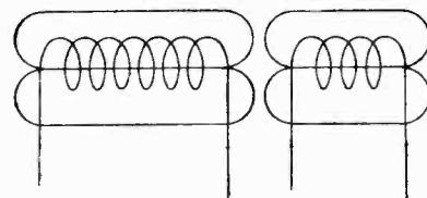
Fig. 8.—Separating the turns reduces the self-induction.
