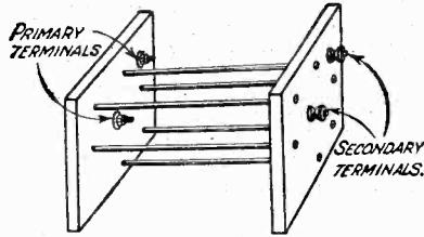
Fig. 1.—Details of the coil former.
