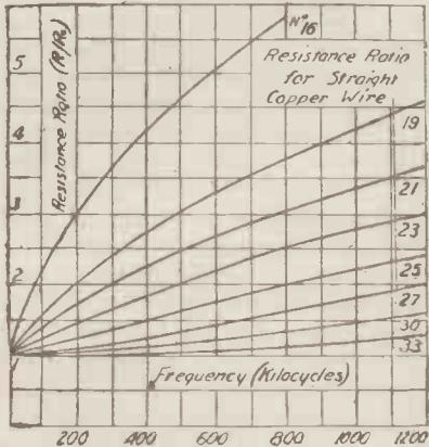
Fig. 2.—Curves showing relation between frequency and resistance ratio for straight copper wires.
