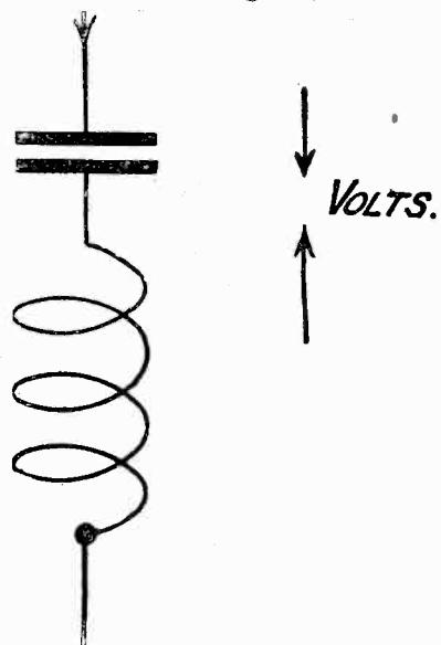
Fig. 3.—Relation of voltages produced across a coil and a condenser.
