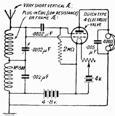
Fig. 4.—A single-control super-regenerative receiver.
