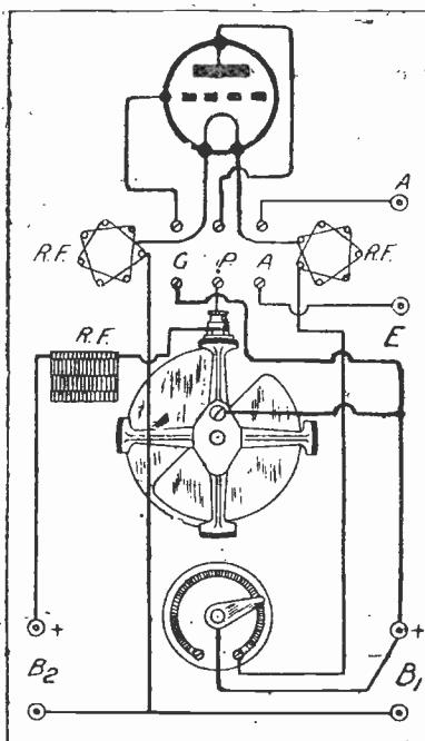
Fig. 1.—The back-of-panel layout of the 5-metre transmitter.
