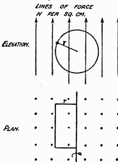
*Fig. 4.—Illustrating the method of rotating the coil for obtaining an expression for self-induction.*
