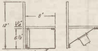
Fig. 5.—Details of the panel supporting brackets, showing manner in which the condenser C10 and grid cells are mounted.
