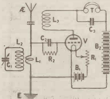
*Fig. 2.—In the case of a single valve the reaction coil L3 may be coupled to either  $L_1$  or  $L_2$ .*
