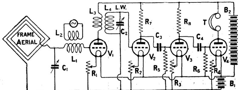
Fig. 2.—A supersonic heterodyne circuit with resistance coupling on the L.W. side, which may give the same distortion as in Fig. 1.
