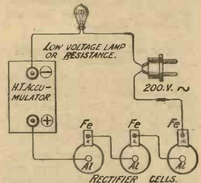
Fig. 4.—When charging H.T. accumulators up to 100 volts from 200v. A.C. mains, three rectifier cells are required.
