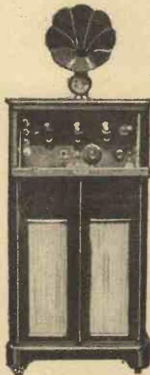
Mr. Bevan's arrangement of the "All Concert" receiver. The batteries are kept in the cupboard below.
