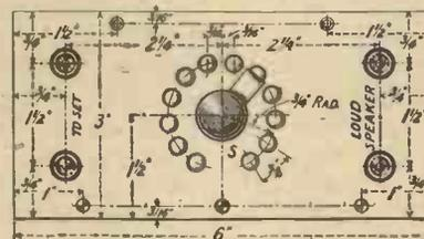
Fig. 2. Gives full dimensions for marking out the vertical panel.
