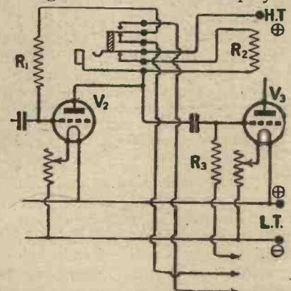
Fig. 2.—Using a jack to change grid-bias with H.T. voltage.
