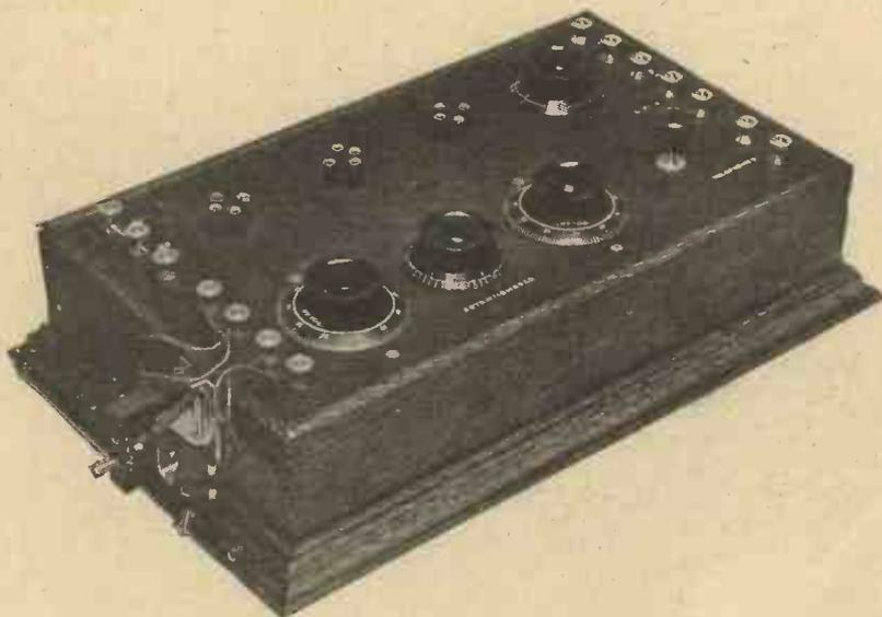
The well-balanced arrangement of the panel is clearly shown in this photograph. Note the connections to the coil-holder.
