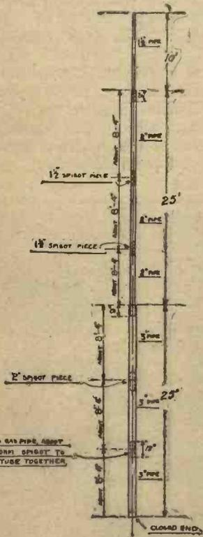
Fig. 1.—Illustrating how spigots are used for joining the larger tubes.
