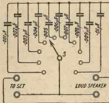
Fig. 1.—Shows the theoretical connections of the unit.
