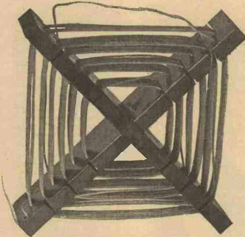
**Fig. 1.**—This type of coil is one in which moisture has little effect upon signal strength, and was the first coil upon which experiments were made.
