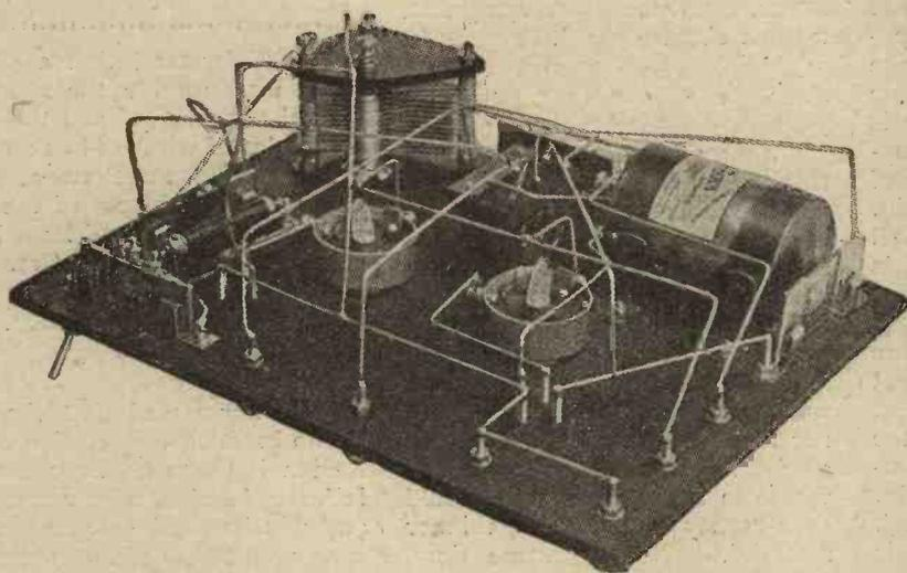
The layout of the receiver permits easy access to the components for wiring up.
