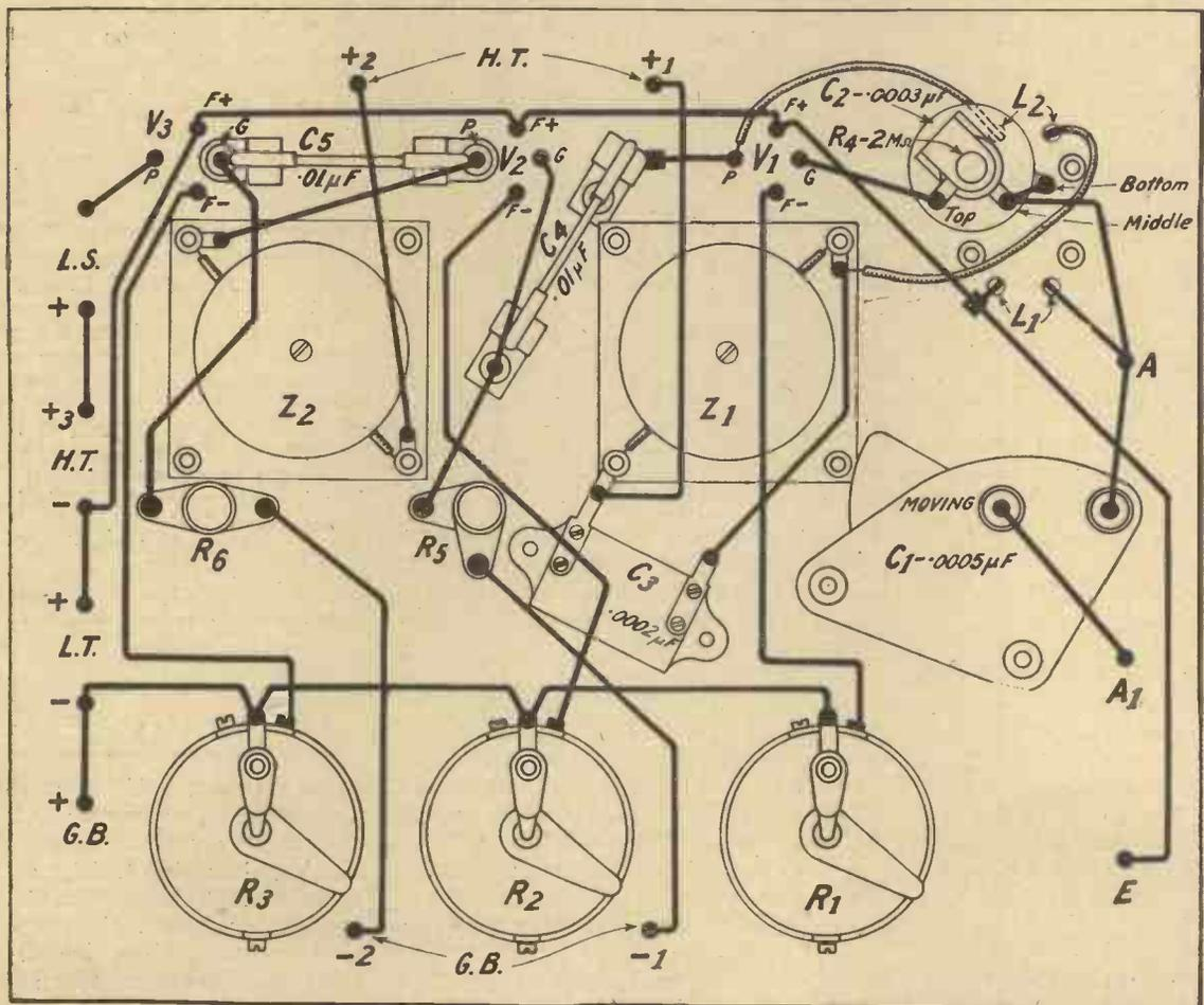
Fig. 3.—Practical back-of-panel wiring diagram. Note that the flexible reaction-coil leads are joined, one to the plate of V1 and the other to the choke coil Z1. Blueprint No. 119B.
