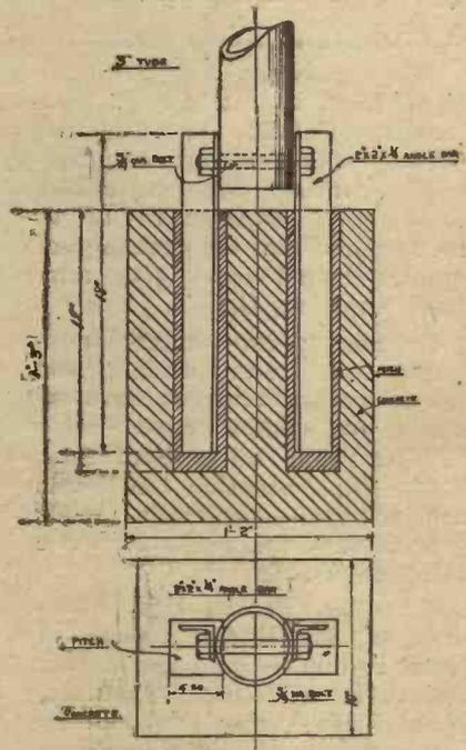
Fig. 3.—The fitting of a hinge to the base of the mast allows for easy lowering.
