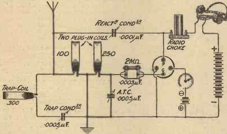
Fig. 3.—A semi-pictorial representation of the Fig. 2 arrangement.
