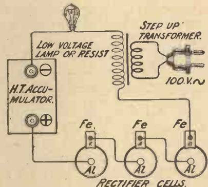
Fig. 5.—The apparatus and connections necessary for charging a 100v. H.T. accumulator from 100v. A.C. mains.
