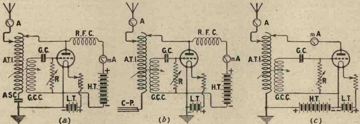
Circuit No. 3.—The magnetic reaction system.
