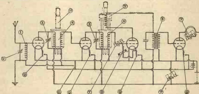
*Diagram of a Conventional 2 Stage H.F. 4 Valve Set. Showing use of **MB** H.F. Reactor and **MB** H.F. Damper. In a stable set the Reactor (5) shown should be used to give Reaction. Sets of this description, however, tend to oscillate of their own accord, in which case the **MB** H.F. Damper (10) should be used to give micrometer control, thus dispensing with the conventional potentiometer shown at (11).*
