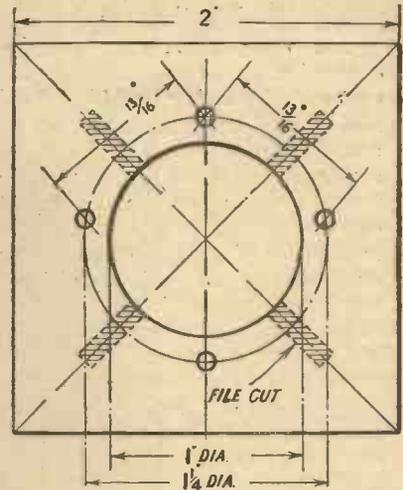
Fig. 2.—A drilling layout of the holder illustrated in Fig. 1.
