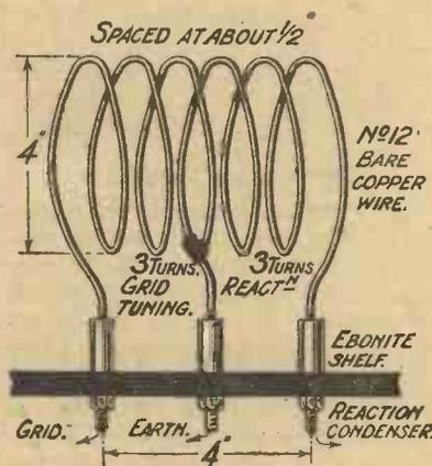
**Fig. 5.**—Mr. Cowper's original coil was wound with No. 12 gauge wire, but a slightly thinner gauge, such as No. 14, may be found easier to wind.
