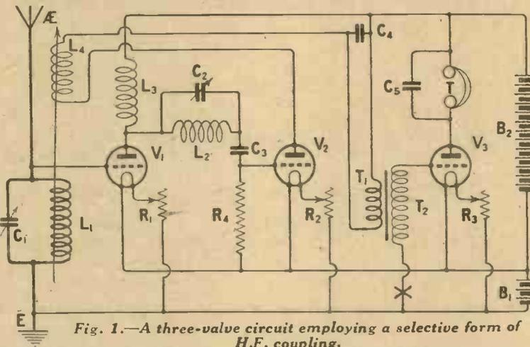
Fig. 1.—A three-valve circuit employing a selective form of H.F. coupling.
