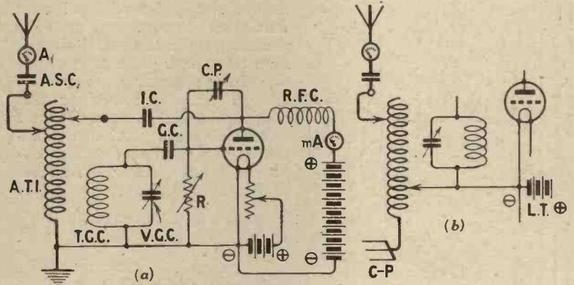
Circuit No. 4.—The tuned grid system.
