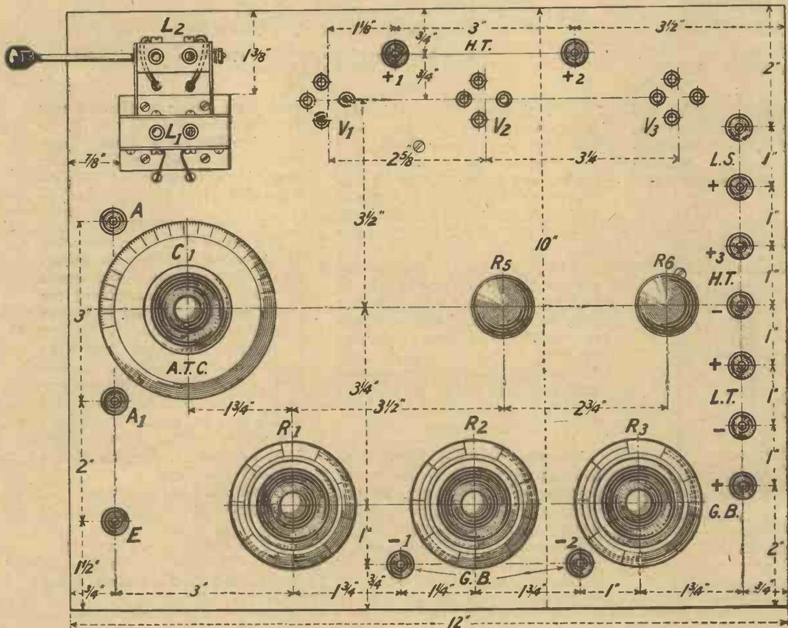
Fig. 2.—This layout of the panel showing all necessary dimensions may be obtained in Blueprint form upon quoting No. 119A.
