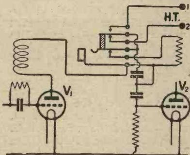
Fig. 1.—With this arrangement for switching in or out the resistance-coupled L.F. valve V2, a constant H.T. voltage may be maintained on the plate of V1.
