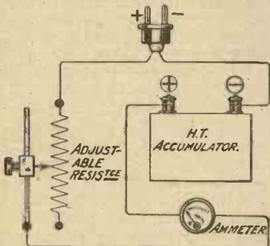
Fig. 1.—Showing the apparatus and connections necessary for charging H.T. accumulators from D.C. mains when a variable resistance is used.
