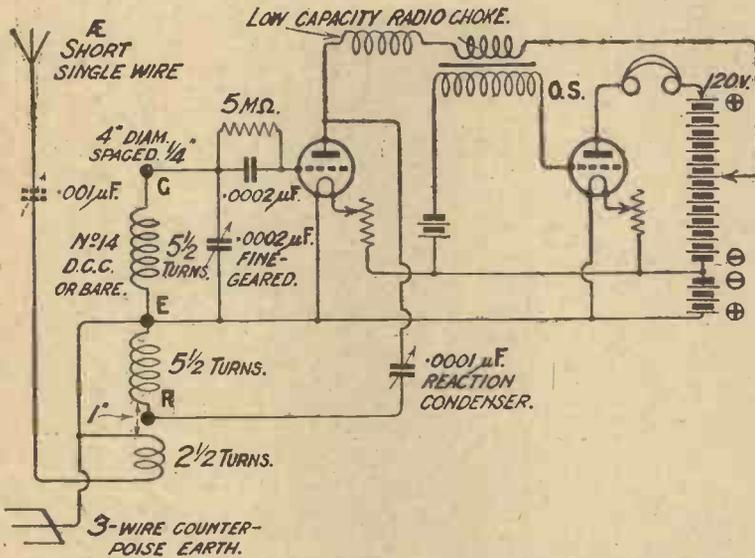
Fig. 3.—The complete circuit, showing the values for the 17 to 73 metres range.
