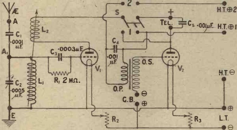
Fig. 1.—The theoretical circuit of the receiver.
