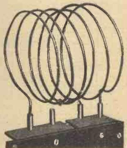
Fig. 4.—The coil with which Mr. Cowper succeeded in obtaining self-oscillation down to 9 metres.
