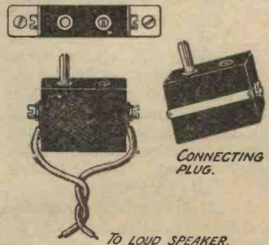
Fig. 3.—A suggested wall plug arrangement.
