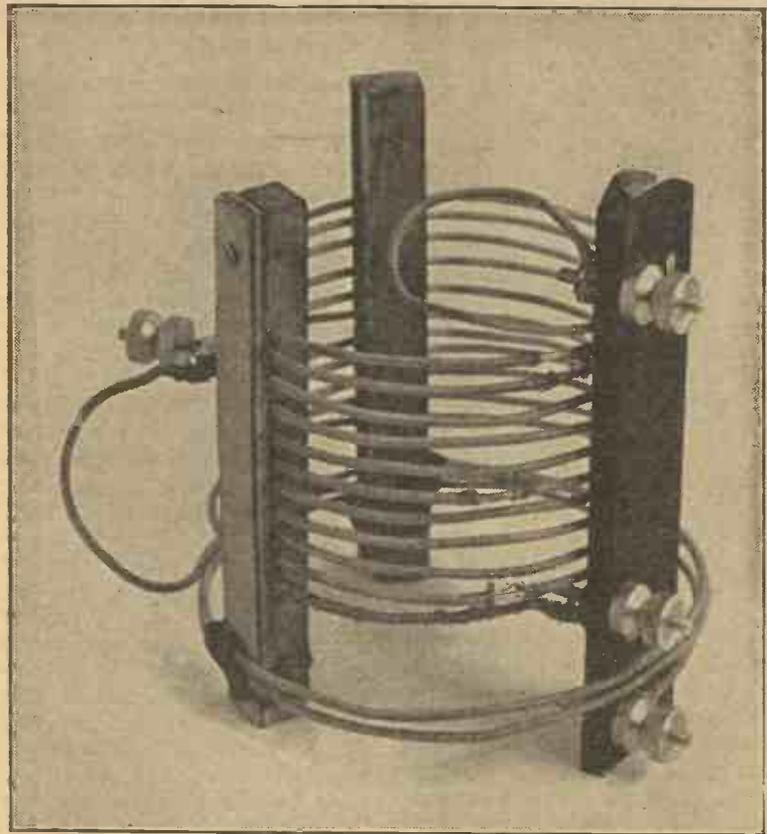
*The type of coil which Mr. Cowper first used in his experiments in short-wave reception.*
