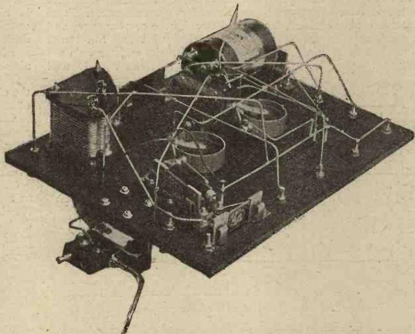
The connections to the coil holder and the grid leak unit may be clearly seen from this photograph.
