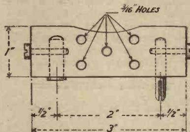
Fig. 2.—The dimensions of a coil-holder which is used by the author. the plug and the socket, but we want something better even than this for short-wave work.
