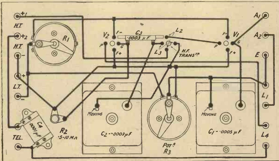
Fig. 3.—This practical back of panel wiring diagram may be used in conjunction with the photographs.
