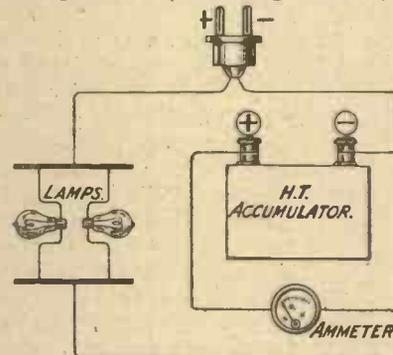
Fig. 2.—Charging H.T. accumulators from D.C. mains is also possible by using lamps in the circuit instead of the variable resistance shown in Fig. 1.
