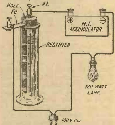
Fig. 3.—The simplest arrangement for charging H.T. accumulators up to 60 volts from 100v. A.C. mains. An ammeter in series with the battery is advisable in this and in the other circuits given.
