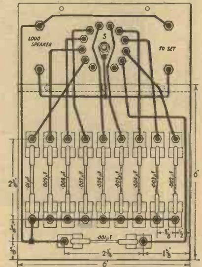
Fig. 3.—In this wiring diagram dimensions are also given for marking out the horizontal panel.
