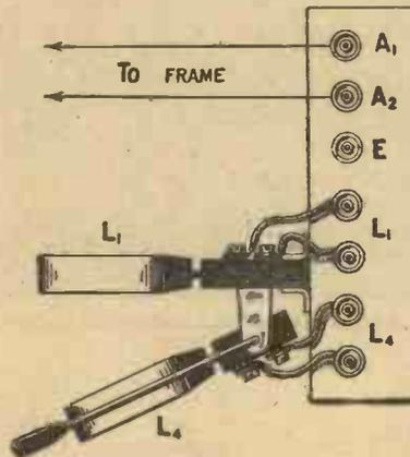
Fig. 1a.—The connections when using the frame aerial.
