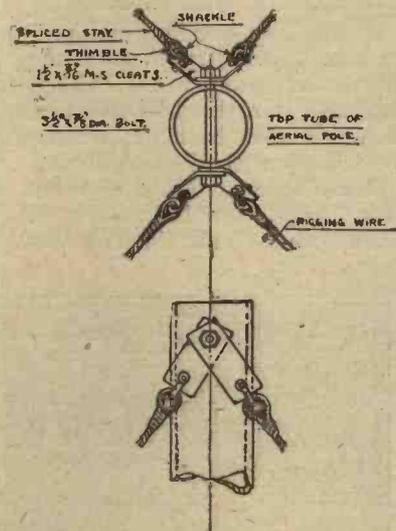
Fig. 2.—Showing how stays may be attached to the mast if desired.
