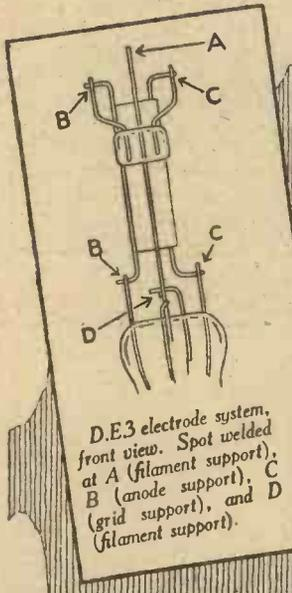
D.E.3 electrode system, front view. Spot welded at A (filament support), B (anode support), C (grid support), and D (filament support).
