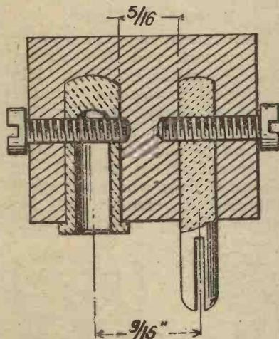
Fig. 1.—A section of a coil socket showing the construction.
