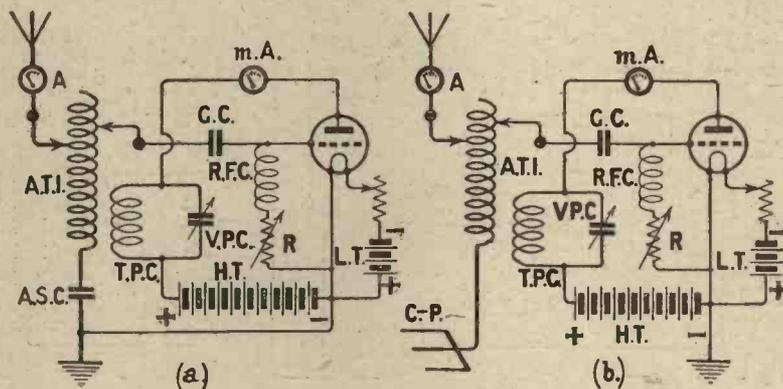
Circuit No. 6. The tuned plate system.
