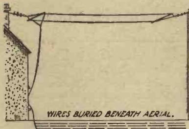
Fig. 2. — Another good earth consists of buried wires beneath the aerial.
