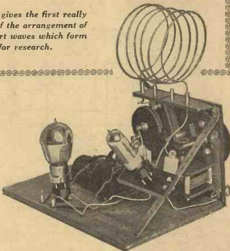
The radio choke may be seen immediately below the coil in this view.
