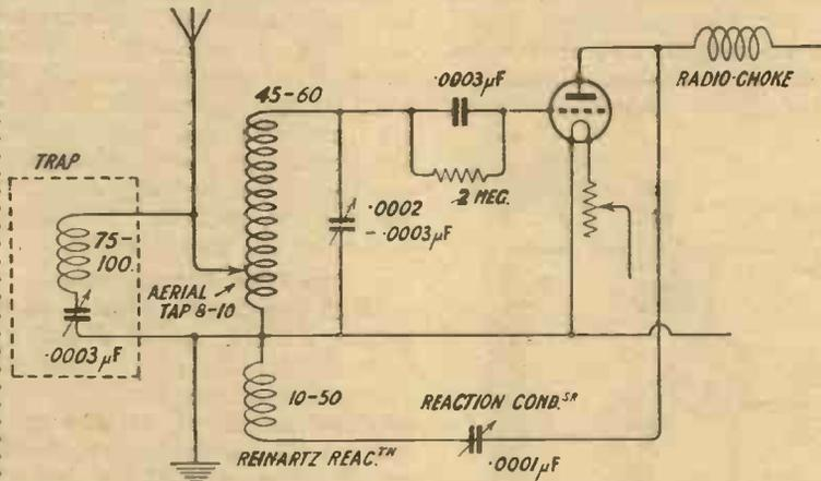
Fig. 1.—The tuning arrangements, together with values for use upon the 300-600 metres wavelength band.
