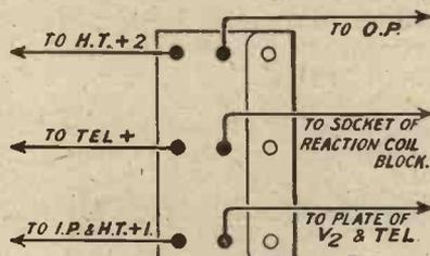
Fig. 3.—The connections to the switch.
