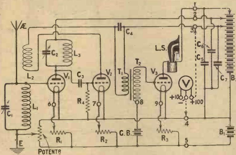
Fig. 1.—In this circuit the numbered points indicate where the voltmeter should be connected for various readings as described in the text.
