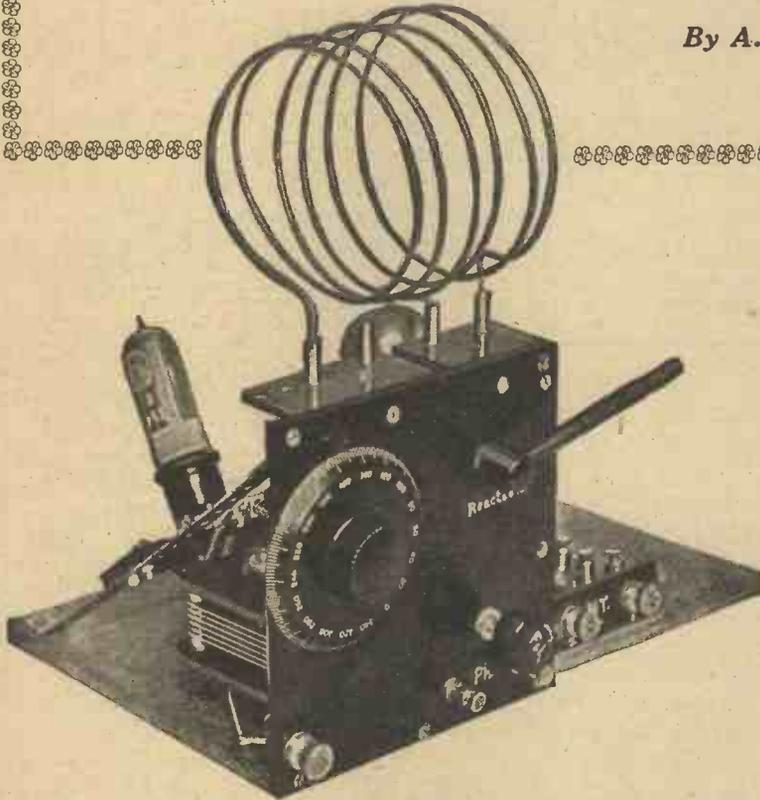
The detector valve is mounted in such a way that the critical leads are extremely short.
