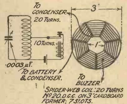
Fig. 1.—The buzzer wavemeter arrangements.
