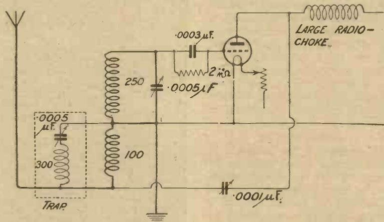
Fig. 2.—The trap applied to an ordinary Reinartz tuner, using plug-in coils, permits the successful reception of Radio Paris without interference from 5XX.
