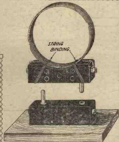
Fig. 3.—Illustrating how the coil may be mounted.
