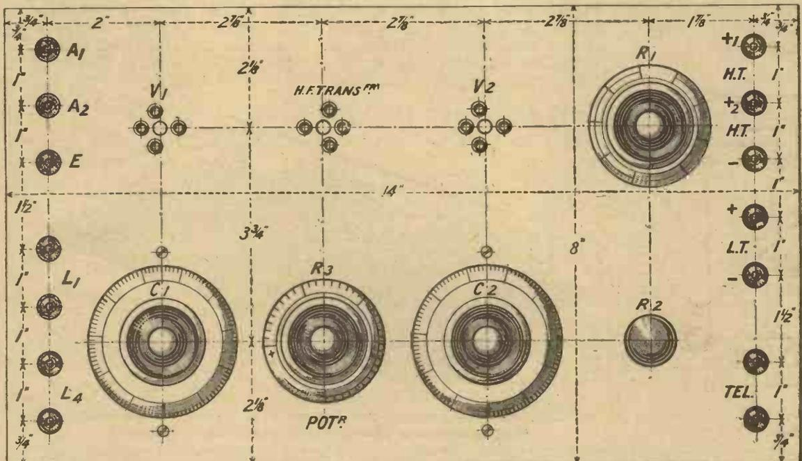
Fig. 2.—A practical drilling diagram and panel layout giving all necessary dimensions.
