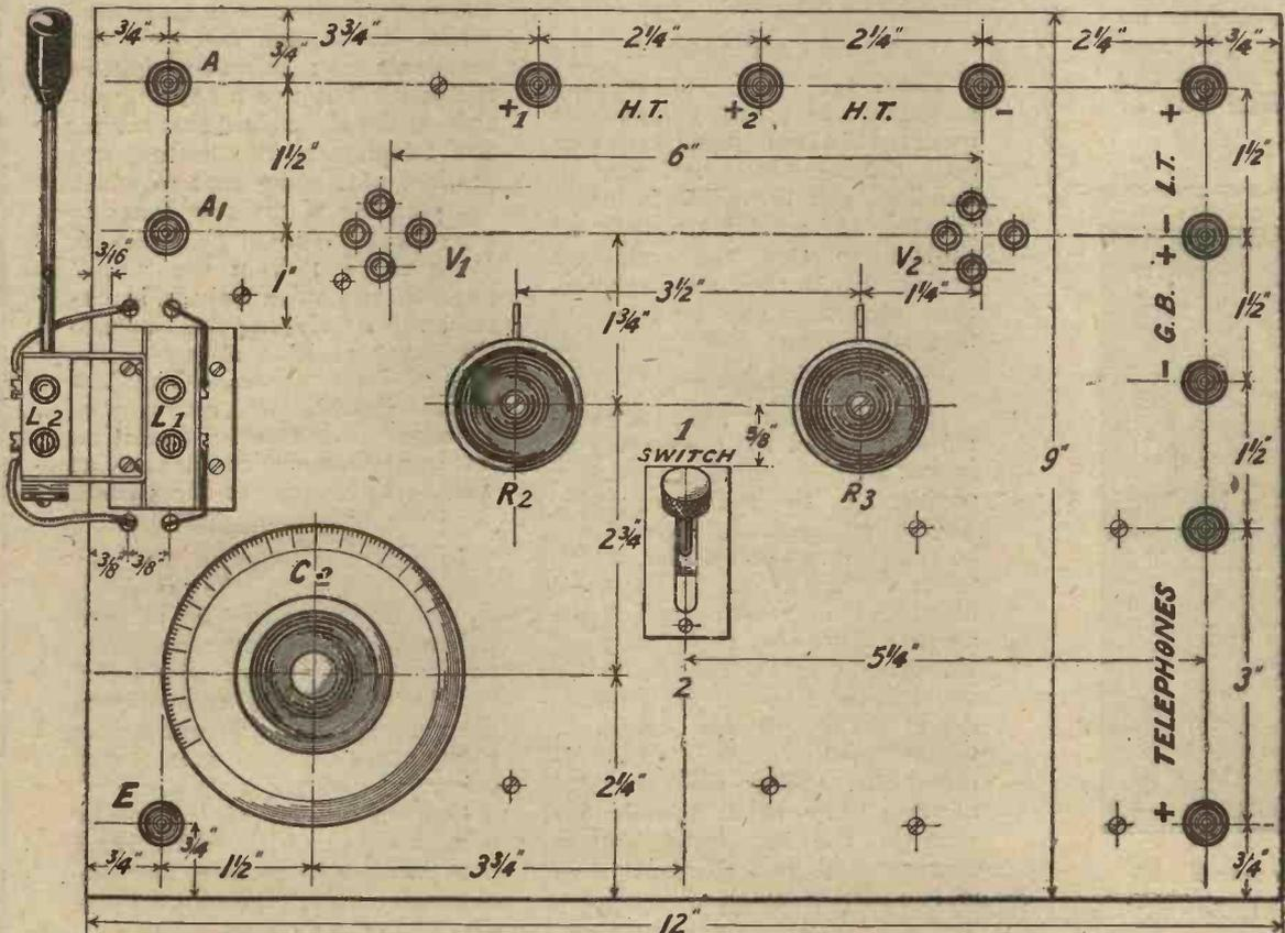
Fig. 2.—Drilling dimensions and all details relating to the layout of the panel may be obtained from this illustration.
