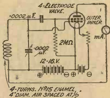
Fig. 2.—The wavemeter circuit used by the author for ultra-short waves.
