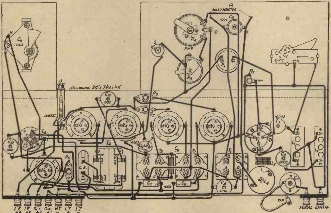
Fig. 3.—Certain parts of the wiring are here shown outside the limits of the baseboard for clearness' sake.
