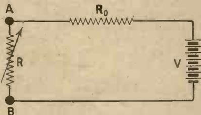
Fig. 1 (A).—In this circuit  $R_0$  represents the "resistance" of the valve.
