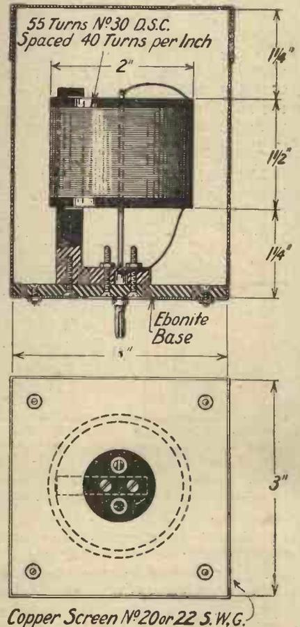
Fig. 5.—Constructional details of the new coil.
