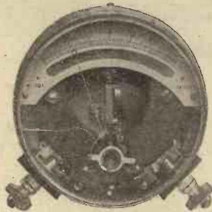
A micro-ammeter is required to indicate the change in anode current of the oscillating valve.
