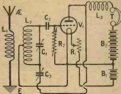
Fig. 1.—Reaction effects are obtained by adjustment of C3, without affecting seriously the setting of C1.
