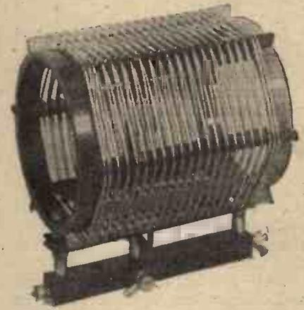
*A commercial version of the skeleton-supported air-spaced coil.*
