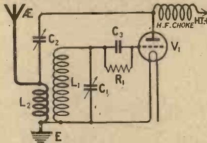
Fig. 5.—When coils of fairly low resistance are used it is possible to use a combined aerial and reaction winding.
