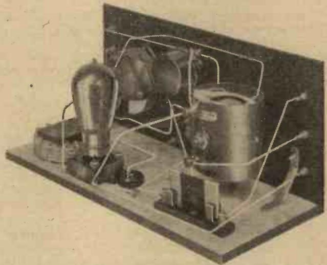
This receiver (described by Mr. G. P. Kendall in March, 1926, issue of the "Wireless Constructor") illustrates one method of applying reaction to a variometer. (Note the hank coil in one end of the tube.)
