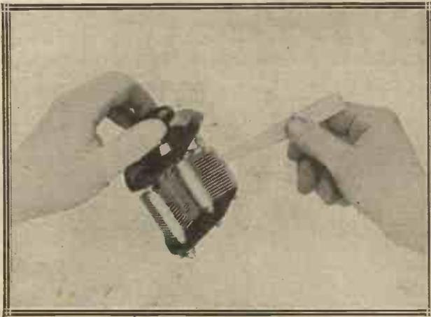
ONE of the most annoying difficulties connected with short-wave reception is to be found in the fact that so many variable condensers make objectionable grating and crackling noises when the set is oscillating upon these high frequencies. It is not alone upon the high frequencies, however, that condensers are apt to give rise to troublesome noises.
