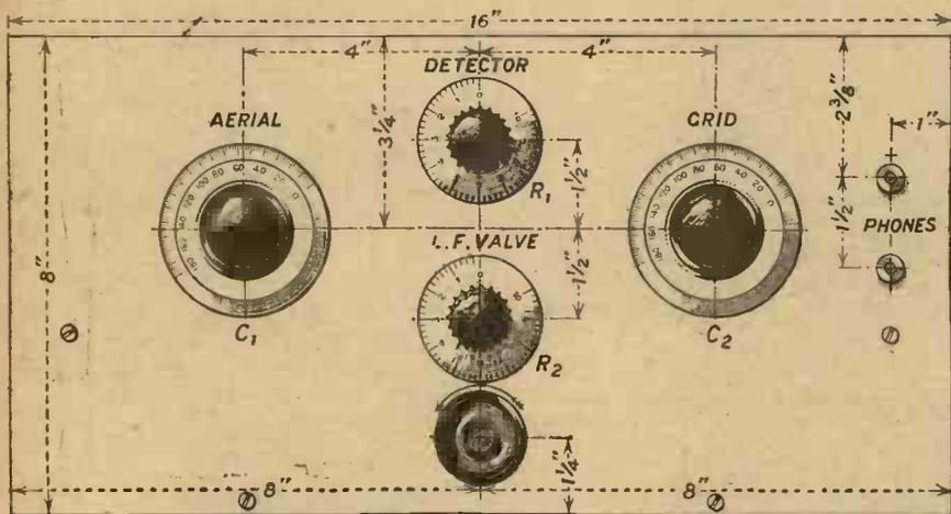
*Fig. 2.—In laying out the panel the positions of the bracket screws will depend on the make of bracket used.*
