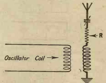
Fig. 4.—The method can be applied to the measurement of aerial resistance.
