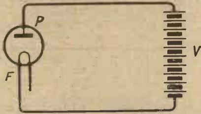
Fig. 3.—With a two-electrode valve current will only flow in one direction.
