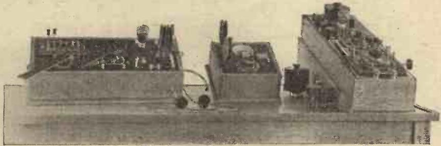
Left to right are the subsidiary oscillator, the quartz control unit, and the wavemeter itself.
