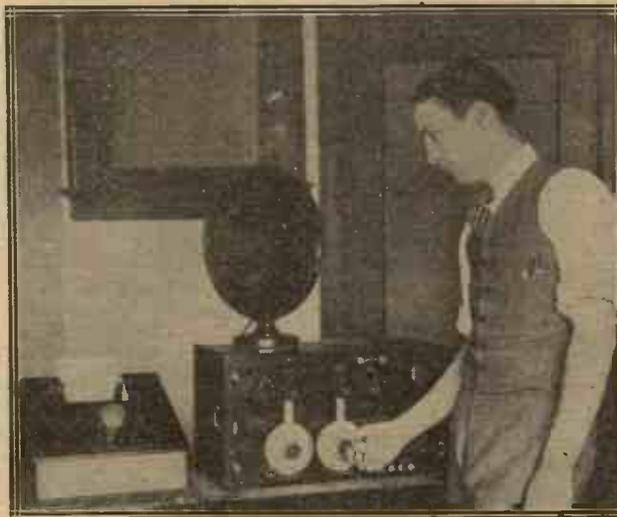
One of the foremost experimenters in radio television in America is C. F. Jenkins, of Washington, whose latest invention is seen here. It is an apparatus which reproduces by means of a travelling pen the handwriting transmitted from a distant station.
