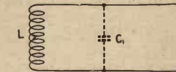
**Fig. 1.**—The self-capacity of a coil can be regarded for practical purposes as a condenser of definite value in parallel with the coil.
