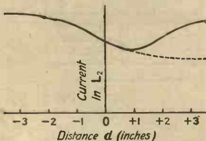
Fig. 3.—The introduction of a single screen between the coils was not found adequate.
