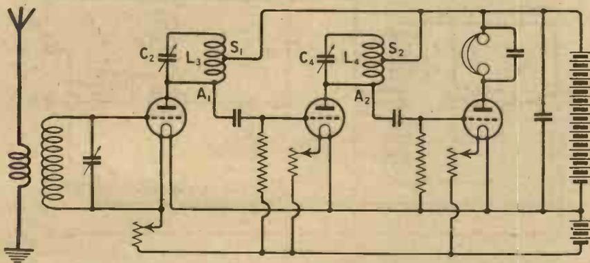
Fig. 3.—Taking the tapplings S1 and S2 from slightly different points upon the coils L3 and L4 will overcome the tendency to parasitic oscillations, with little effect on oscillation at the main frequency.
