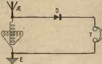
*Fig. 1.—In even the simplest circuit the variation of tuning by means of a variometer produces quite different effects from those of a condenser method.*
