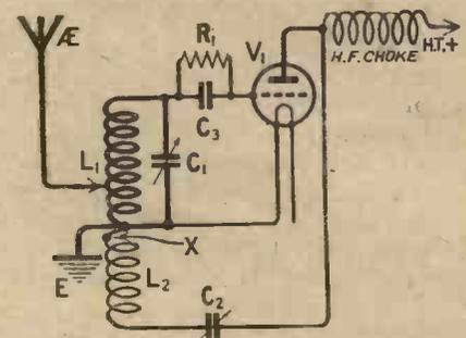
Fig. 6.—Auto-coupling is sometimes used to enable the reaction condenser to be inserted at the point X, but this is not advised.
