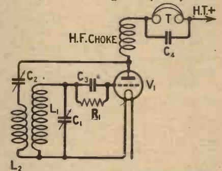
Fig. 3.—Better results are obtained by including a choke in series with the 'phones.
