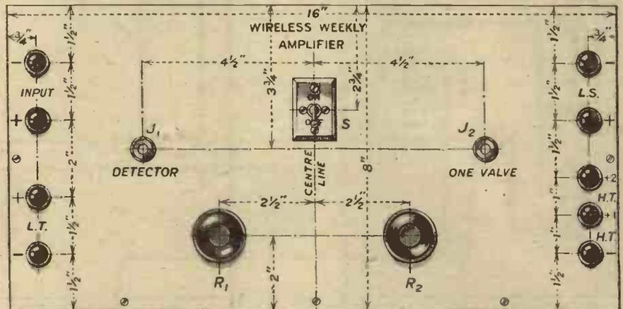
Fig. 2.—The lettering of the jacks corresponds to that in the circuit diagram.
