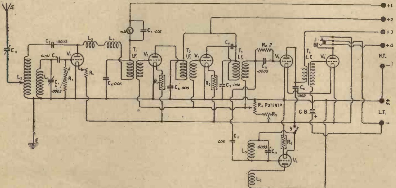
Fig. 1.—The condenser in the aerial circuit is of the small neutrodyne type, while  $C_8$  is supplied with the intermediate transformers.
