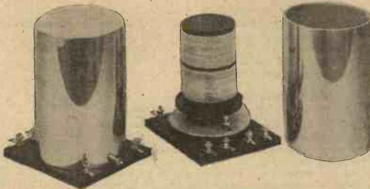
This view shows how the coil is located inside the screen in the Peto-Scott form.
