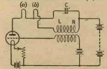
Fig. 4.—The oscillatory circuit used in the experiments from which the photographic records were obtained.
