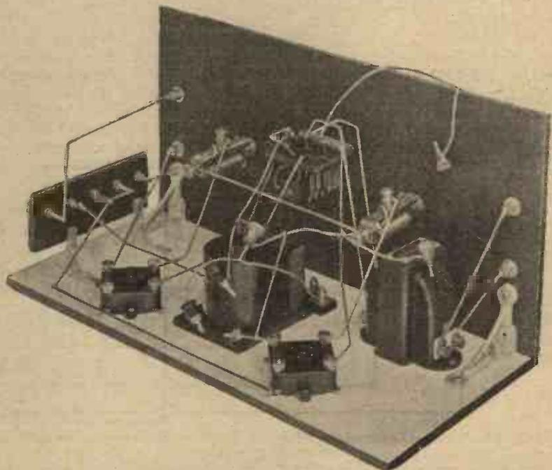
An expedient sometimes adopted to secure stability is to use different methods of coupling between successive stages.
