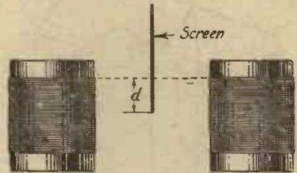
Fig. 2.—The effect of introducing a single shield between the coils to a distance "d" was investigated, and the result is expressed in Fig. 3.
