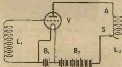
*Fig. 2.—A simplified version of Fig. 1, including only the parts of the circuit responsible for the subsidiary oscillations.*
