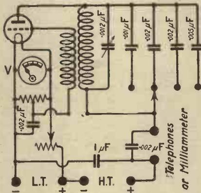
Fig. 1.—The main oscillating circuit.
