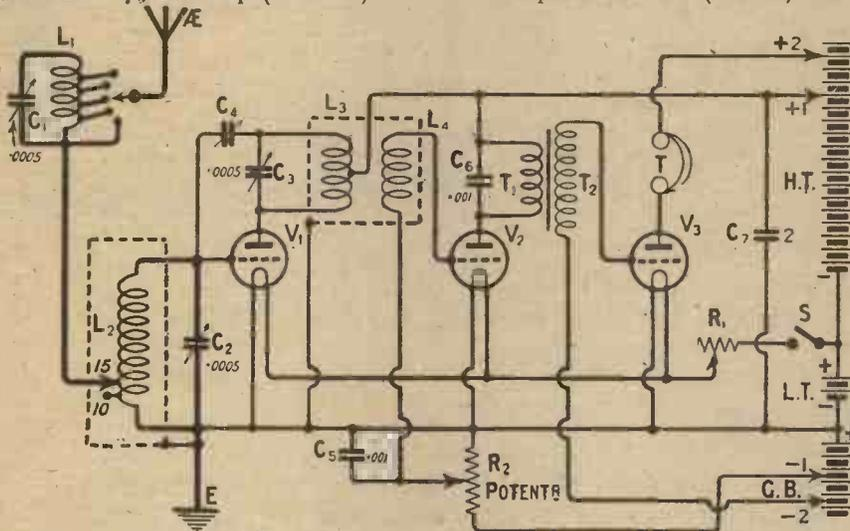
Fig. 1.—The dotted lines represent the shields, which are connected to earth.
