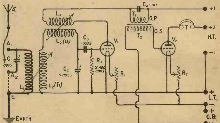
Fig. 1.—The circuit is quite a typical "split-secondary" arrangement. The aerial condenser may be used in series or parallel.
