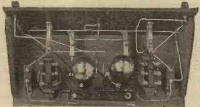
L.S. terminals will be put into action in the anode circuit of the second low-frequency valve.
