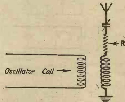
Fig. 4.—The method can be applied to the measurement of aerial resistance.
