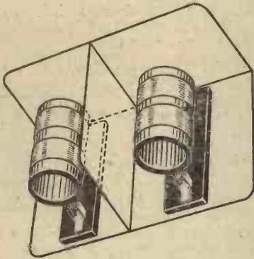
Fig. 4.—This method of partial screening gave a reduction of 60 per cent. in the amount of energy transferred.
