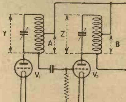
Fig. 4.—The essential portion of Fig. 3, redrawn to indicate the relationship between the portions A and B of the two anode coils.
