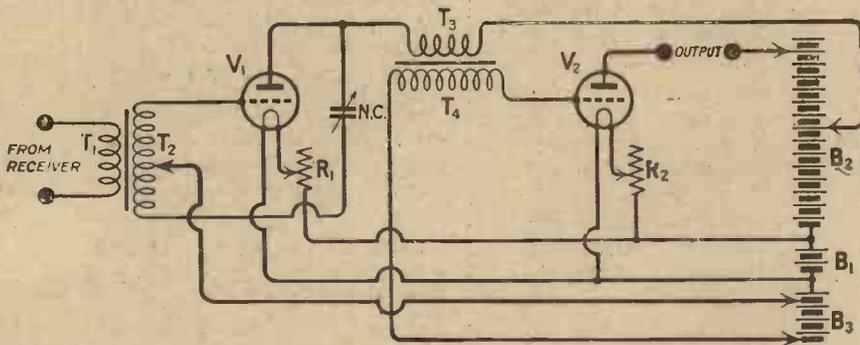
Fig. 4.—The use of a tapped transformer is indicated here in the grid circuit of the first valve.
