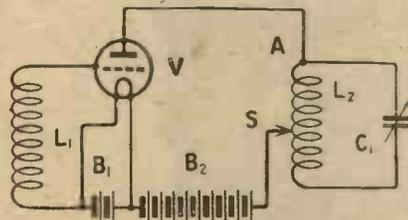
*Fig. 1.—This type of circuit is prone to produce oscillations at a frequency distinct from the main frequency.*
