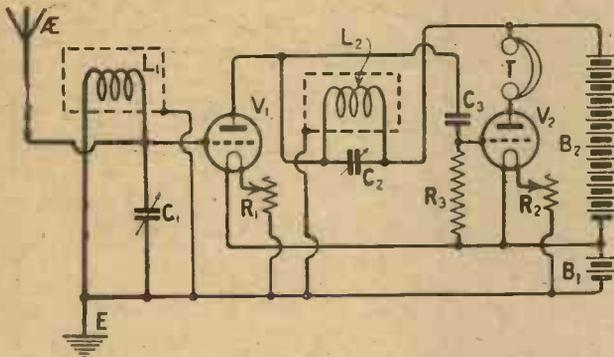
Fig. 1.—Screened coils gave a perceptible improvement in even this simple circuit.
