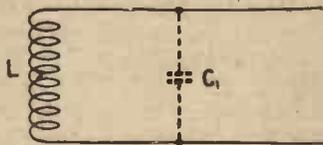
*Fig. 1.—The self-capacity of a coil can be regarded for practical purposes as a condenser of definite value in parallel with the coil.*
