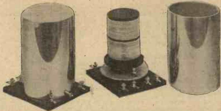
This view shows how the coil is located inside the screen in the Peto-Scott form.
