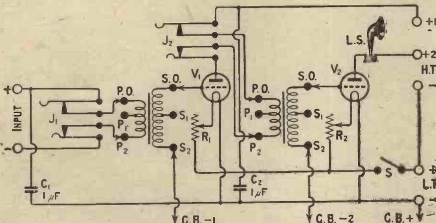
Fig. 1.—Plugs and jacks are provided to permit telephones to be used with one note-magnifying valve and to enable them to be connected directly to the input.
