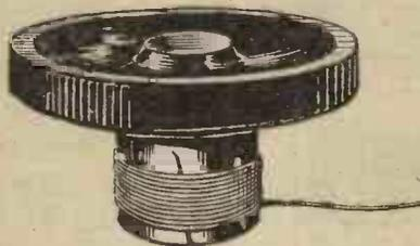
*In winding the wire it should be kept as tight as possible.*
