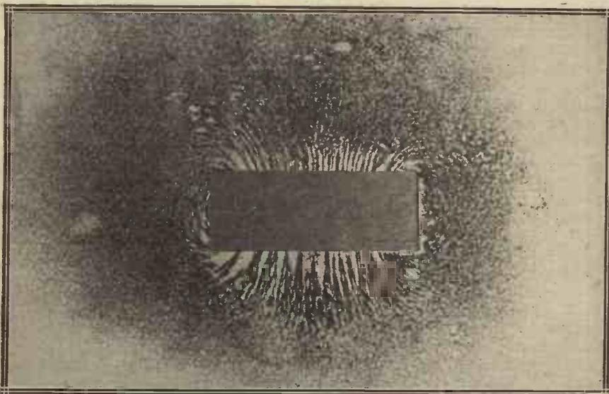
*The field of coil B was determined by the iron filings method.*
