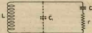
Fig. 3.—The self-capacity of the coil may give rise to notable errors if it is comparable to the capacity C.
