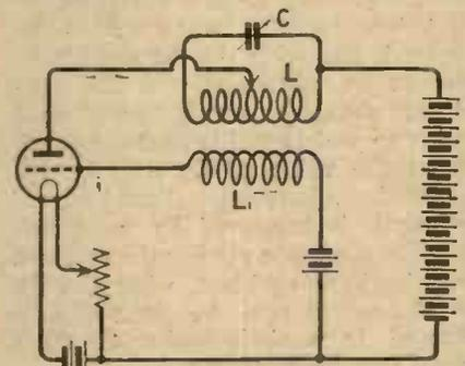
*Fig. 2.—The use of an anode tap makes possible an adjustment for the maximum oscillatory current without alteration of the coupling.*
