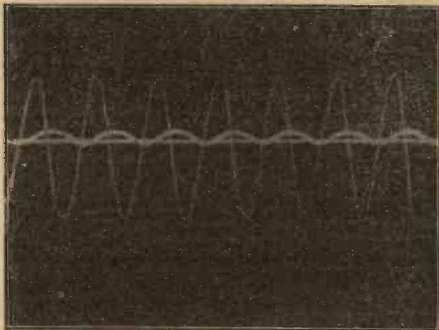
photographs, the oscillator in question being essentially designed for low frequencies, the lowest value reached being 150 cycles per second. To meet this necessity the untuned grid coil was wound to give an inductance (air-core) of over 3 henries.
