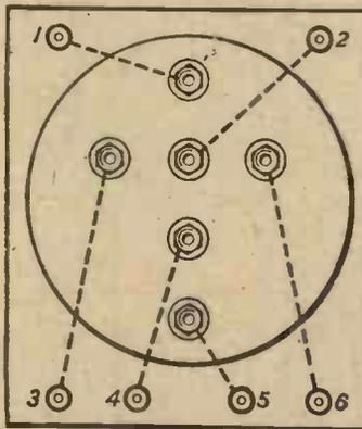
Fig. 4.—The standard connections of the coil base.
