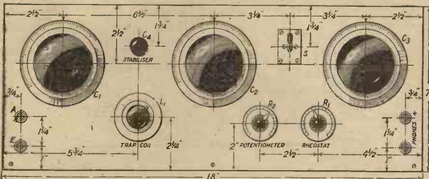
Fig. 2.—The panel lay-out gives a very convenient arrangement of controls.
