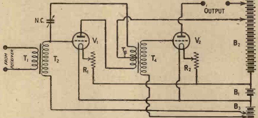
Fig. 3.—A centre-tapped or similar L.F. transformer is needed in this circuit.
