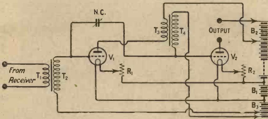
Fig 1.—A simple scheme resembling the Hazeltine neutrodyne arrangement.
