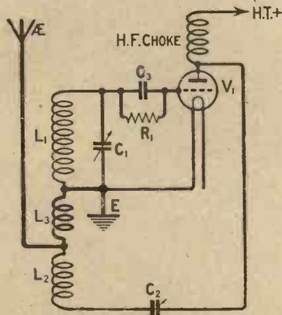
Fig. 4.—In the first Reinartz circuits two windings ( $L_2$  and  $L_3$ ) were provided for reaction and aerial coupling.
