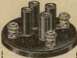
"Duco" Type "D" Valve Holder for Baseboard mounting. One of the Insulated valve sockets which screw into base of solid ebonite is coloured red to indicate Anode, thus offering protection against incorrect insertion of valve. Nickel-plated connecting tags are carried to terminals. Two screws only are required for mounting.
