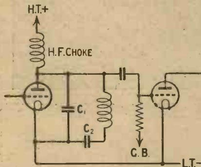
**Fig. 1.**—The circuit arrangement used at Rugby to filter out unwanted harmonics.
