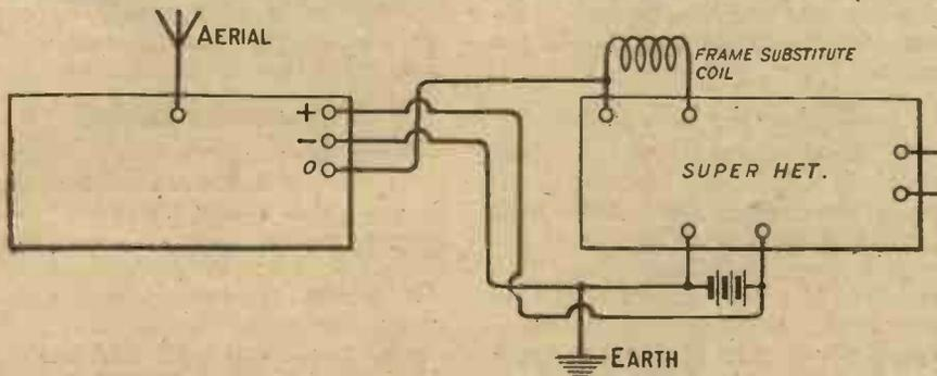
Fig. 3.—When the adapter is used with a superheterodyne the aerial and earth connections are as shown here.
