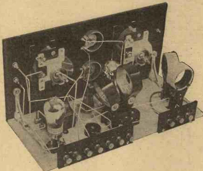
*The aerial and secondary coupling coils are adjusted in position by swivelling their mounts.*
