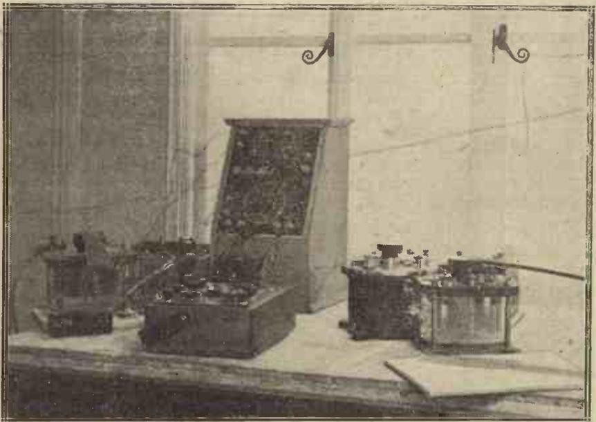
A view of the actual apparatus used at Elstree for measuring H.F. resistance.
