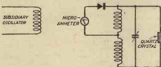
Fig. 2.—The frequency of the subsidiary oscillator is checked by means of a crystal control circuit.
