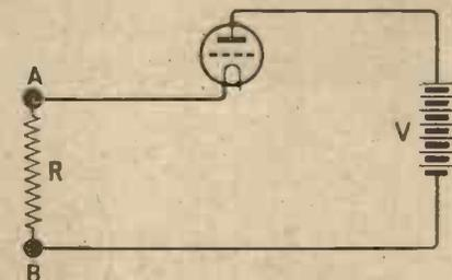
Fig. 1 (B).—Here the valve and external resistance are shown in their correct relationship. Compare with Fig. 1 (A).
