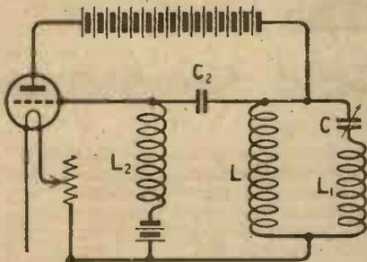
Fig. 3.—This circuit incorporates most of the features met with in practical reaction circuits.
