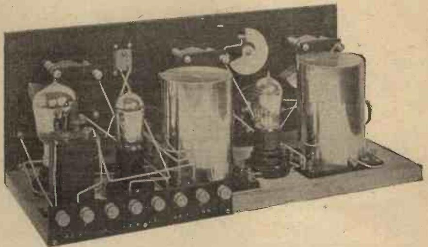
The use of screened coils permits the set to be made very compact.
