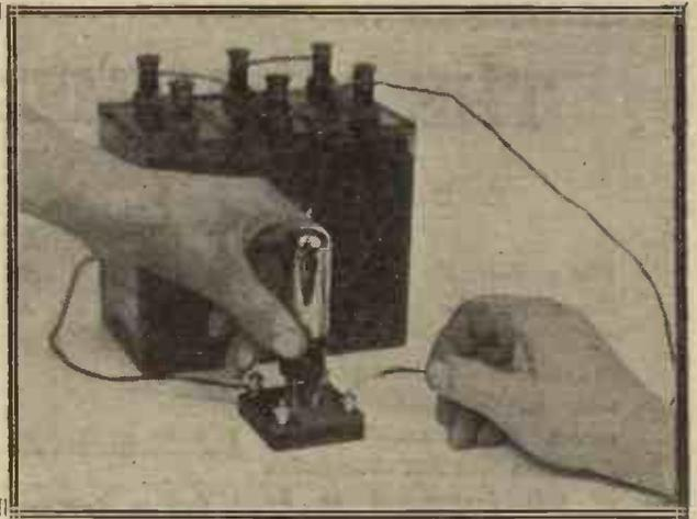
**M**ANY experimenters who have graduated in the bright-emitter school do not fully realise that although the filament of a dull-emitter valve may be continuous and appear to light correctly, the valve may nevertheless have lost its emission and be practically useless whilst in that condition.
