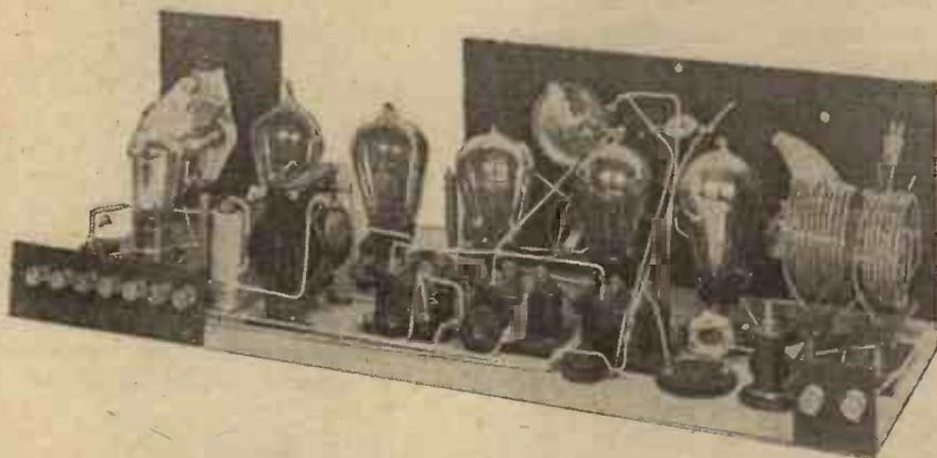
This view shows how the aerial lead from the series condenser is attached to the appropriate tapping point on L2.
