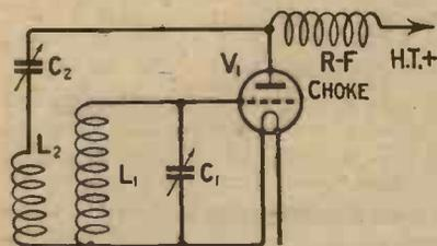
Fig. 1.—The reaction circuit provides a parallel path to filament for the H.F. component of the anode current.
