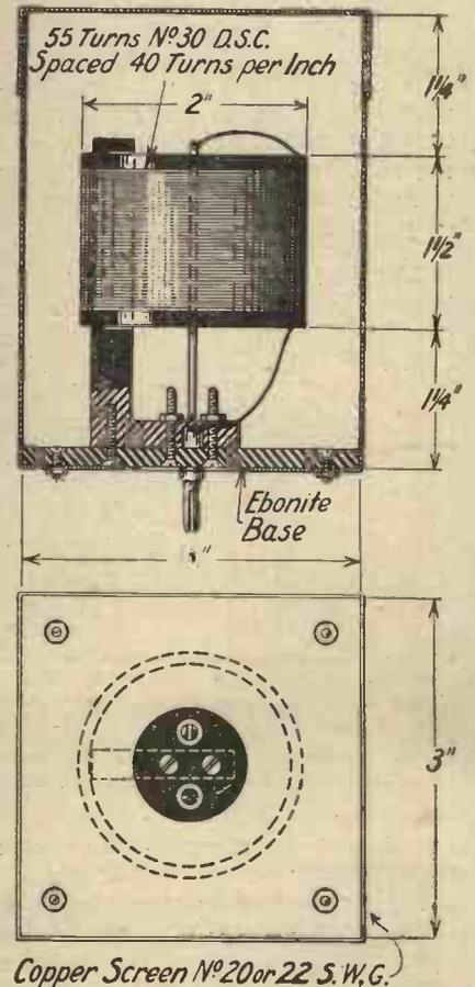
Fig. 5.—Constructional details of the new coil.
