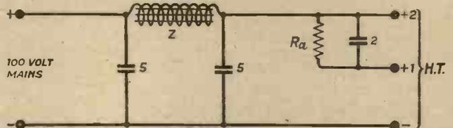
The negative side of the mains is joined directly to the high-tension negative terminal of the receiver, whilst the positive side is connected through a high-impedance choke coil Z, which may be one of the chokes normally employed in an ordinary choke-coupled
