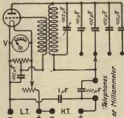
Fig. 1.—The main oscillating circuit.
