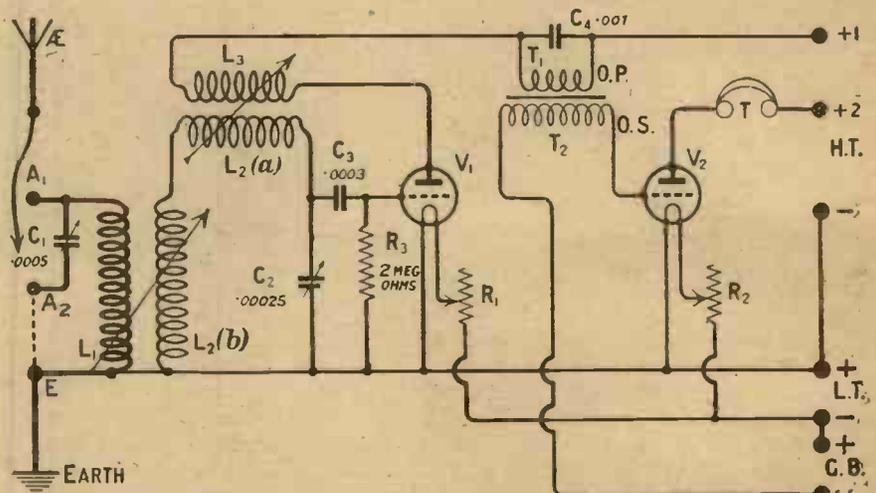
Fig. 1.—The circuit is quite a typical "split-secondary" arrangement. The aerial condenser may be used in series or parallel.
