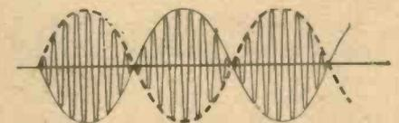
*Fig. 3.—When the permanent field (Fig. 2) is zero, the current takes the form shown here.*
