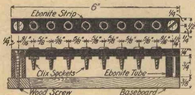
Fig. 4.—The sets of Clix sockets are mounted on strips of ebonite.
