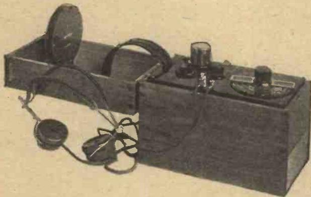
*The buzzer type of wavemeter is much easier to use with a superheterodyne than one of the heterodyne type.*
