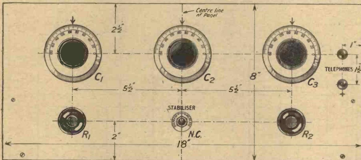
Fig. 3.—The lay-out of the panel is particularly neatly balanced.
