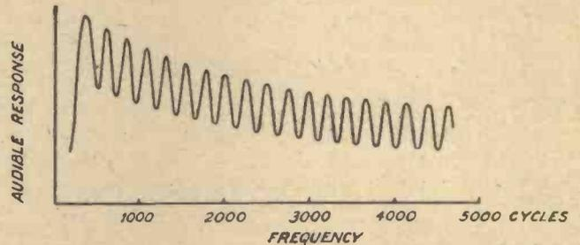
Now for some of the difficulties which meet the constructor: they are usually of two types, a rattling noise with loud notes and pronounced resonance at a certain high note. The rattling noise is due to looseness of some part of the paper, usually at the centre, and careful construction is the only cure. Dust getting into the centre is also said to cause rattling, and should be blown out with a bellows periodically.
