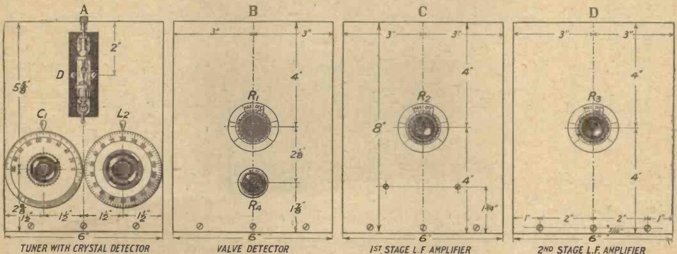
**Fig. 1.**—The panels are all of the same dimensions and there is very little drilling to be done.
