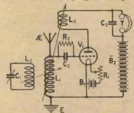
Fig. 4.—This circuit shows how that of Fig. 3 would be arranged if separate coils were used for the various functions.
