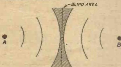
Fig. 1.—Interference may produce "dead spots" between two stations working on the same frequency.
