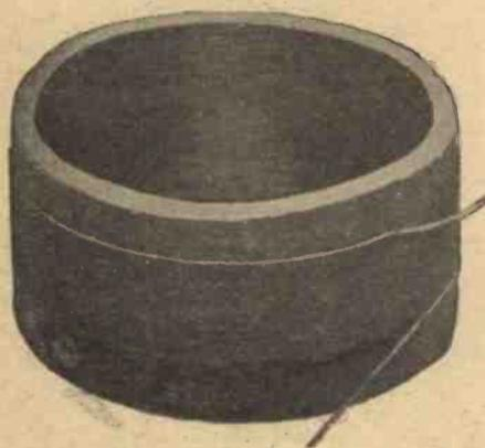
Large diameter relative to winding length is a factor for low H.F. resistance for a given frequency.
