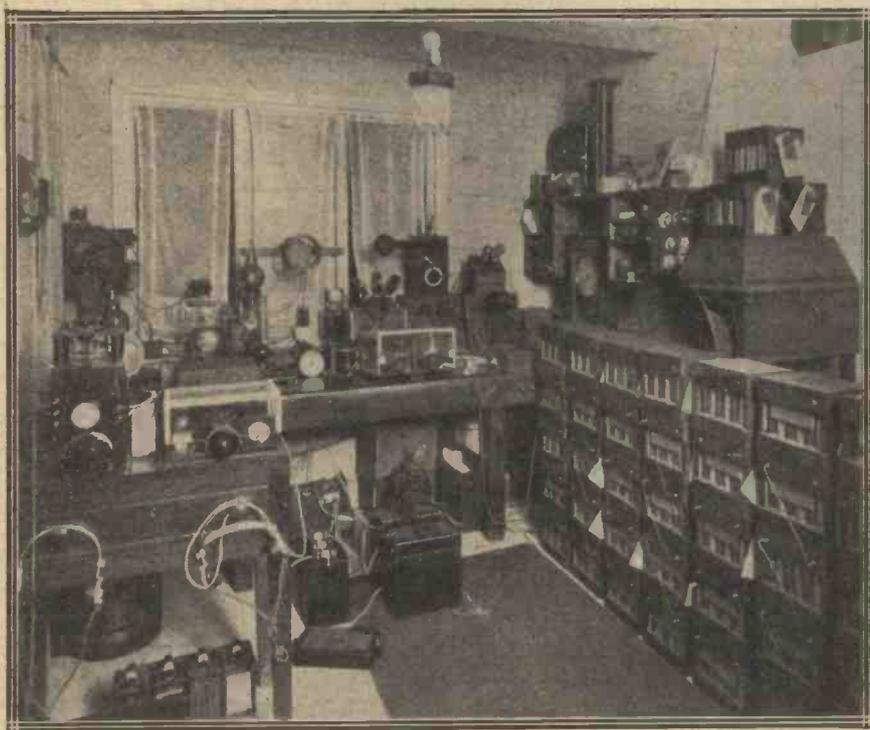
Much important short-wave experimental work has been done by amateurs, and their position in regard to key patents is clearly defined. This is one of the latest views of "2OD," showing a 1,500-volt bank of C.A.V. accumulators used in some recent experiments with Australia. An increase of 25% was reported on switching over from rectified A.C. to the pure D.C. supply.
