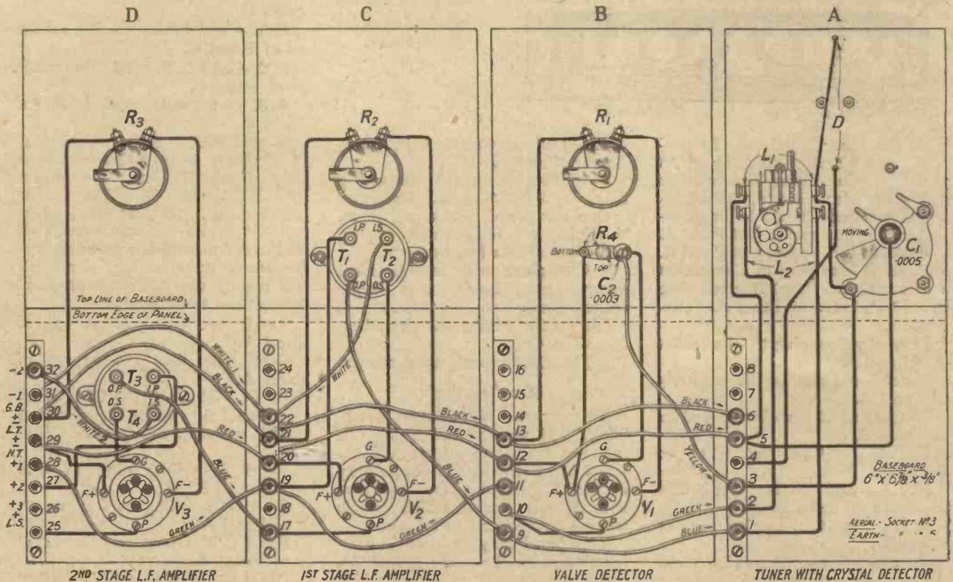
Fig. 3.—Stiff wire is used for the permanent connections and flex for the links between the units.
