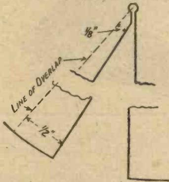
Fig. 6.—In cutting the gap allow an overlap like this.
