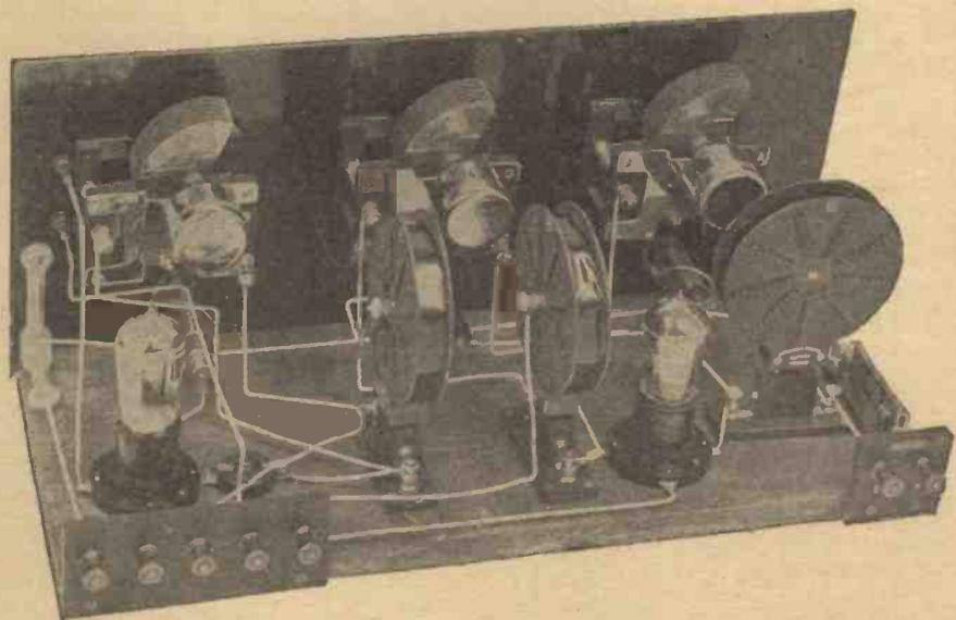
The two coils shown parallel to each other are the ones forming the H.F. transformer. For good selectivity they will usually require to be placed almost at right angles.
