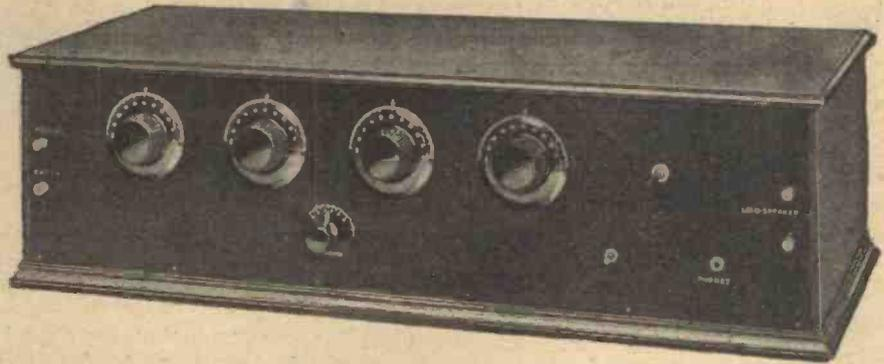
Anode bend rectification is employed in the "Remarkable Five-Valve Receiver," with which loud-speaker results of excellent quality have been obtained from a large number of broadcasting stations.
