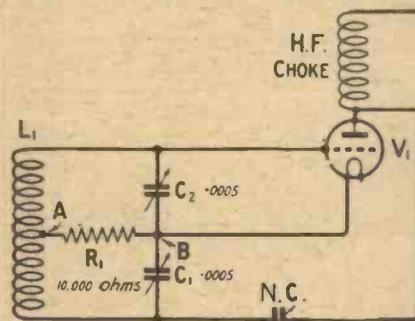
Fig. 1.—Illustrating the split-condenser method of neutralisation.
