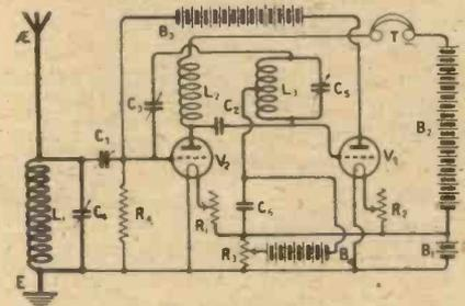
In the article "Reflexing the Prince Circuit" in last week's issue of "Wireless Weekly," Fig. 4 on page 316 was incorrectly shown, the battery B4 being wrongly connected. This diagram is correctly reproduced herewith.
