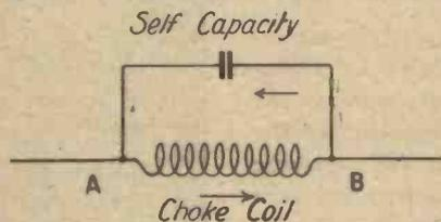
Fig. 2.—The inductance of the choke and its self-capacity may provide an actual reflector circuit.
