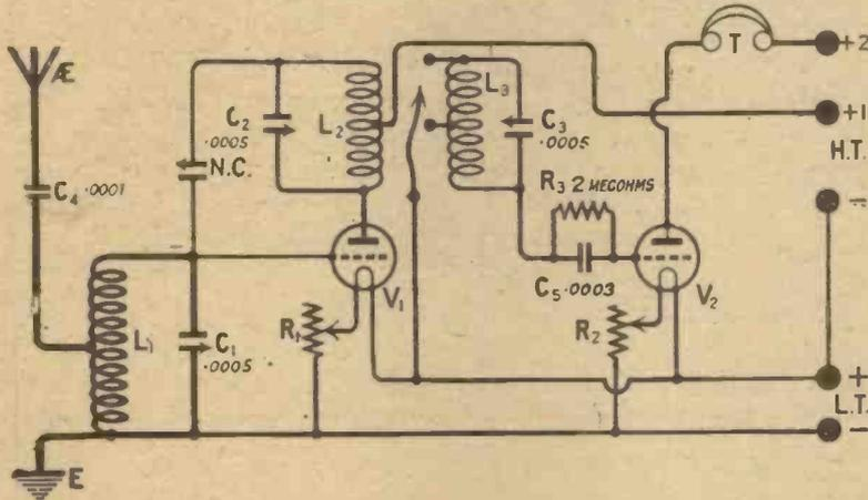
Fig. 1.—In the circuit adopted for this set the coils L2 and L3 constitute the interval transformer. The degree of coupling between them must be adjusted with some care.
