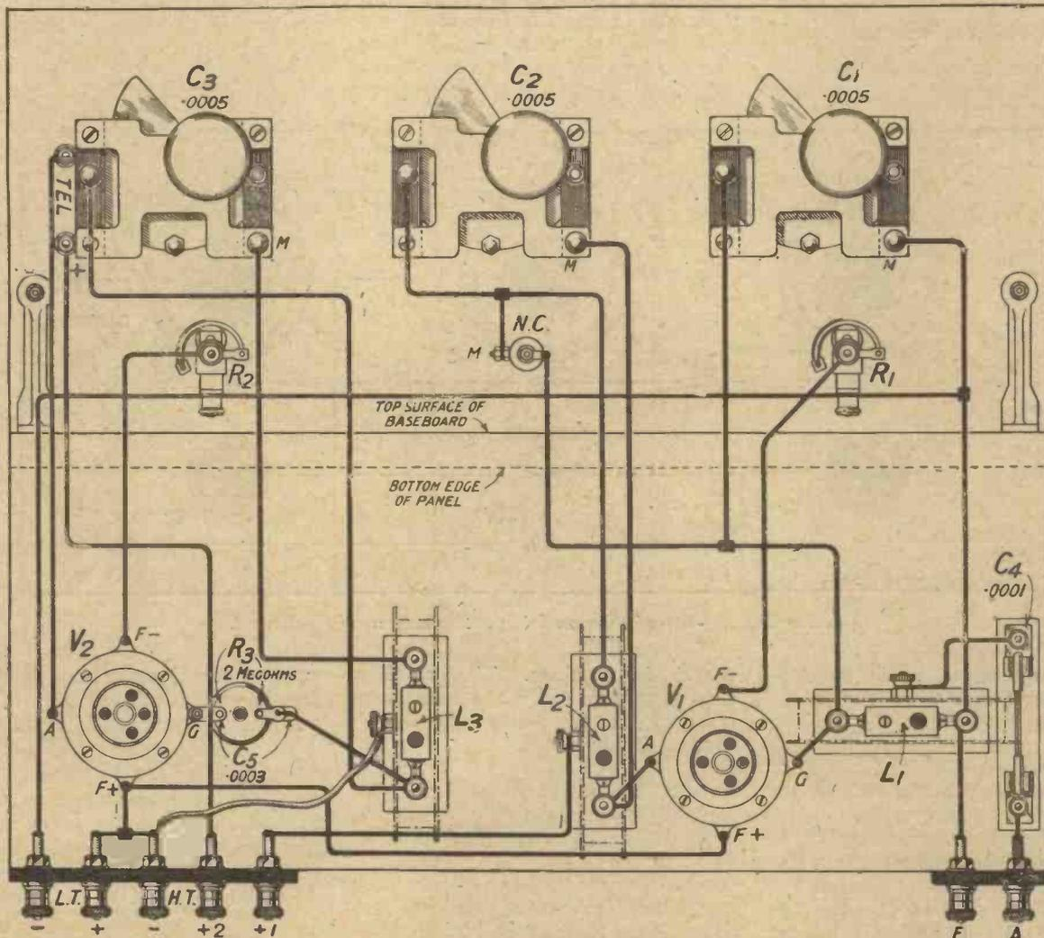
Fig. 2.—In wiring the set it is recommended that the leads to the coil  $L_3$  should be done with  $\text{flex.}$
