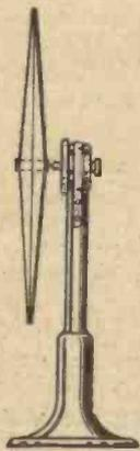
Fig. 3.—The diaphragm and its actuating mechanism can be mounted upon some sort of pedestal.
