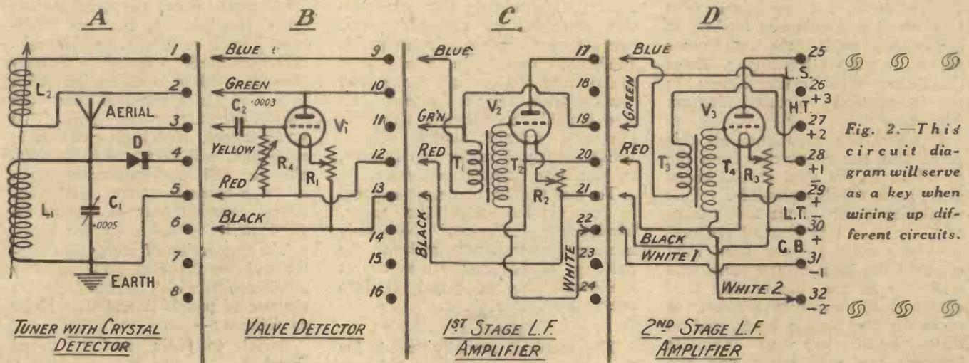
Fig. 2.—This circuit diagram will serve as a key when wiring up different circuits.
