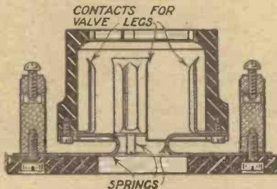
An anti-microphonic valve-holder of good workmanship, made by Messrs. The Norman Radio Co., Ltd.
