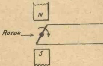
*Fig. 1.—In a simple alternator, revolution of the rotor in the magnet field produces an alternating current voltage.*
