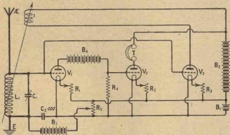
Fig. 3.—Reaction can be obtained by adding a special valve (V3) for the purpose.
