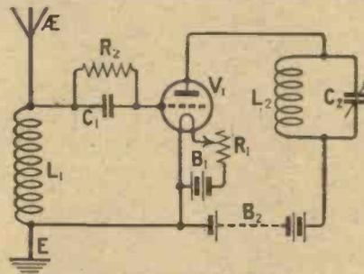
Fig. 3.—This circuit employs a form of trap tuning, by virtue of the coupling which is provided in practice between L1 and L2 (again shown separated here).
