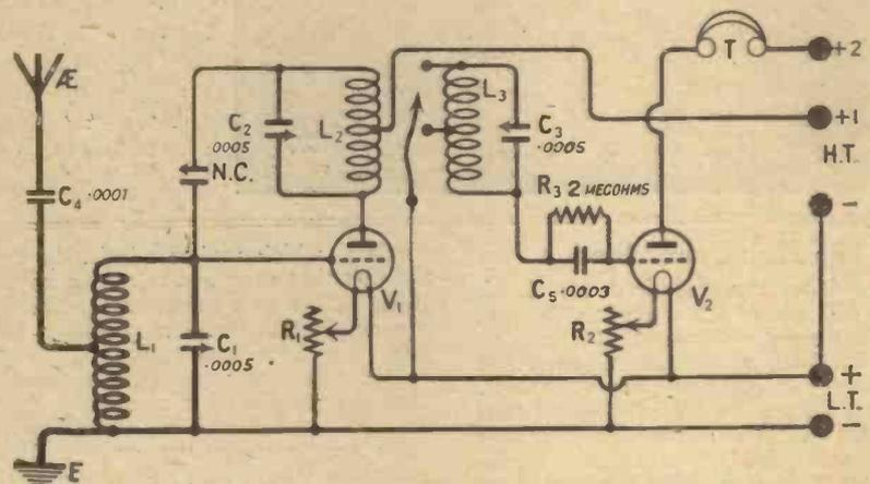
The circuit is repeated for reference purposes. Note that L<sub>3</sub> is the movable coil.
