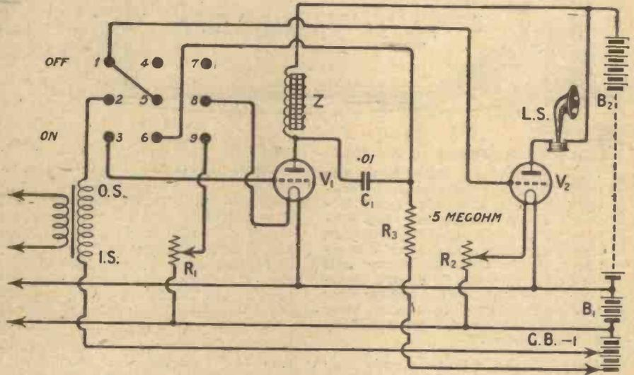
Fig. 1.— This arrangement allows of the valve V<sub>2</sub> being in circuit whether one or two stages of L.F. amplification are used.
