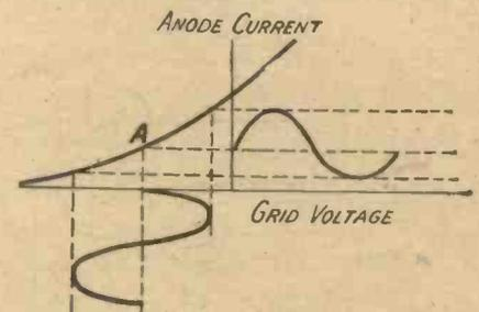
*Fig. 1.—With the anode current method rectification takes place owing to asymmetrical variations in the current.*
