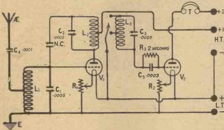
Fig. 1.—In the circuit adopted for this set the coils L2 and L3 constitute the intervalve transformer. The degree of coupling between them must be adjusted with some care.
