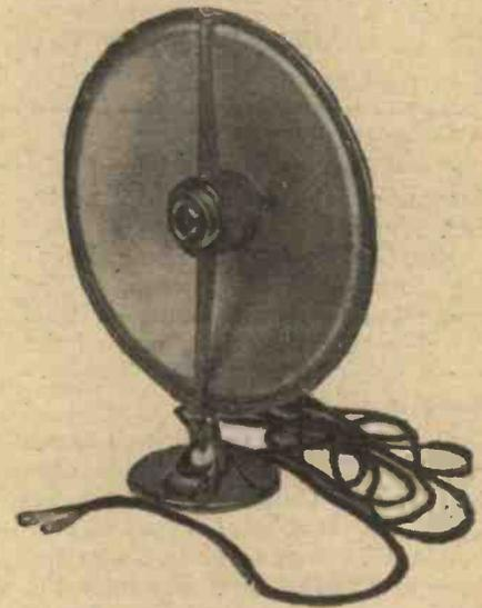
A commercial version of a single-cone loud-speaker (this a "Sferavox," the other commercial instrument illustrated in the heading of this article being a "Kone").
