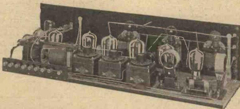
*One of the attractions of the superheterodyne is that although it contains many tuned circuits, a number of them are permanently adjusted to a fixed frequency, and do not require manipulation. In this set, for example, three circuits are provided with tuning condensers which could be located inside the receiver, where they can be set once and for all.*
