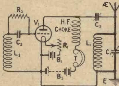
Fig. 6.—A form of reaction used in the Reinartz circuit is shown here.
