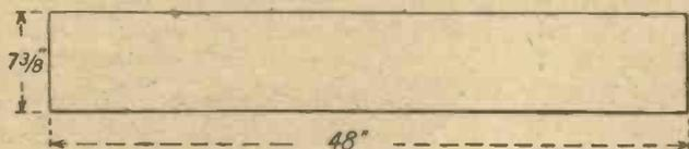
*Fig. 1.—These are the dimensions for a strip of paper from which a pleated diaphragm can be made.*
