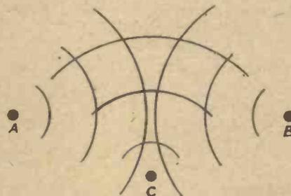
Fig. 2.—The provision of a number of stations would ensure that such interference effects as might occur would not produce blind areas.
