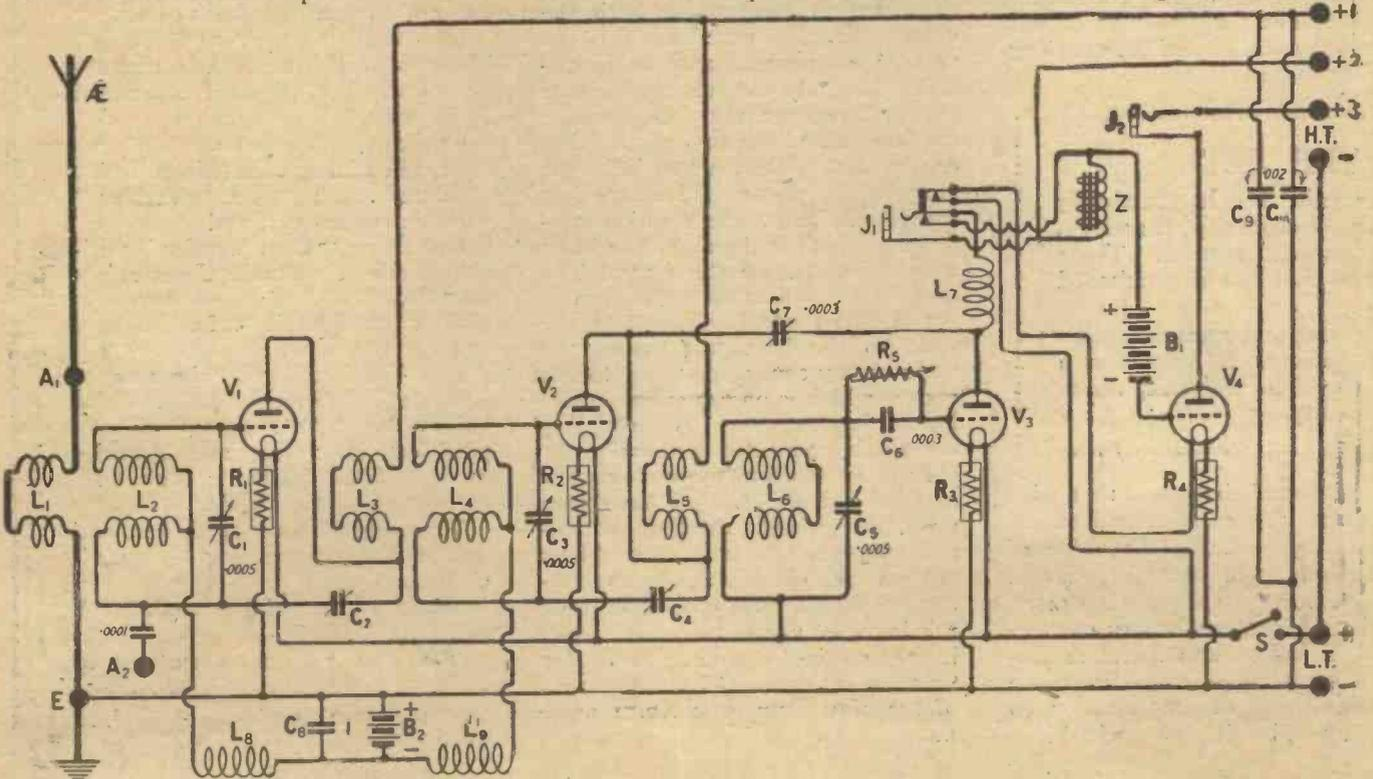
Fig. 2.—A slightly simplified version of the circuit. The terminal A2 permits the aerial to be auto-coupled.
