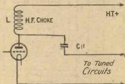
Fig. 3.—It is becoming quite a common practice to separate the oscillatory component of the anode current from the steady current.
