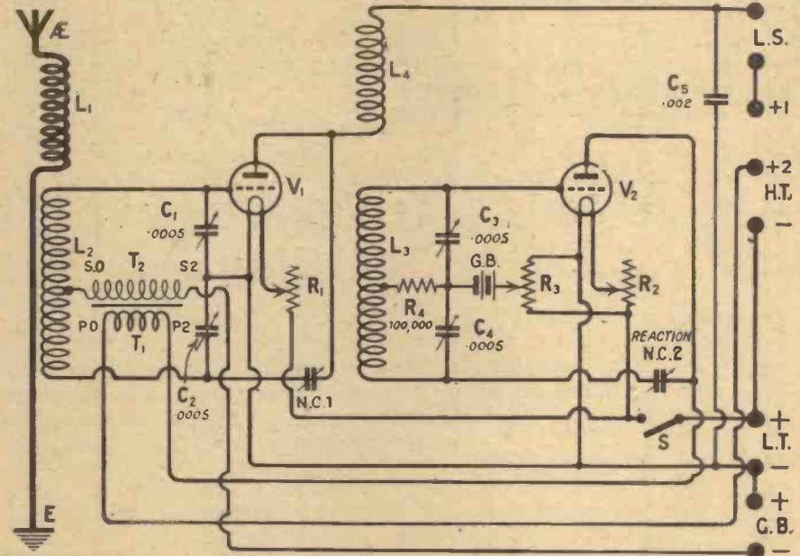
Fig. 2.—Anode bend rectification is employed, reaction control being provided by means of the condenser NC.2.
