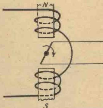
*Fig. 2.—The addition of an alternating field to the alternator of Fig. 1 will produce modulations of the current generated.*
