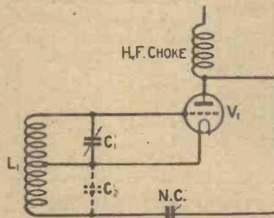
Fig. 2.—If only half the coil is tuned trouble may be produced by the self-capacity of the untuned portion.
