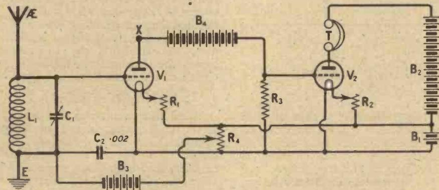
Fig. 1.—A conventional example of the trigger circuit.
