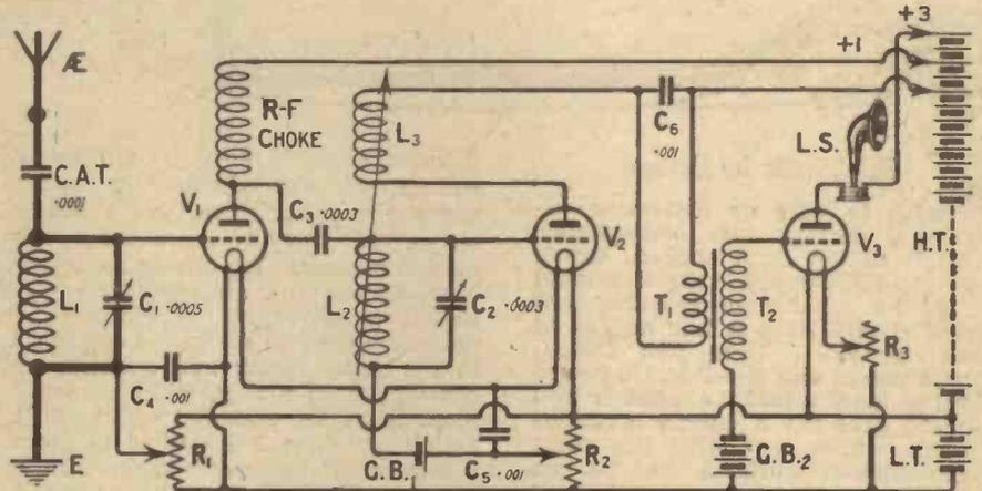
Reaction may be applied in a very simple manner to the circuit  $L_2 C_3$ , as illustrated.
