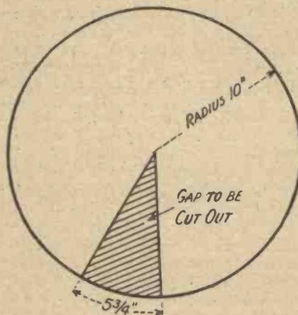
Fig. 5.—A cone diaphragm can be cut to these dimensions.
