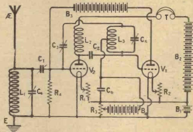
Fig. 4.—The final development was a neutralised version.
