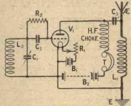
Fig. 7.—By tuning the grid circuit Fig. 6 becomes a true Reinartz.  $L_1$  and  $L_2$  are understood to be coupled together in each case.
