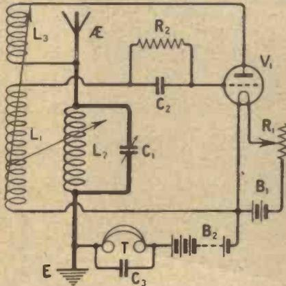
Fig. 5.—In this circuit the various couplings are shown, so that the relation of the two opposing reaction effects may be clear.
