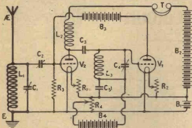
Fig. 3.—This is the circuit of Fig. 2 re-arranged in the manner usual in drawing reflex circuits.
