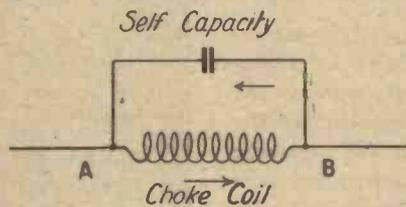
Fig. 2.—The inductance of the choke and its self-capacity may provide an actual reflector circuit.
