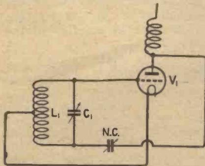
Fig. 1.—Centre-tapped coil circuits are prone to parasitic oscillation troubles.
