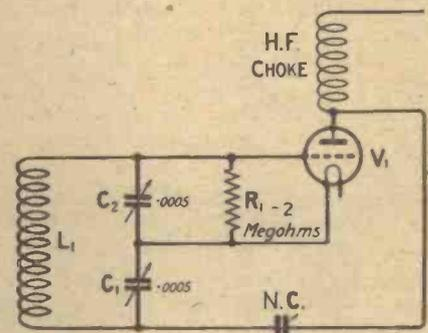
Fig. 3.—This circuit is free from parasitic oscillations, but the position of the grid-leak is not a desirable one.
