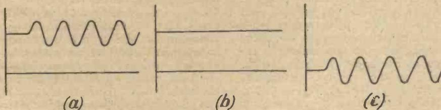
Fig. 1.—The anode current of a valve (a) can be regarded as being made up of a direct current component (b) and an alternating one (c).
