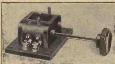
In the Penton coil-holder connection is made to the moving holder by means of metal strips.
