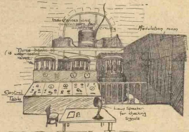
readjustments of the actual strength applied to the transmitter, but this is only a comparatively small adjustment, and the whole service is nothing more or less than a repeater station such as is employed on ordinary trunk telephone services.
