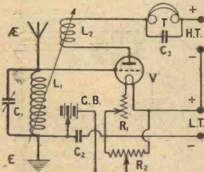
Fig. 2.—A grid-bias battery will usually be needed in addition to the potentiometer to apply a sufficiently negative bias to the grid of the valve.
