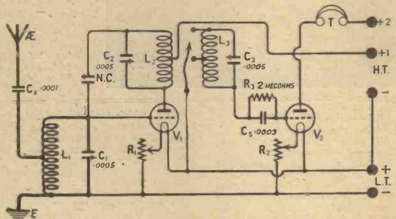
The circuit is repeated for reference purposes. Note that  $L_3$  is the movable coil.
