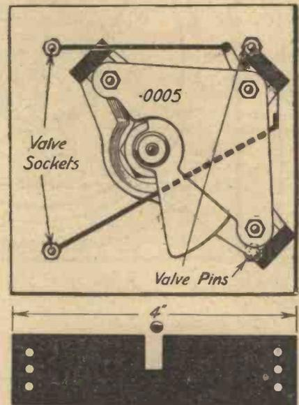
*Fig. 1(a).—The layout of the panel carrying the variable condenser will be apparent from this diagram. (b) Two pieces of ebonite of this shape will be required for each coil former,*
