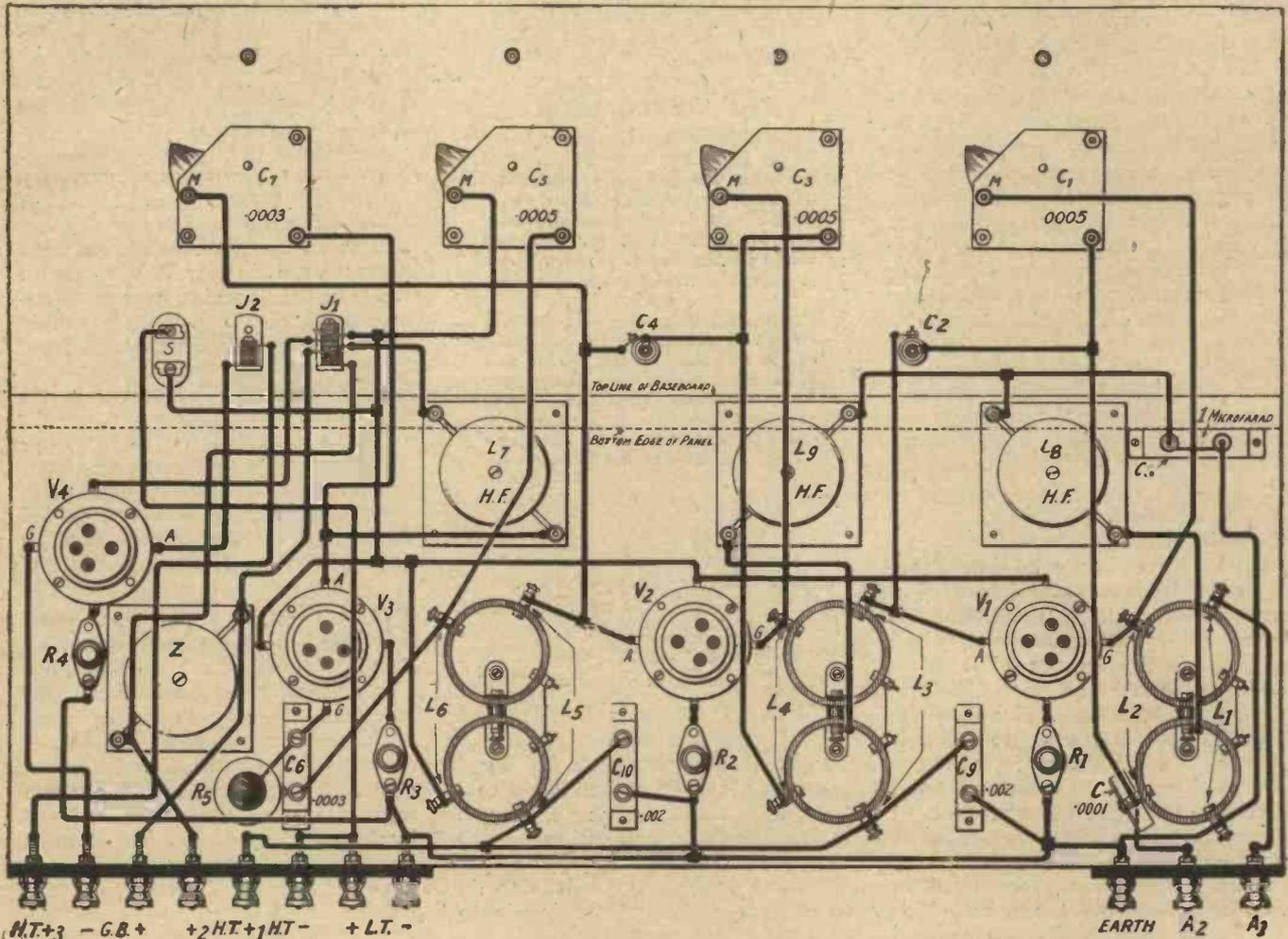
Fig. 3.—The condenser C8 should be shorted with a piece of wire when no grid bias is being used.
