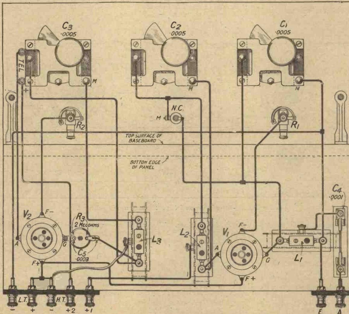
Fig. 2.—In wiring the set it is recommended that the leads to the coil  $L_3$  should be done with flex.
