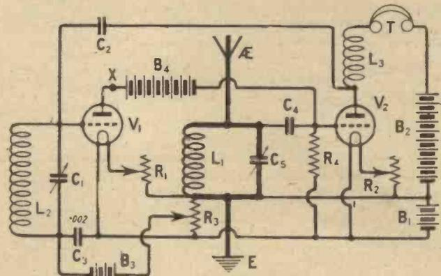
Fig. 2.—In this reflexed version "Parallel Feed" H.F. coupling is used.
