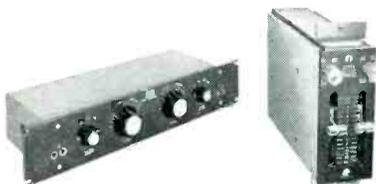
**ALTEC 9061A & 9063A PROGRAM EQUALIZERS** provide continuously variable equalization at selectable frequencies: up to 12-db boost at 40 or 100 cycles, and 3, 5, 10 or 15 kc; 16-db attenuation at 100 cycles and 10 kc. Passive circuitry. 9061A, for plug-in mounting, features straight-line controls. 3½"H x 1½"W x 5½"D. 9063A, for standard rack mounting, has rear-mounted input and output terminals normaled through front-panel jacks and rotary control switches. 3½"H x 19"W x 5¼"D.
