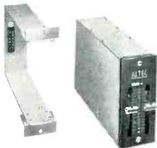
**ALTEC 9060A MICROPHONE EQUALIZER** provides up to 12-db equalization, and 16-db attenuation at 100 cycles and 10 kc. Straight-line controls are precisely calibrated in 2-db steps. Passive L/C/R bridged "T" network circuit. Compact plug-in design. 3½"H x 1½"W x 5½"D.
