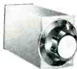
**ALTEC 9068A VARIABLE LOW-PASS FILTER AND 9069A VARIABLE HIGH-PASS FILTER** provide 18 db per octave attenuation with 10 positions of LF and HF cut-off. With toroidally wound inductances, units may be used in extremely low-level circuitry without noise or hum pick-up. Zero insertion loss. 9068A LOW-PASS FILTER is 3"H x 2¼"W x 5½"D. 9069A HIGH-PASS FILTER is same size.
