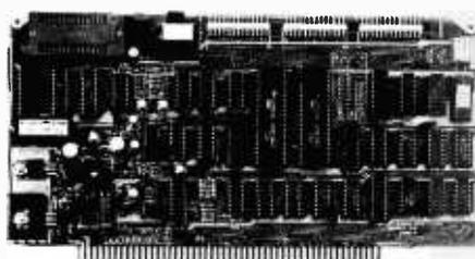
The BURNER I/O has a complete EPROM programmer, two serial ports, one parallel I/O port with handshaking and memory management.
