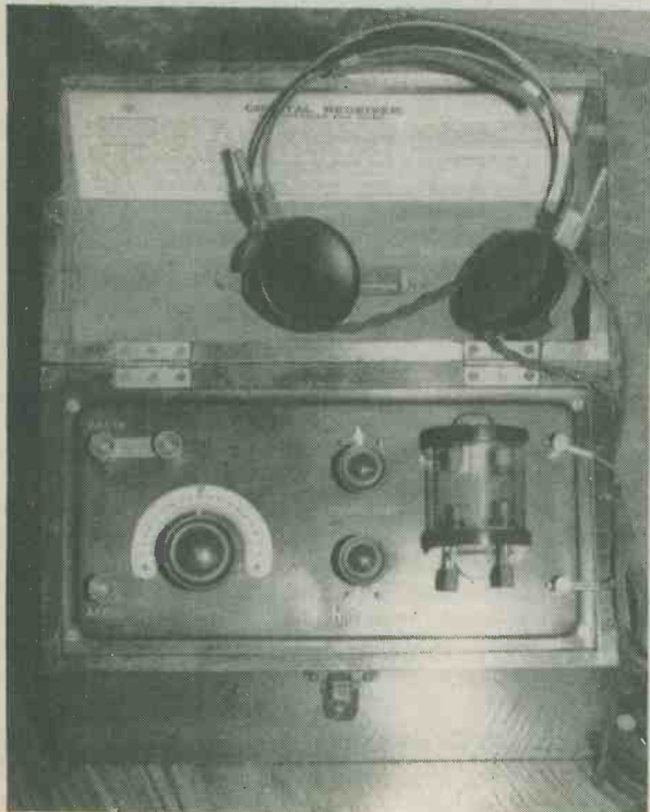
Overall view of the receiver, complete with headphones. The "Instructions For Using" are mounted inside the receiver case lid
